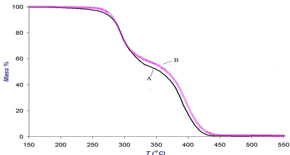
**Figure S3.** TGA curves of commercial PMMA (A) and the same polymer melt blended for 7 min in a Brabender mixer at 185 °C (B). (TGA, N<sub>2</sub>, 20 °C/min)
