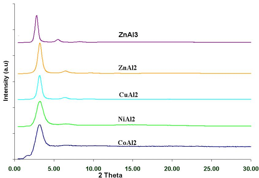
**Figure S1.** XRD traces of undecenoate containing LDHs of CoAl<sub>2</sub>, NiAl<sub>2</sub>, CuAl<sub>2</sub>, ZnAl<sub>2</sub> and ZnAl<sub>3</sub>.
