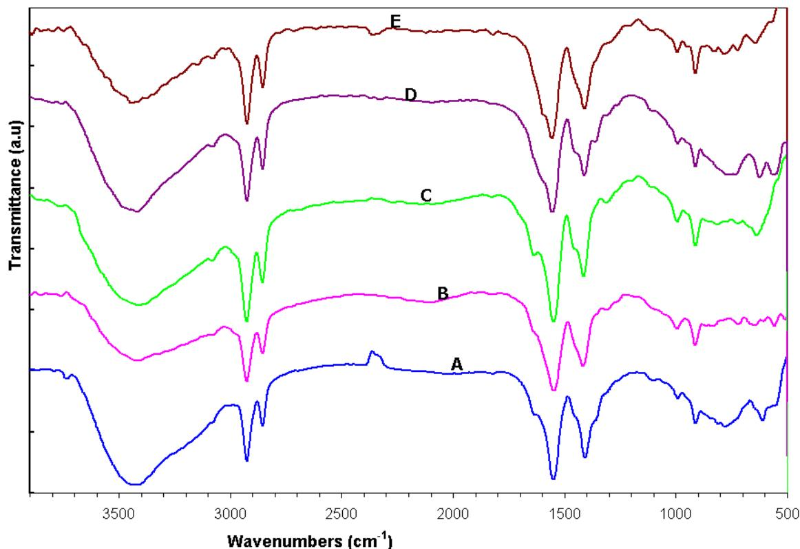
**Figure S2:** FT-IR of different undecenoate LDHs : (A) CoAl<sub>2</sub>; (B) CuAl<sub>2</sub>; (C) NiAl<sub>2</sub>; (D) ZnAl<sub>2</sub> and (E) ZnAl<sub>3</sub>.
