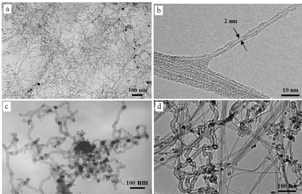
Figure S3. TEM images of the as-grown samples synthesized at 1000°C. (a,b) SD-SWCNTs without addition of thiophene (sample 1); (c) MWCNTs with addition of 1% thiophene (sample 2). (d) TEM images of the as-grown sample synthesized at 1100°C with addition of 1% thiophene (sample 4).
