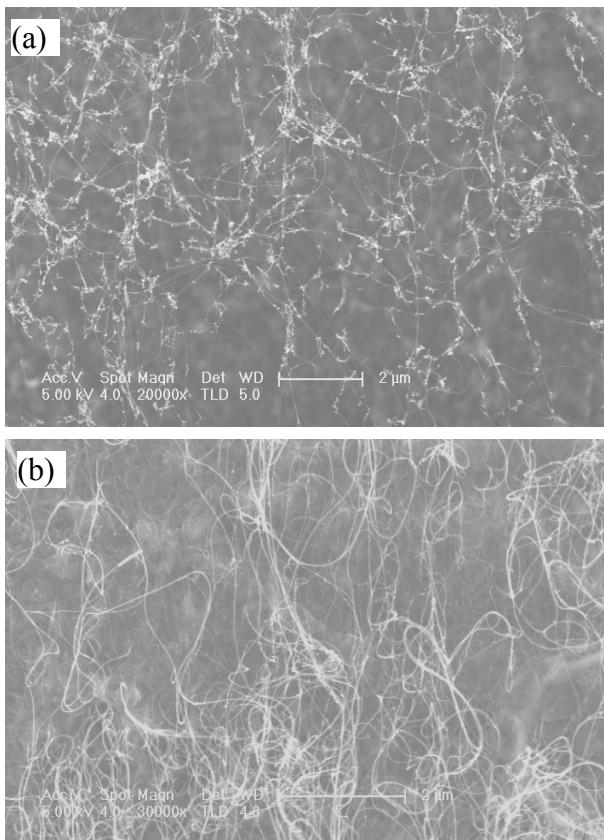
Figure S5. SEM images of the as-prepared (a) and purified SWCNTs (b).
