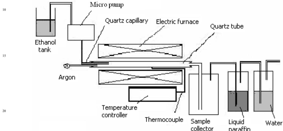
Figure S1. Experimental setup used for the present synthesis of carbon nanotubes. Note that when no thiophene was added, single wall carbon nanotubes could be collected only from the internal wall of
