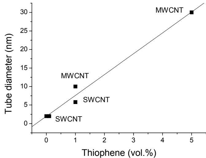
Figure S8. Dependence of tube diameter on thiophene addition.
