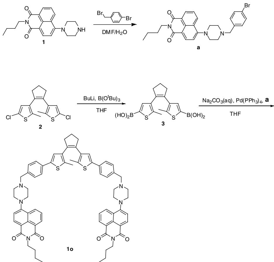
**Scheme S1:** Synthesis route of Nap-Pip-DTE **1o**.
