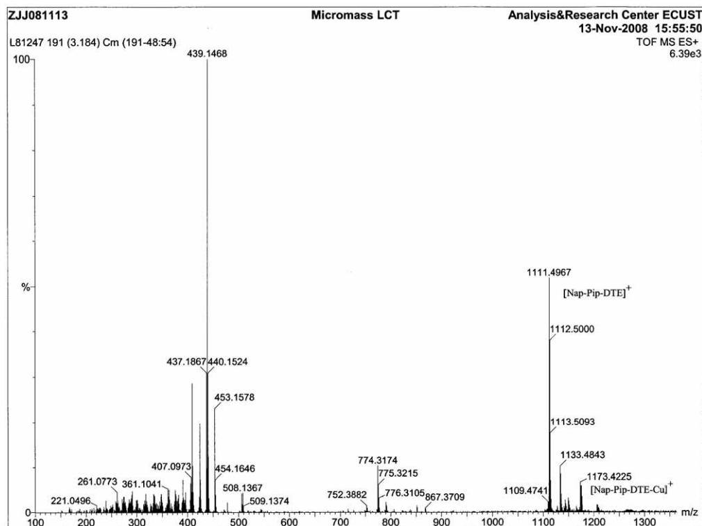
**Figure S3:** ESI-MS spectra of Nap-Pip-DTE **1o** (top) and Nap-Pip-DTE-Cu **1oCu** (bottom) in a mixture of H<sub>2</sub>O-CH<sub>3</sub>CN (1:9, v/v), and calculated isotopic distribution for the peaks at 1111.4974 and 1173.4255, respectively.
