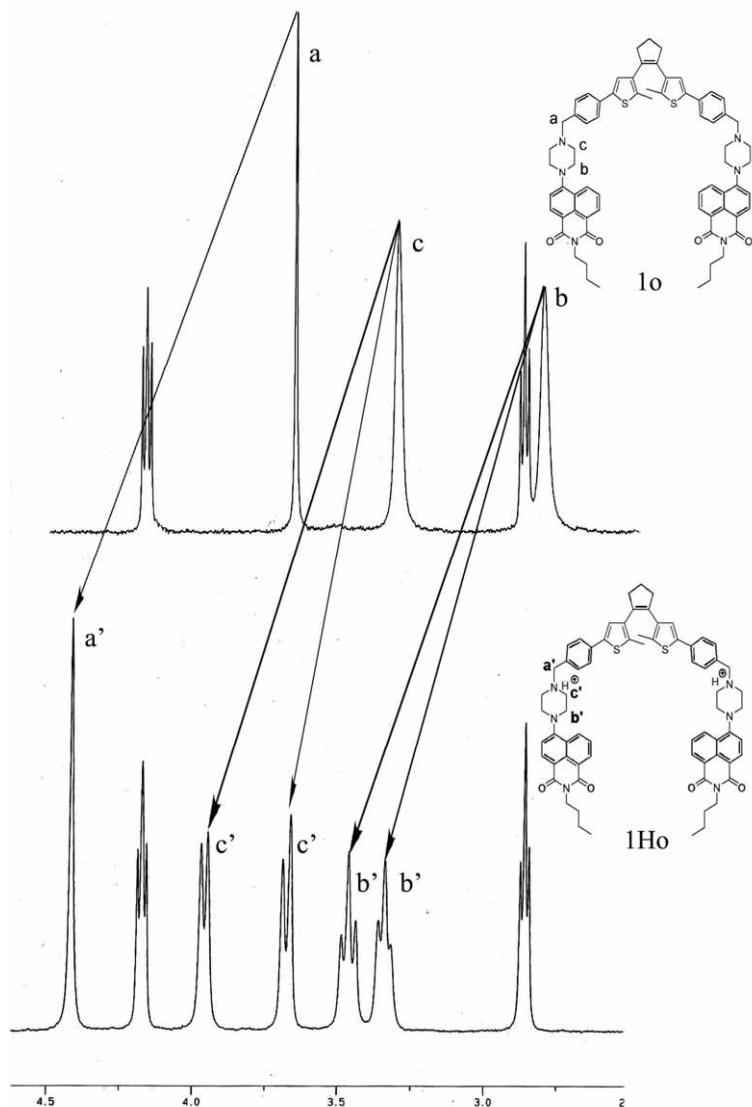
**Figure S4:** Parts of the <sup>1</sup>H NMR spectra of: Nap-Pip-DTE **1o** (top) and after protonation **1Ho** (bottom) in CDCl<sub>3</sub>.
