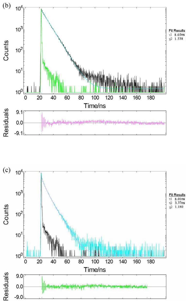
**Figure S8:** The fluorescence life-time of **1o**, **1Ho** and **1oCu** was measured in the mixture of  $\text{CH}_3\text{CN}: \text{H}_2\text{O}$  ( $\text{v/v} = 9:1$ ) at 510 nm emission monitor upon excited at 440 nm at room temperature. (a) The life-time of **1o** (blue,  $\tau_1 = 7.29$  ns,  $\tau_2 = 0.25$  ns). (b) The life-time of **1Ho** (black,  $\tau_1 = 8.05$  ns). (c) The life-time of **1oCu** (blue,  $\tau_1 = 8.01$  ns,  $\tau_2 = 3.37$  ns).
