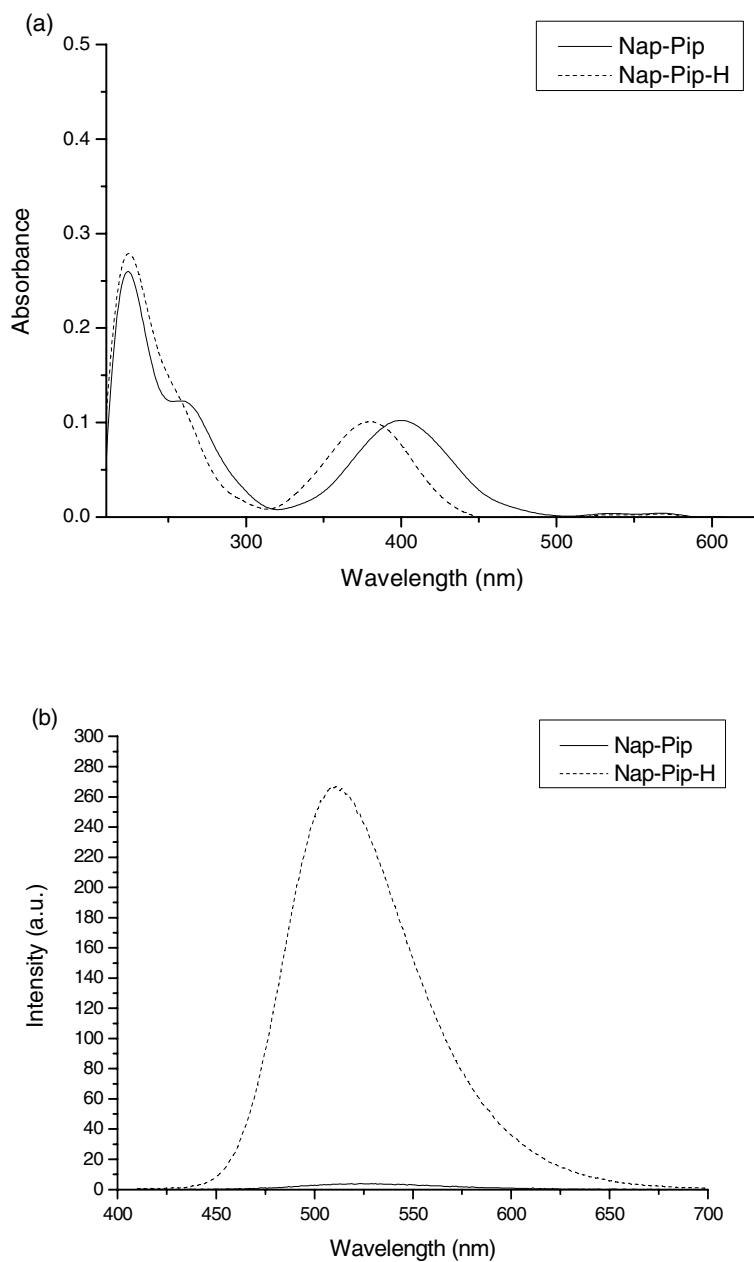
**Figure S5:** (a) Absorption spectra and (b) emission spectra of Nap-Pip ( $10^{-5}$  M, solid line) and Nap-Pip-H ( $10^{-5}$  M, dash line) in a mixture of  $\text{CH}_3\text{CN}: \text{H}_2\text{O} = 9:1$  (v/v). All emissions are excited upon 400 nm at 298K.
