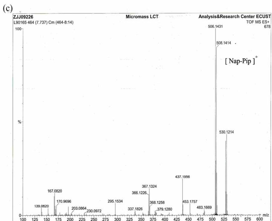
**Figure S1:** (400MHz) (a) <sup>1</sup>H-NMR spectra (b) <sup>13</sup>C-NMR spectra and (c) ESI-MS spectra of Nap-Pip (a) in CDCl<sub>3</sub>, and calculated isotopic distribution for the peaks at 506.1431.
