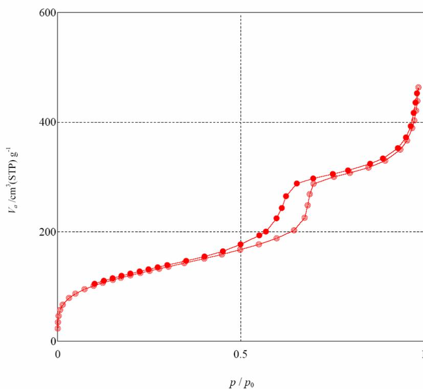
**Figure 7.** Nitrogen adsorption-desorption isotherm for SBA-15-Pr-SO<sub>3</sub>H
