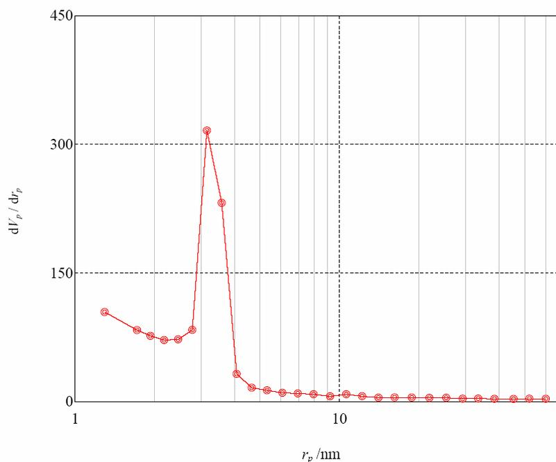
**Figure 8.** BJH average pore diameter diagram for SBA-15-Pr-SO<sub>3</sub>H
