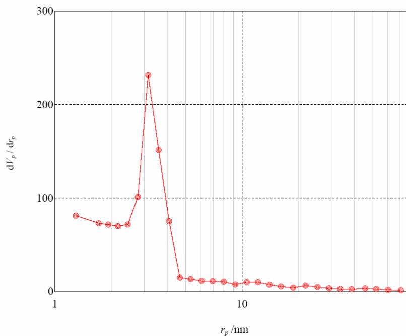
**Figure 3.** BJH average pore diameter diagram for SBA-15-Pr-SH
