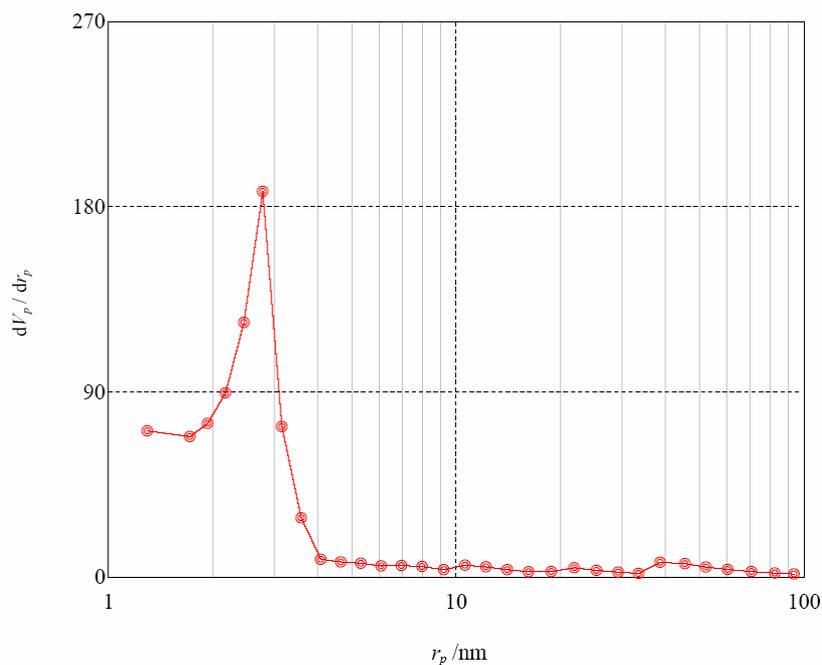
**Figure 11.** BJH average pore diameter diagram for SBA-15-Ph-Pr-SO<sub>3</sub>H
