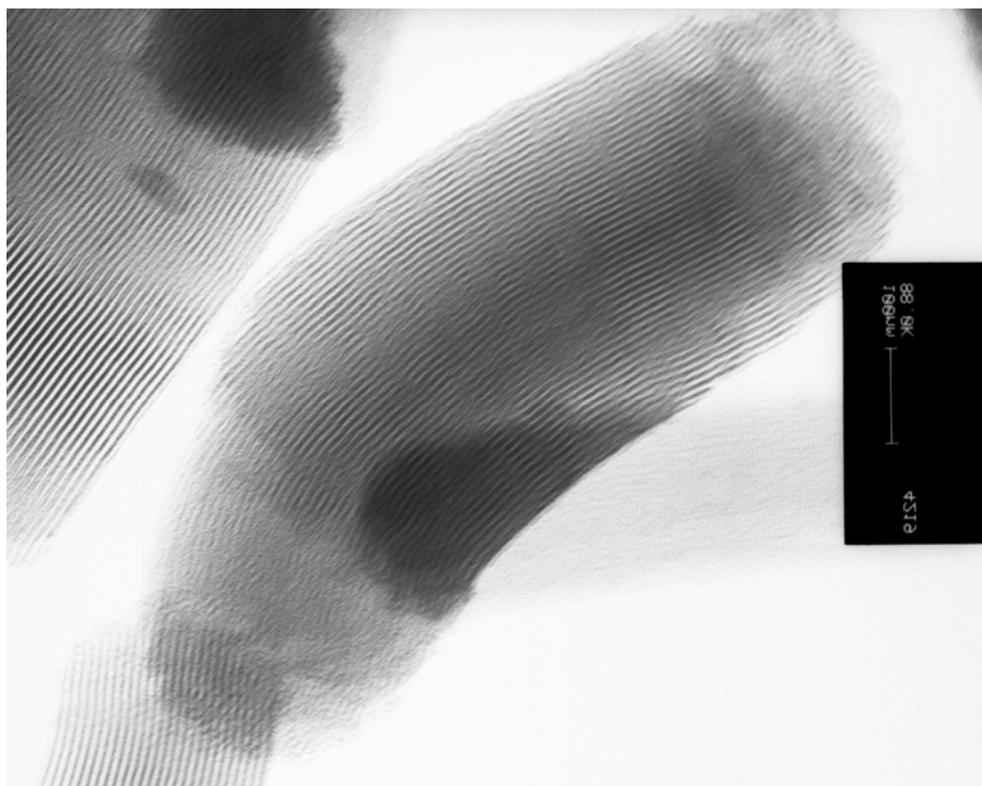
**Figure 12:** TEM image of SB/A-15-Ph-Pr-SO<sub>3</sub>H
