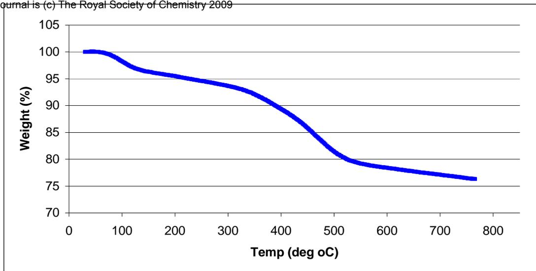
**Figure 9.** TGA diagram of SBA-15-Ph-Pr-SO<sub>3</sub>H
