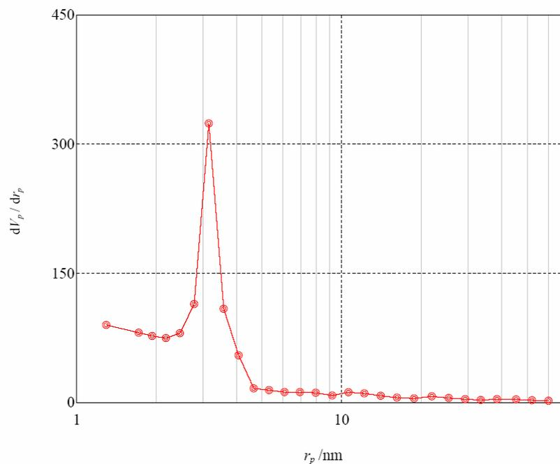
**Figure 6.** BJH average pore diameter diagram for SBA-15-Ph-Pr-SH
