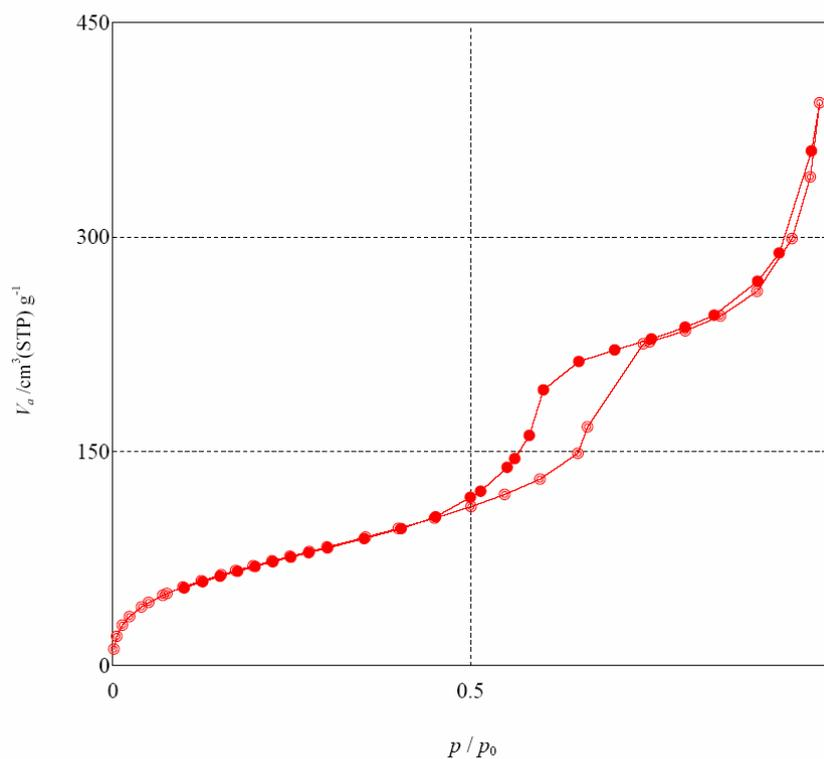
**Figure 2.** Nitrogen adsorption-desorption isotherm for SBA-15-Pr-SH
