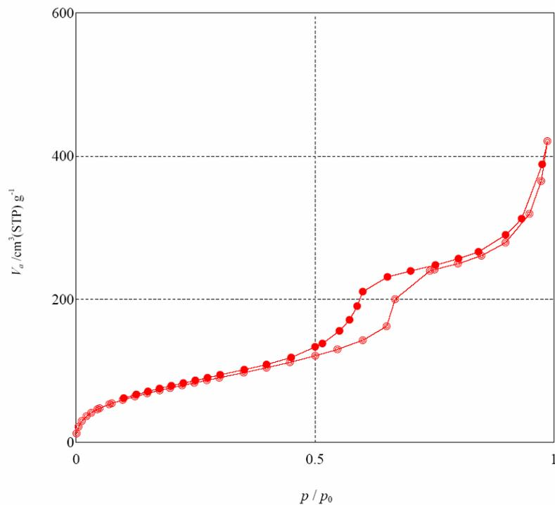
**Figure 5.** Nitrogen adsorption-desorption isotherm for SBA-15-Ph-Pr-SH
