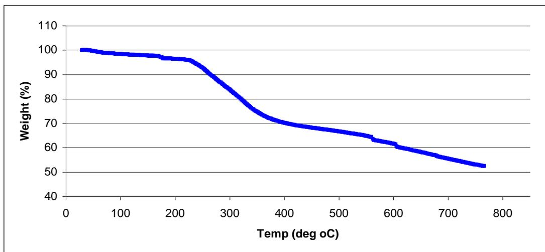
**Figure 1.** TGA diagram for SBA-15-Pr-SH
