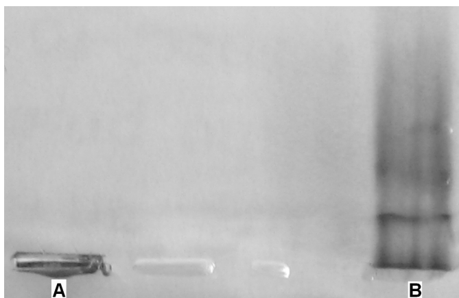
Fig. S1 Gel electrophoresis (0.5% agarose in 0.5x TBE) of before and after ligand exchange: lane A, one-dimensional gold nanoparticles-CTAB; lane B, one-dimensional gold nanoparticles-mono-6-thio- \beta -cyclodextrin
