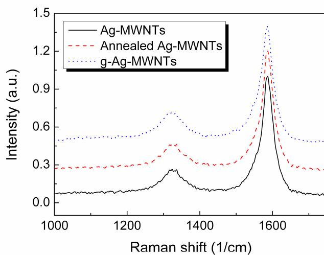
Figure S4. Raman spectra of Ag-MWNTs, annealed Ag-MWNTs and g-Ag-MWNTs. The excitation wavelength was 633 nm (Kaiser Optical, Raman microscope), and the spectra were normalized by the g-peak of nanotubes.
