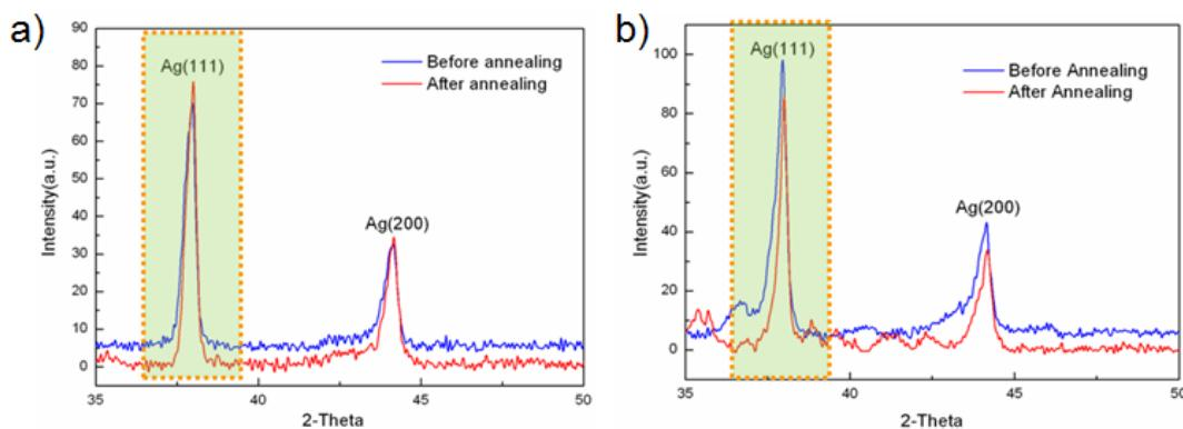
Figure S3. XRD patterns before and after the annealing process at 185 °C for 1 hr. (a) Ag-MWNTs (b) g-Ag-MWNTs.
