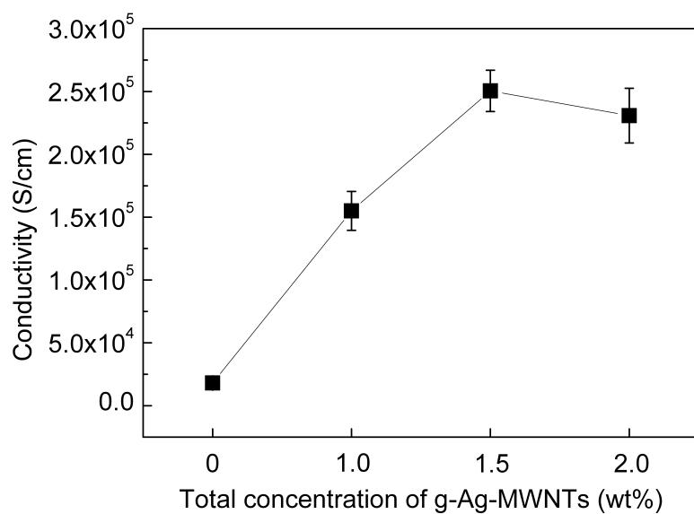
Figure S5. The conductivity of the composite as a function of the total concentration of g-Ag-MWNTs.
