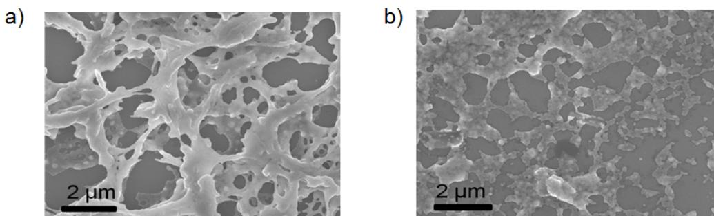
Figure S2. SEM images of coalesced nano-Ag particles annealed at 185 °C for 1 hr. (a) Before glutaric-acid functionalization (b) After functionalization.
