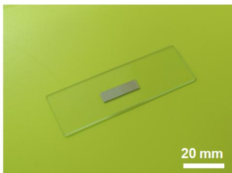
Figure S1. The specimen for the conductivity measurements were screen-printed using the silver/epoxy composite with g-Ag-MWNTs.
