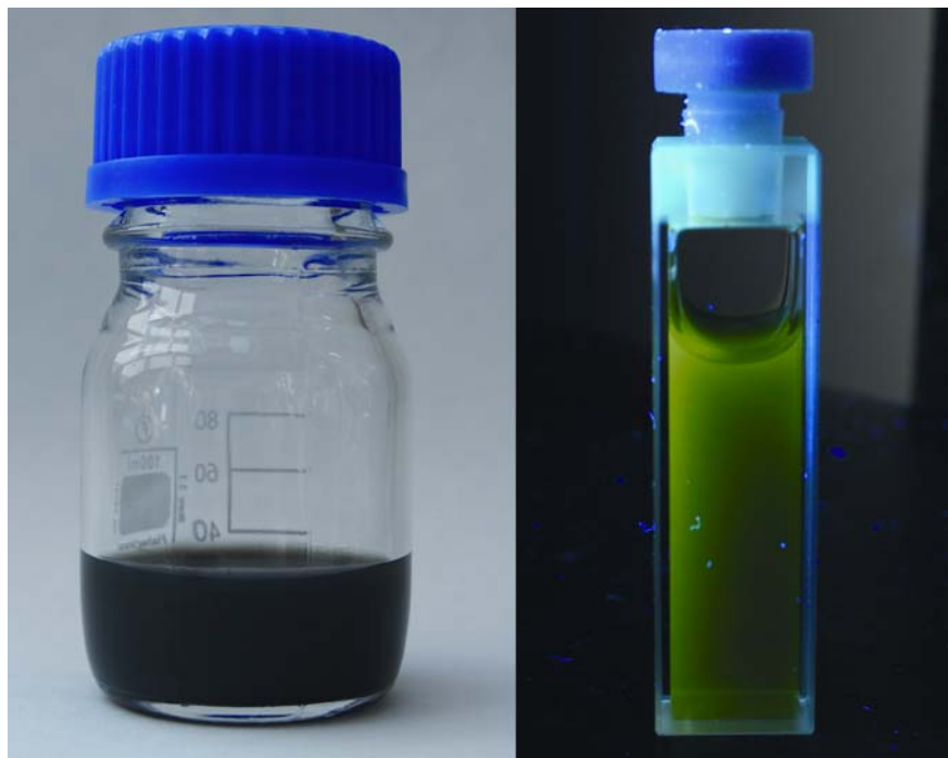
Fig. S1 Photo of LSMO@siF@si-w water dispersion under daylight (left) and under UV irradiation (right).
