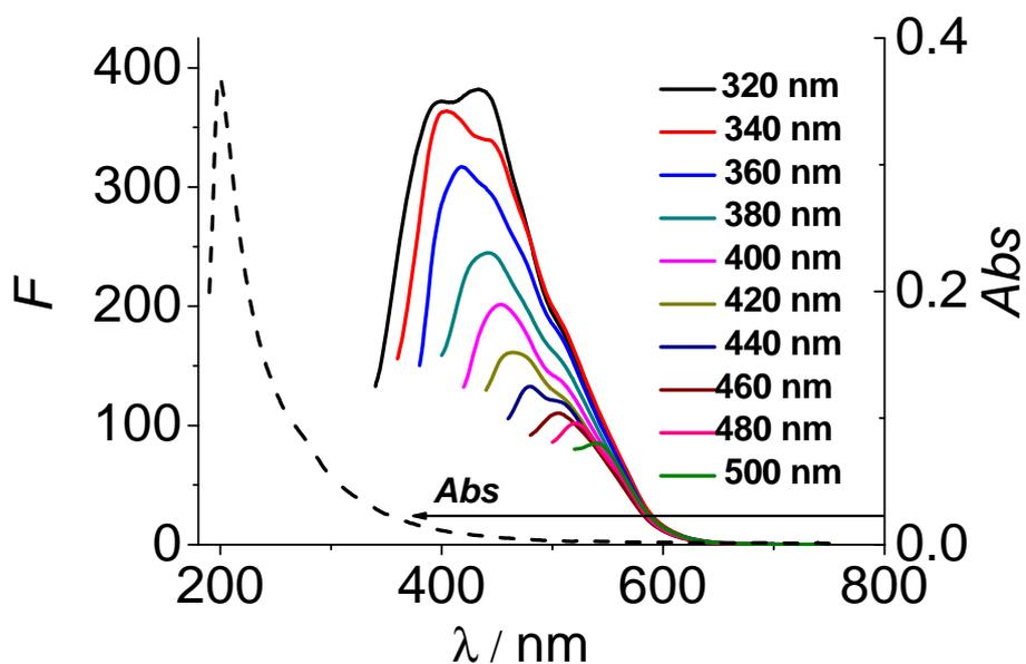
**Figure S9.** UV-Visible absorption spectrum and photoluminescence emission spectra (with progressively longer excitation wavelengths from 320 nm to 500 nm in 20 nm increment) of carbon dots (microwave pyrolysis condition: 70% glycerol, 5 mM  $\text{H}_2\text{SO}_4$ , 8 min). By selecting quinine sulfate as the standard and 360 nm as the excitation wavelength, the photoluminescence quantum yield was measured and calculated to be 7.7%.
