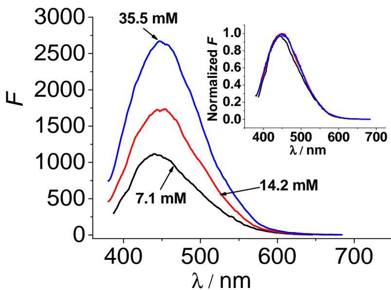
**Figure S7.** Photoluminescence emission spectra ( $\lambda_{\text{ex}} = 360 \text{ nm}$ ) of carbon dots normalized to the absorbance at 360 nm. Microwave synthesis conditions: 70% glycerol, 7.1, 14.2 or 35.5 mM phosphate, 12 min. Inset: normalized photoluminescence emission spectra.
