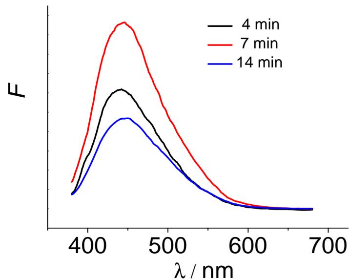
**Figure S5** Photoluminescence emission spectra ( $\lambda_{\text{ex}} = 360 \text{ nm}$ ) of carbon dots normalized to the absorbance at 360 nm. Microwave synthesis conditions: 70% glycerol, 7.1 mM phosphate, 4, 7 or 14 min.
