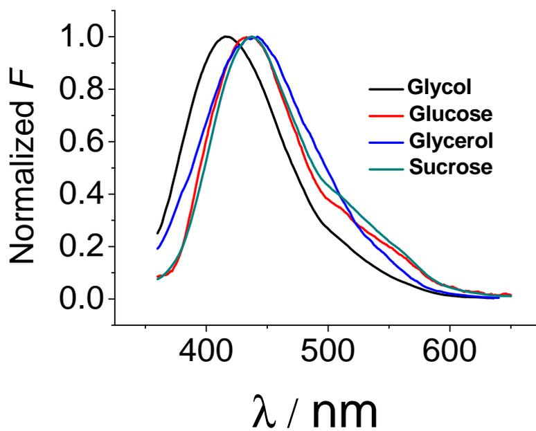
**Figure S11.** Normalized photoluminescence emission spectra ( $E_x = 340$  nm) of carbon dots synthesized from different carbohydrate starting materials.
