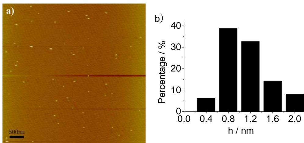
**Figure S4** AFM characterization of carbon dots synthesized by 70% glycerol in the presence of 7.1 mM phosphate with 7 min. (a) Representative AFM image; (b) height analysis.
