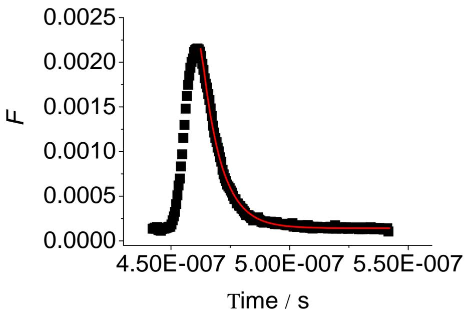
**Figure S1.** Photoluminescence decay curve of carbon dots in water. A single exponential fit gives a lifetime of  $8.00 \pm 0.07$  ns. Luminescence lifetime was measured with a Lecroy Wave Runner 6100 digital oscilloscope (1 GHz) using a 355 nm laser (Continuum Sunlite OPO with pulse width = 4 ns) as an excitation source.
