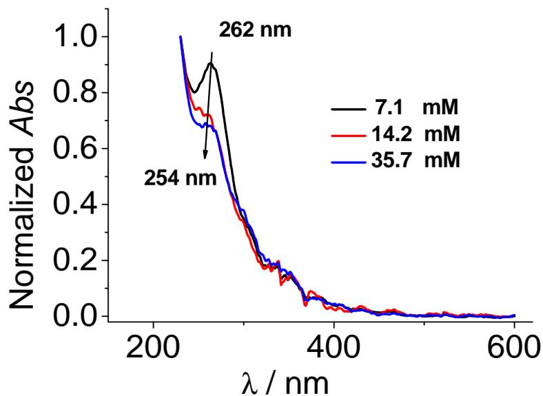
**Figure S6.** Normalized absorption spectra of carbon dots synthesized by 70% glycerol in the presence of different amounts of phosphate salt with 12 min microwave treatment.
