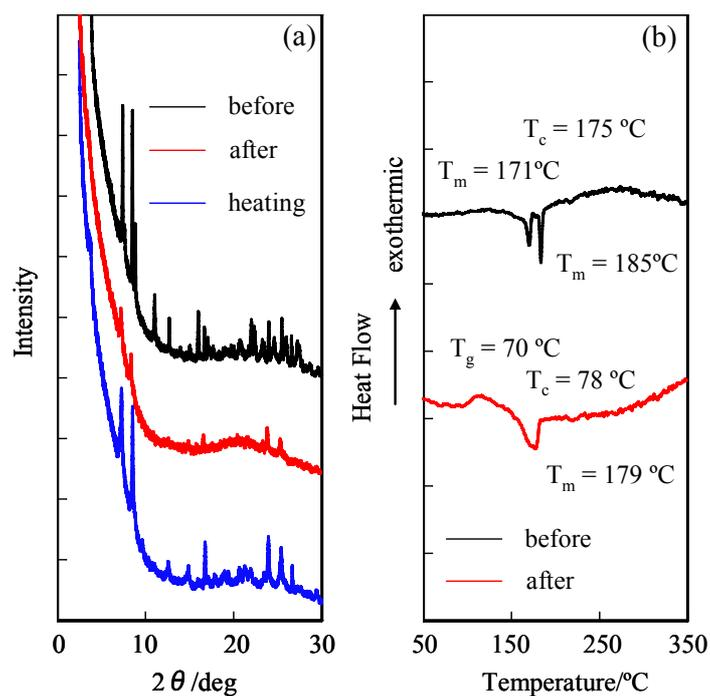
**Fig. S23** (a) XRD patterns and (b) DSC curves (scan rate:  $10^\circ\text{C min}^{-1}$ ) of **i4a** before and after grinding, and after heating the ground solid.
