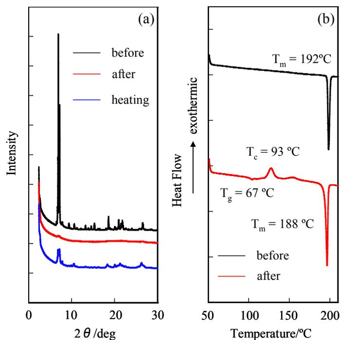
**Fig. S16** (a) XRD patterns and (b) DSC curves (scan rate:  $10^\circ\text{C min}^{-1}$ ) of **1d** before and after grinding, and after heating the ground solid.
