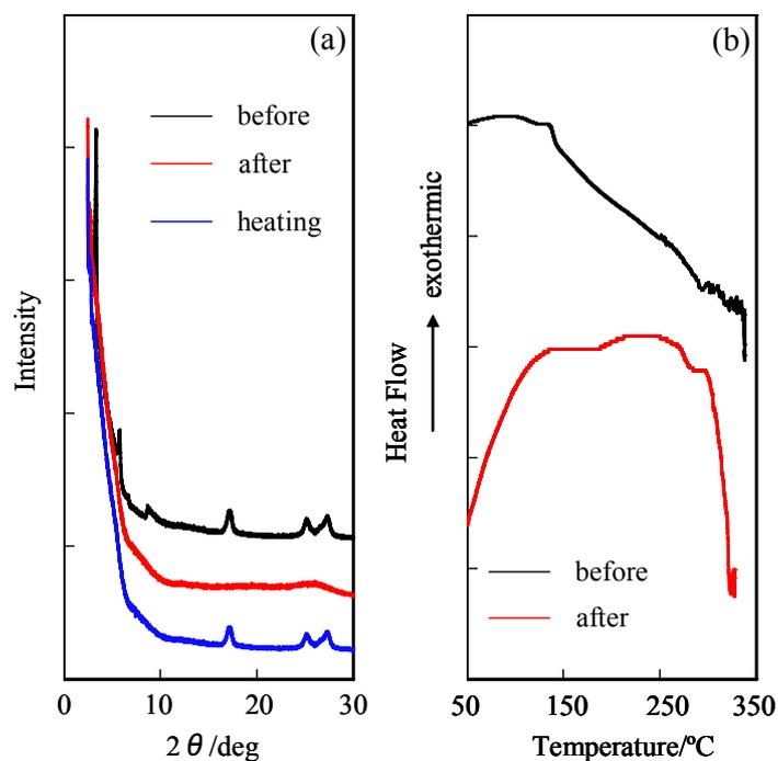
**Fig. S18** (a) XRD patterns and (b) DSC curves (scan rate:  $10^{\circ}\text{C min}^{-1}$ ) of **3a** before and after grinding, and after heating the ground solid.
