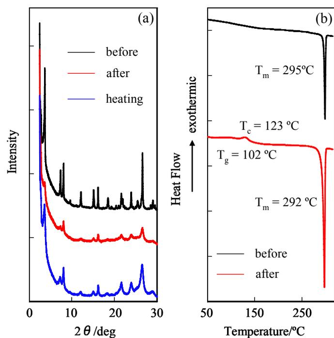
**Fig. S13** (a) XRD patterns and (b) DSC curves (scan rate:  $10^\circ\text{C min}^{-1}$ ) of **1a** before and after grinding, and after heating the ground solid.
