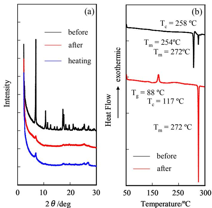
**Fig. S15** (a) XRD patterns and (b) DSC curves (scan rate:  $10^\circ\text{C min}^{-1}$ ) of **1c** before and after grinding, and after heating the ground solid.
