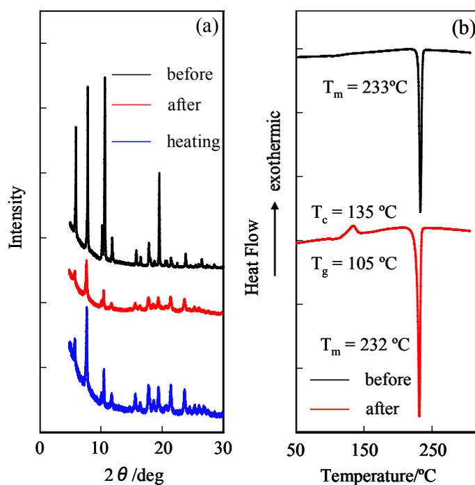
**Fig. S20** (a) XRD patterns and (b) DSC curves (scan rate:  $10^{\circ}\text{C min}^{-1}$ ) of **5a** before and after grinding, and after heating the ground solid.
