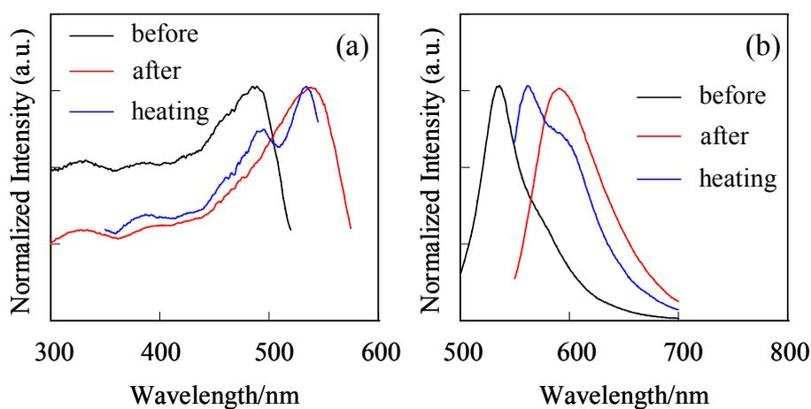
**Fig. S2** (a) Excitation and (b) fluorescence spectra of **1b** before and after grinding, and after heating the ground solid at 150 °C.
