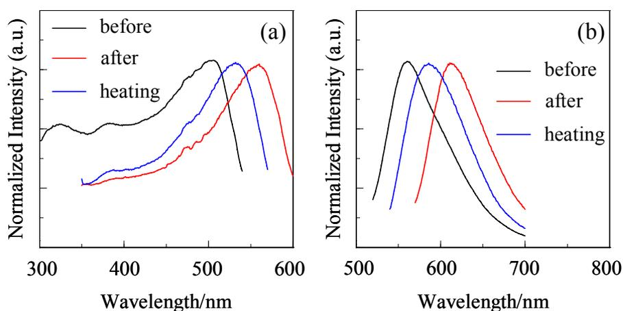
**Fig. S1** (a) Excitation and (b) fluorescence spectra of **1a** before and after grinding, and after heating the ground solid at 150 °C.
