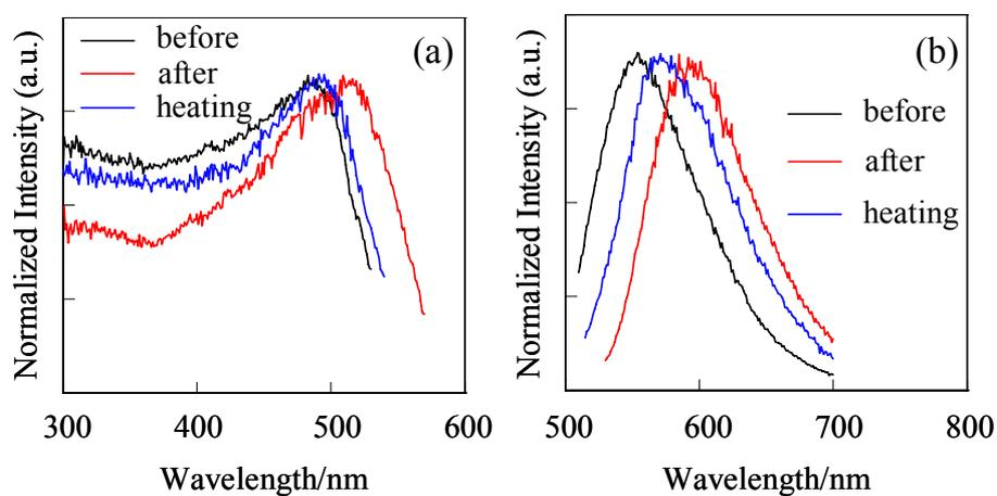
**Fig. S10** (a) Excitation and (b) fluorescence spectra of **11b** before and after grinding, and after heating the ground solid at 200 °C.
