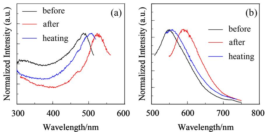
**Fig. S5** (a) Excitation and (b) fluorescence spectra of **2a** before and after grinding, and after heating the ground solid at 180 °C.
