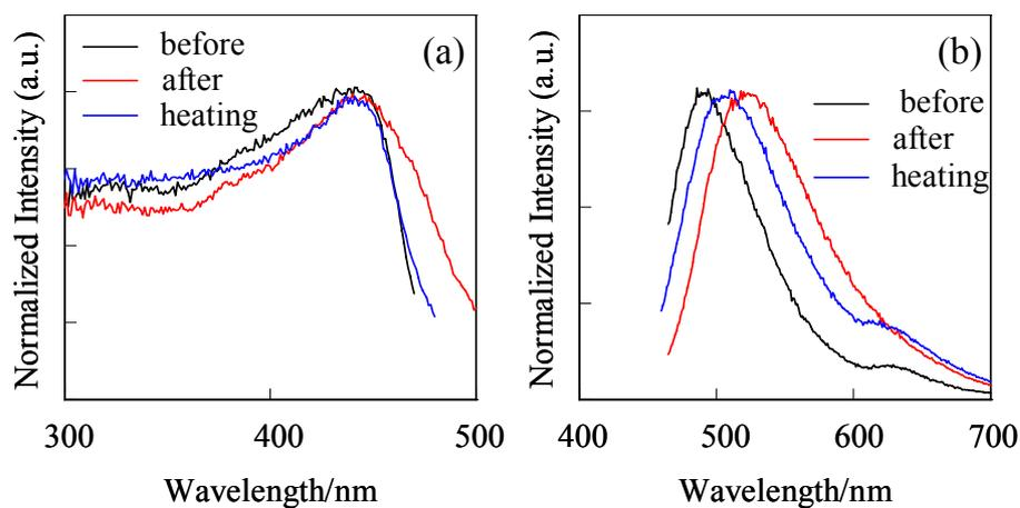
**Fig. S11** (a) Excitation and (b) fluorescence spectra of **i4a** before and after grinding, and after heating the ground solid at 150 °C.
