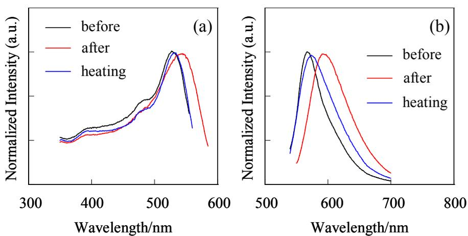
**Fig. S4** (a) Excitation and (b) fluorescence spectra of **1d** before and after grinding, and after heating the ground solid at 150 °C.
