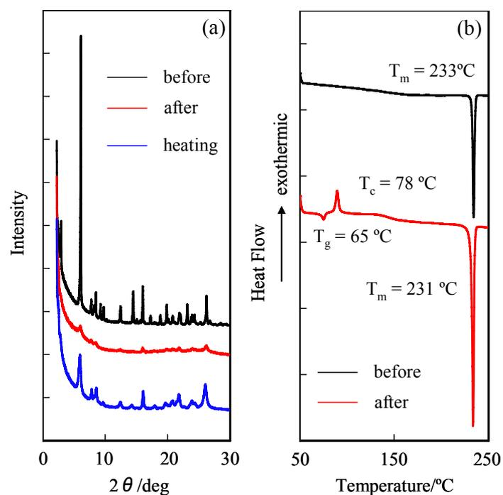
**Fig. S14** (a) XRD patterns and (b) DSC curves (scan rate:  $10^\circ\text{C min}^{-1}$ ) of **1b** before and after grinding, and after heating the ground solid.
