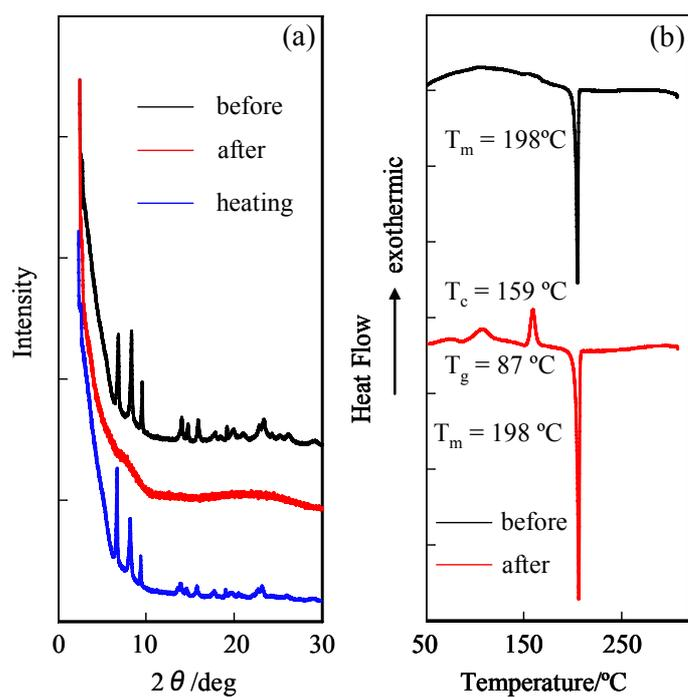
**Fig. S19** (a) XRD patterns and (b) DSC curves (scan rate:  $10^{\circ}\text{C min}^{-1}$ ) of **4a** before and after grinding, and after heating the ground solid.
