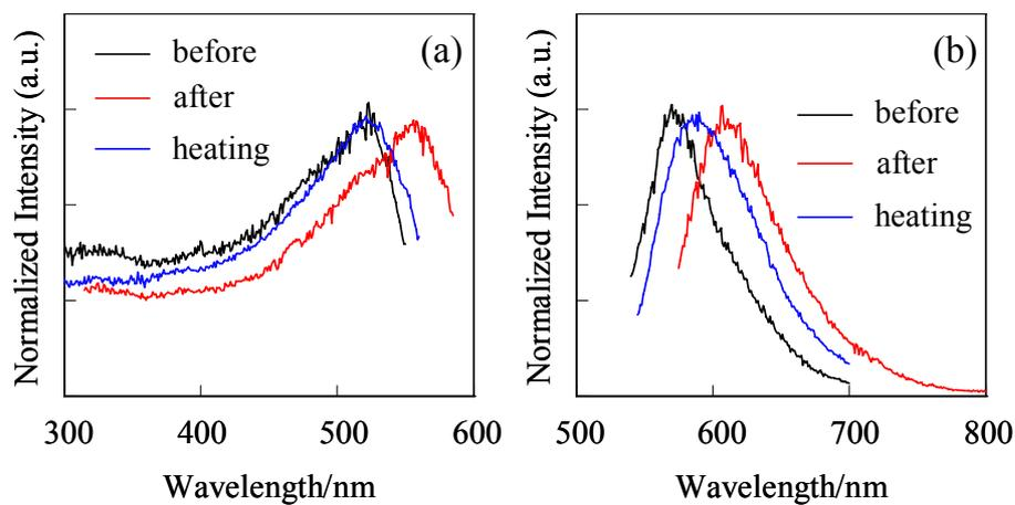
**Fig. S9** (a) Excitation and (b) fluorescence spectra of **3b** before and after grinding, and after heating the ground solid at 230 °C.
