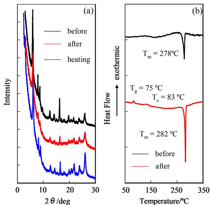
**Fig. S22** (a) XRD patterns and (b) DSC curves (scan rate:  $10^\circ\text{C min}^{-1}$ ) of **11b** before and after grinding, and after heating the ground solid.
