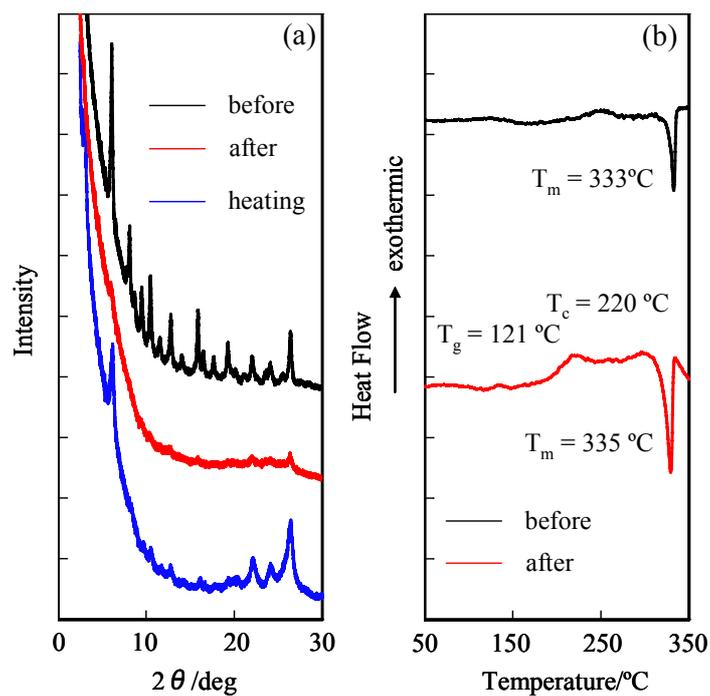
**Fig. S21** (a) XRD patterns and (b) DSC curves (scan rate:  $10^\circ\text{C min}^{-1}$ ) of **3b** before and after grinding, and after heating the ground solid.
