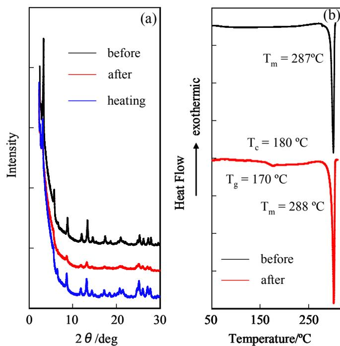
**Fig. S17** (a) XRD patterns and (b) DSC curves (scan rate:  $10^{\circ}\text{C min}^{-1}$ ) of **2a** before and after grinding, and after heating the ground solid.
