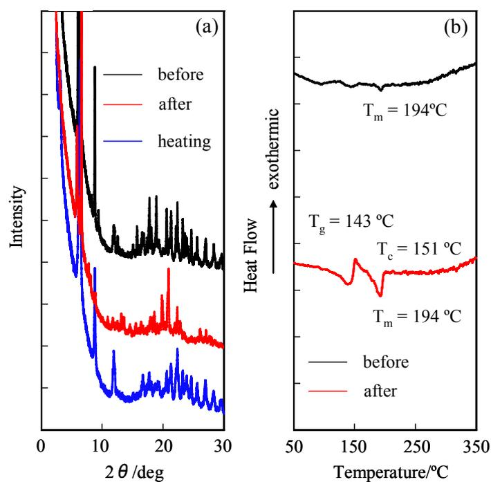
**Fig. S24** (a) XRD patterns and (b) DSC curves (scan rate:  $10^\circ\text{C min}^{-1}$ ) of **i5a** before and after grinding, and after heating the ground solid.
