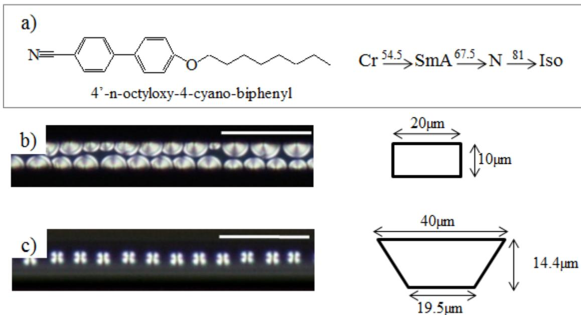
Fig. S1. a) The molecular structure and phase transition temperature of 4'-n-octyloxy-4-cyano-biphenyl (8OCB). b) POM images of 8OCB in a PEI coated rectangular microchannel with width = 20  $\mu\text{m}$  and depth = 10  $\mu\text{m}$ . c) POM image of 8OCB in a PEI coated trapezoidal microchannels with top-width = 40  $\mu\text{m}$ , bottom-width = 19.5  $\mu\text{m}$  and depth = 14.4  $\mu\text{m}$  (Scale: 50  $\mu\text{m}$ ).
