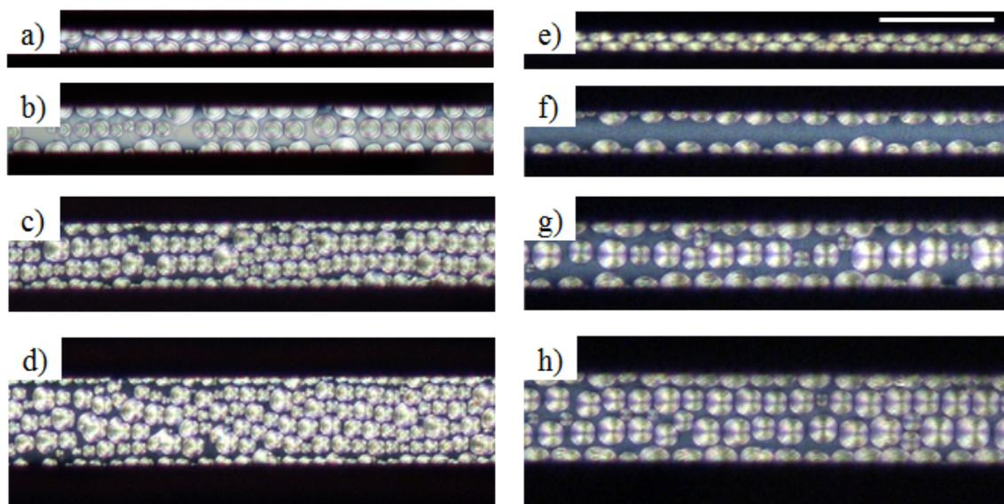
Fig. S2. POM images of 8CB in rectangular shaped channels of different widths and depths. a-d) width = 10 - 40 $\mu\text{m}$  (from top to bottom) and fixed depth = 5 $\mu\text{m}$ . e-h) width = 10 - 40 $\mu\text{m}$  (from top to bottom) and fixed depth = 10 $\mu\text{m}$  (Scale: 50  $\mu\text{m}$ ).
