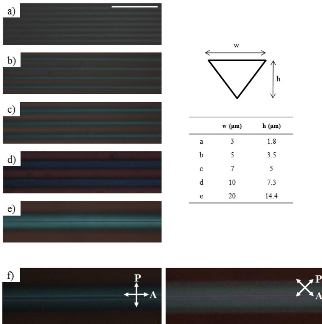
Fig. S3. a-e) POM images of **8CB** in V-shaped channels of different  $w = 3 - 20\mu\text{m}$  and  $h = 1.8-14.4\mu\text{m}$  (Scale:  $50\mu\text{m}$ ). f) POM images taken by rotating the samples at  $0^\circ$  and  $45^\circ$ .
