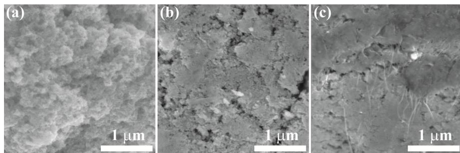
**Figure S1.** SEM images of (a) MnO<sub>2</sub> nanoparticles, (b) MnO<sub>2</sub> nanoparticles with carbon black + PTFE binder, showing granular structures, and (c) MnO<sub>2</sub> nanoparticles with the GO/SWCNTs/ PEDOT:PSS (G-T-P) glue forming continuous phase with interpenetrating SWCNTs.
