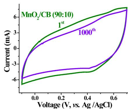
**Figure S3.** Cycling performance of MnO<sub>2</sub>/CB (90:10) without PTFE binder showing only 75% of the initial capacitance was retained after 1000 cycles.
