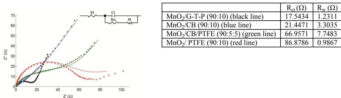
**Figure S2.** Fitting curves and equivalent circuit of the Nyquist plots in Figure 3b. R<sub>1</sub> is ohmic resistance; C<sub>1</sub> is the double layer capacitance; R<sub>ct</sub> is the charge transfer resistance; and W is the finite length Warburg contribution. The resultant values of R<sub>ct</sub> and R<sub>w</sub> from the fitting are shown in the right table.
