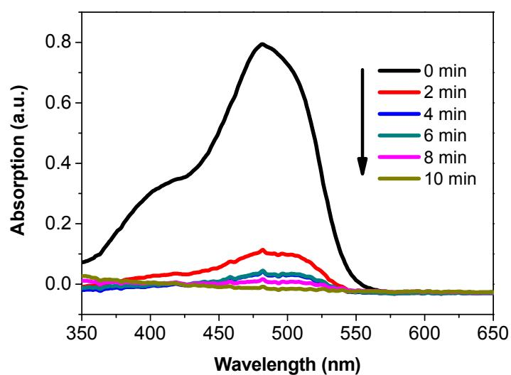
**Figure S4.** Absorption spectra of AO 7 solution at different time after irradiating with UV light and using  $\text{TiO}_2$  P25 as the reference photocatalyst
