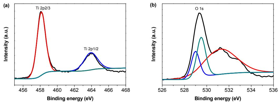
**Figure S5.** High resolution XPS spectrum of a) Ti 2p and b) O 1s of the TiO<sub>2</sub> nanorod spheres with Cu deposited.
