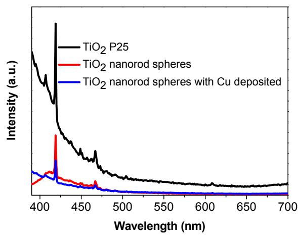
**Figure S3.** Photoluminescence spectrum of the TiO<sub>2</sub> nanorod spheres with Cu deposited, TiO<sub>2</sub> nanorod spheres and TiO<sub>2</sub> P25. From the PL spectrum of TiO<sub>2</sub> nanorod spheres and the TiO<sub>2</sub> nanorod spheres with Cu deposited, it is obvious that the electrons transfer between TiO<sub>2</sub> and Cu was enhanced by the deposition of Cu on the surface of TiO<sub>2</sub> nanorods. This is beneficial for the photocatalytic H<sub>2</sub> generation.
