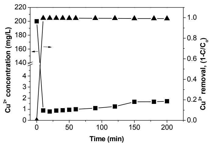
**Figure S6.** The Cu<sup>2+</sup> concentration against the reaction time in the simultaneous Cu<sup>2+</sup> removal and H<sub>2</sub> generation process under the irradiation of UV light and the corresponding removal rate of Cu<sup>2+</sup> from the solution
