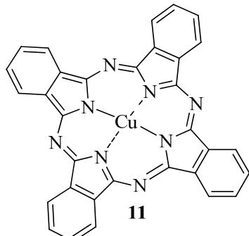
The SAW device was loaded with phthalonitrile (10 mg, 78 µmol), 1,8-diazabicyclo[5.4.0]undec-7-ene (35 µl, 234 µmol) and CuCl<sub>2</sub> (2.7 mg, 20.1 µmol) in diethylene glycol (40 µl) as the solvent. The reaction droplet was allowed to react on SAW for 15 min with the device and droplet temperature reaching 80 °C to afford, after collection by filtration and washing with ethanol, copper phthalocyanine **11** (5.8 mg) in an overall yield of 52%.
