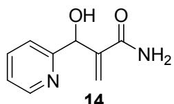
2-Pyridinecarboxaldehyde (**13**, 9.5 µl, 99.9 µmol), acrylamide (7.1 mg, 99.9 µmol) and quinuclidine (11.1 mg, 99.8 µmol) were mixed together in 10 µl of methanol and loaded onto the SAW device. The reaction droplet was allowed to react on SAW for 15 min with the device and droplet temperature reaching 70 °C to afford 2-(hydroxy(pyridin-2-yl)methyl)acrylamide as a colourless oil **14** (14.5mg) in an isolated yield (silica gel pipette column, eluting with ethyl acetate) of 86%.
