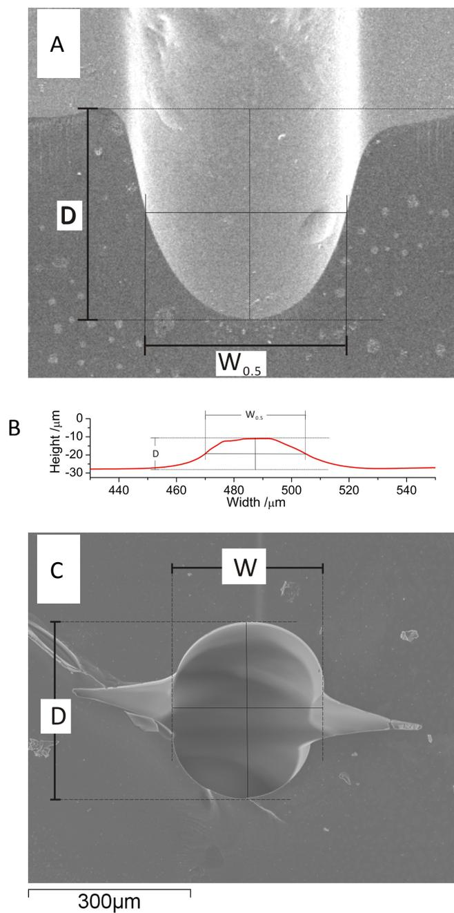
**Figure S1.** The depth (D) and width (W) of the three structures to calculate the aspect ratio was shown.
