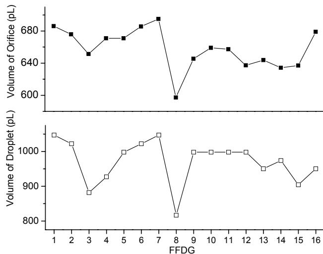
**Fig. S1** Correlation between the volumes of orifices in sixteen flow-focusing droplet generators (■) connected in a manifold manner in a module and the volumes of droplets (□) generated in these droplet generators. The flow rates of water and mineral oil are 3.2 and 0.53 mL/hr per droplet generator, respectively.
