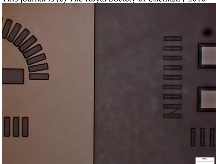
**Fig. S5.** Microphotograph of a portion of an etched die with both biased (left side) and physically isolated (right side) mask features. The metal mask appears bright in this epi-illumination image. The die was etched with a -2.0 V potential applied to the metal mask. Features on the die that were electrically isolated by design show enhanced lateral etch and extended tapers, while the electrically connected, biased portion of the die exhibits steeper sidewalls.
