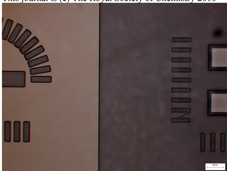
**Fig. S5.** Microphotograph of a portion of an etched die with both biased (left side) and physically isolated (right side) mask features. The metal mask appears bright in this epi-illumination image. The die was etched with a  $-2.0$  V potential applied to the metal mask. Features on the die that were electrically isolated by design show enhanced lateral etch and extended tapers, while the electrically connected, biased portion of the die exhibits steeper sidewalls.
