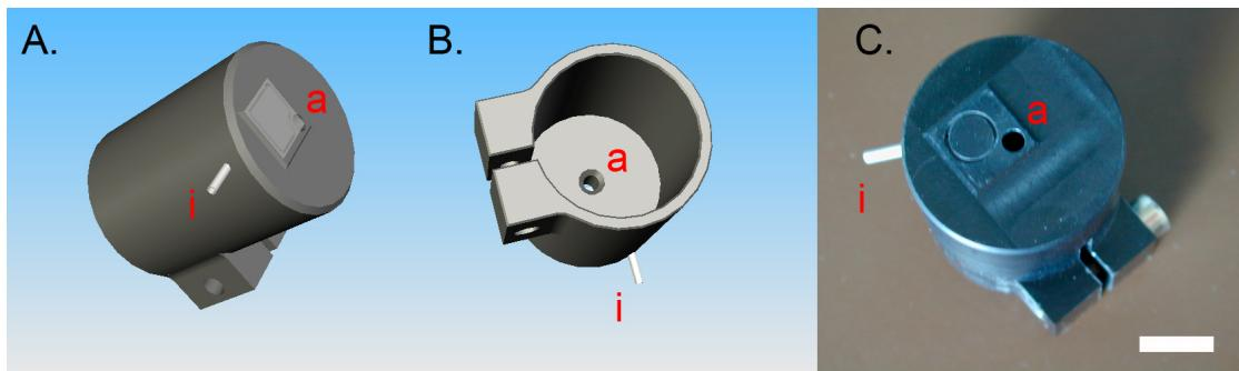
**Supplementary Figure 1** Adaptor Design. **(A and B)** 3D CAD image viewed from two angles. The inlet used to apply the vacuum is shown (i). **(C)** Photograph of adaptor from below. The 10 x 10 mm square area is used to hold the stamp with a vacuum using the ring channel. The smaller aperture within this square area is for observation through the stamp during printing. Scale bar indicates 1 cm.
