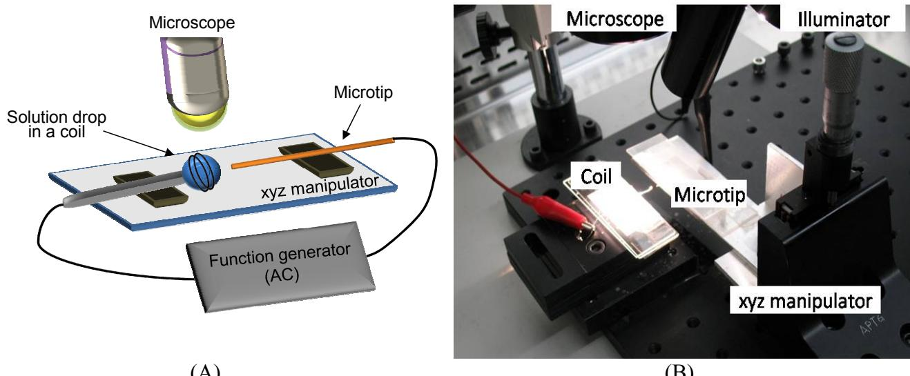
**Figure S2.** (A) Illustration of an experimental setup and (B) Photograph of the experimental setup.
