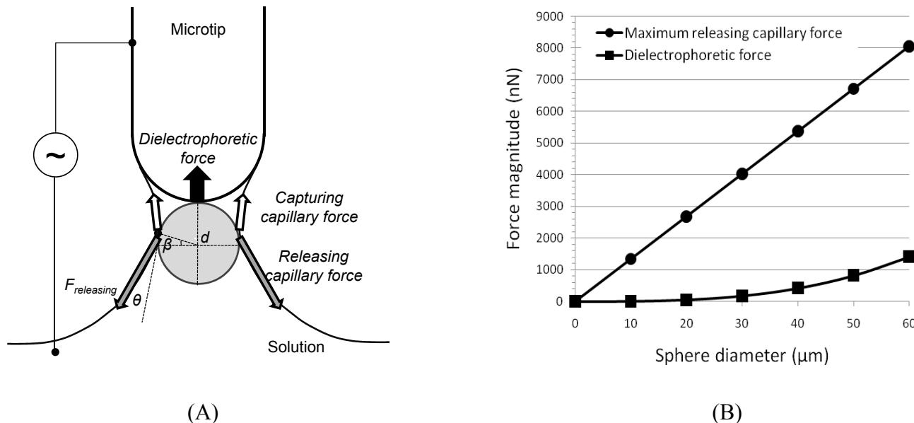
**Figure S3.** (A) Schematic of capillary- and dielectrophoretic force analysis (B) Capillary- and dielectrophoretic forces according to the various diameters of polystyrene spheres.
