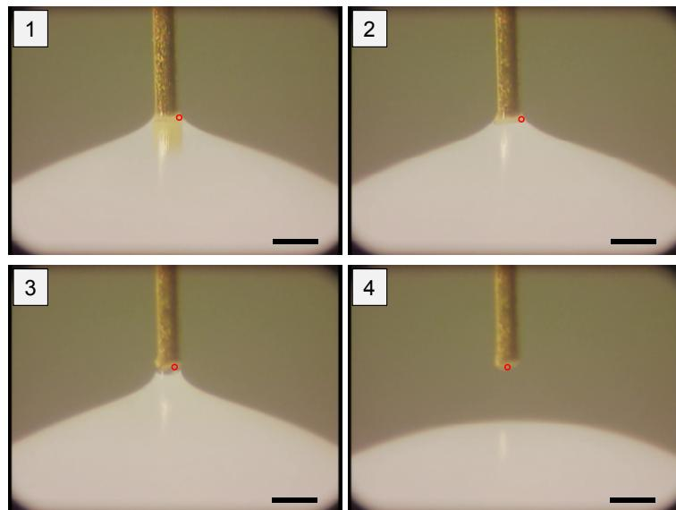
**Figure S1.** Sequential images ( $1 \rightarrow 4$ ) for sphere movement on a microtip surface in a withdrawal step (scale bars: 50  $\mu\text{m}$ ).
