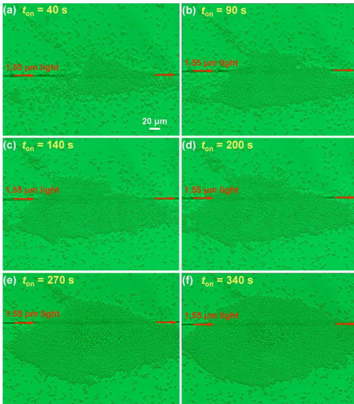
FIG. S1. CCD captured microscope images of the SiO<sub>2</sub> particles assembled from  $t_{\text{on}} = 40$  to 340 s. (a)  $t_{\text{on}} = 40 \text{ s}$ . (b)  $t_{\text{on}} = 90 \text{ s}$ . (c)  $t_{\text{on}} = 140 \text{ s}$ . (d)  $t_{\text{on}} = 200 \text{ s}$ . (e)  $t_{\text{on}} = 270 \text{ s}$ . (f)  $t_{\text{on}} = 340 \text{ s}$ .
