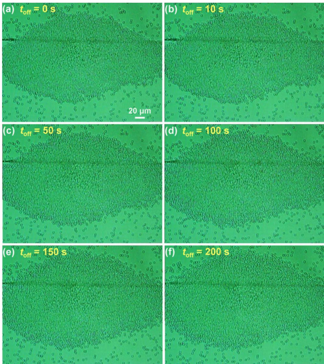
FIG. S2. CCD captured microscope images of the  $\text{SiO}_2$  particles diffused from  $t_{\text{off}} = 0$  to 200 s. (a)  $t_{\text{off}} = 0 \text{ s}$ . (b)  $t_{\text{off}} = 10 \text{ s}$ . (c)  $t_{\text{off}} = 50 \text{ s}$ . (d)  $t_{\text{off}} = 100 \text{ s}$ . (e)  $t_{\text{off}} = 150 \text{ s}$ . (f)  $t_{\text{off}} = 200 \text{ s}$ .
