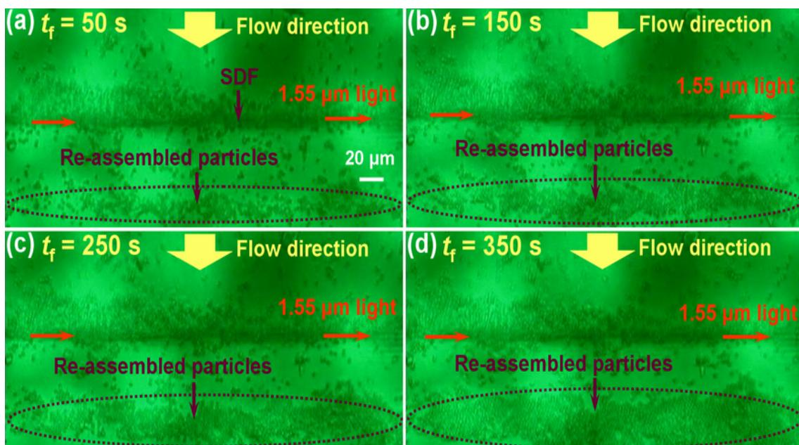
FIG. S9. The impact of flowing surrounding on the assembly of 3.14- $\mu\text{m}$ -diameter  $\text{SiO}_2$  particles by using a 1.4- $\mu\text{m}$ -diameter SDF. The yellow arrows show the follow direction which perpendicular to the SDF while the red arrows show the propagation direction of the 1.55  $\mu\text{m}$  light in the SDS. The flow rate is 4  $\mu\text{m}/\text{s}$ .  $t_f$  denotes the time duration of the flow applied.
