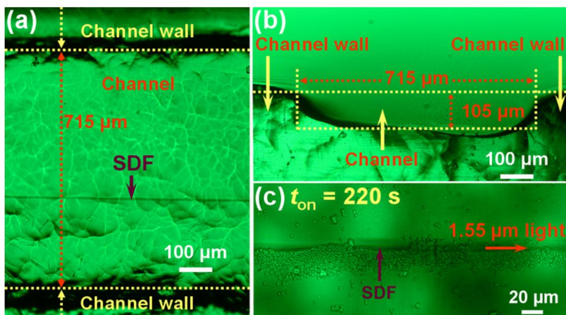
FIG. S8. Assembly of SiO<sub>2</sub> particles in a fluidic channel. (a) Microscope image of the SDF placed in the fluidic channel. (b) Microscope image of the cross section of the fluidic channel. (c) After launching an optical power of 200 mW into the SDF for 220 s, about 300 particles were assembled.
