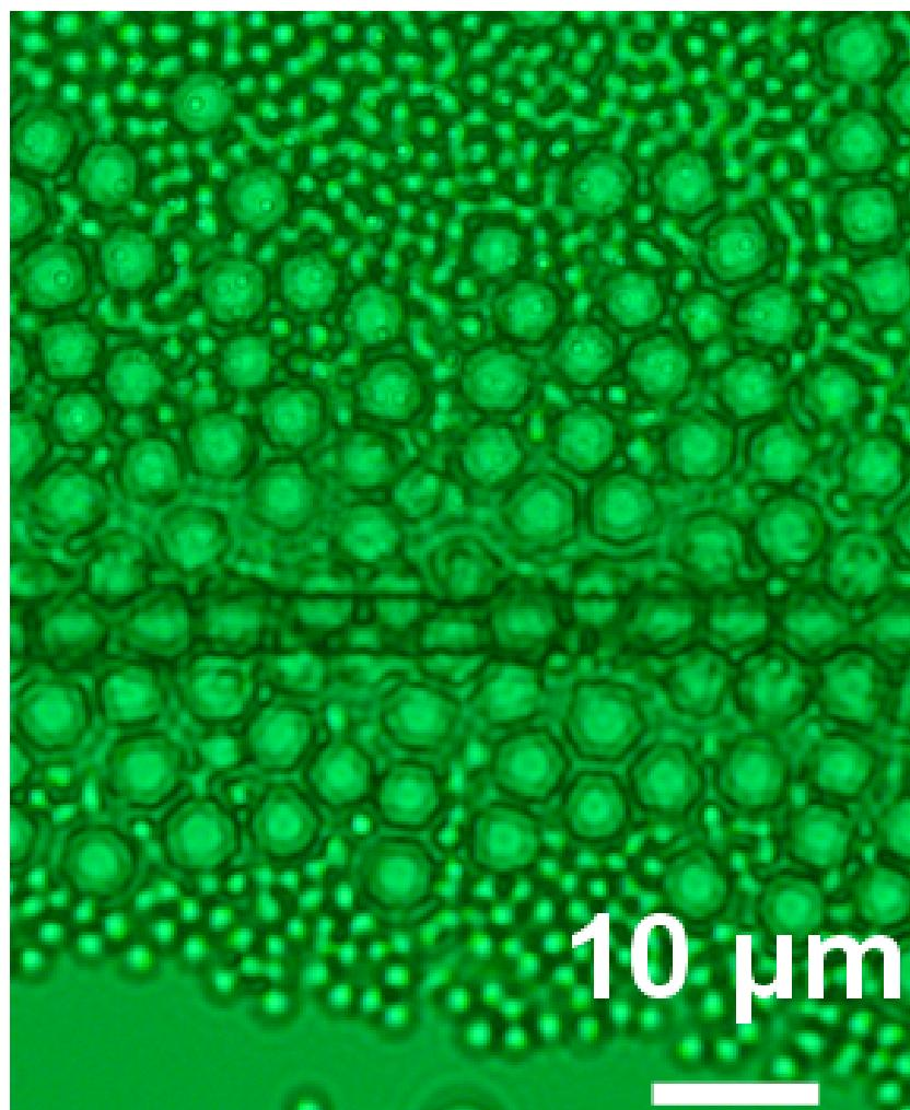
FIG. S6. Selective assembly of  $\text{SiO}_2$  particles with diameters of 2.08 and 5.65  $\mu\text{m}$  from a mixture.
