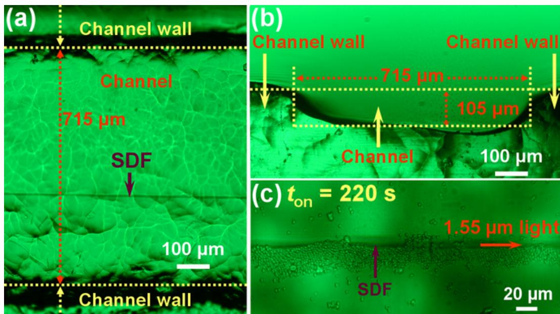
FIG. S8. Assembly of  $\text{SiO}_2$  particles in a fluidic channel. (a) Microscope image of the SDF placed in the fluidic channel. (b) Microscope image of the cross section of the fluidic channel. (c) After launching an optical power of 200 mW into the SDF for 220 s, about 300 particles were assembled.
