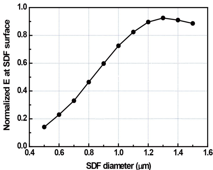
FIG. S7. Normalized electric field amplitude at the SDF surface with different diameters at the wavelength of 1.55- $\mu\text{m}$ .
