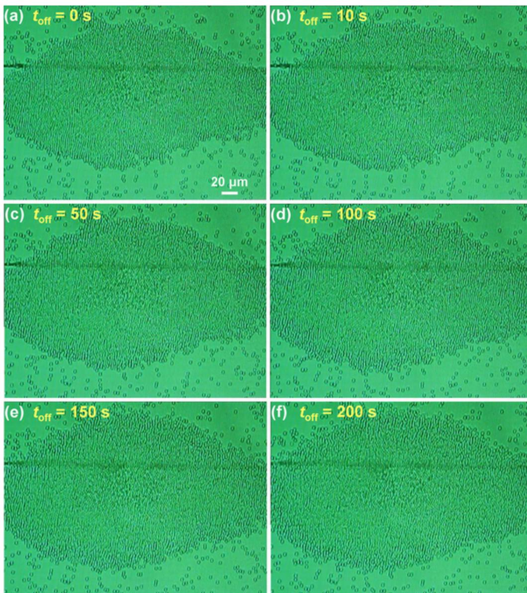
FIG. S2. CCD captured microscope images of the  $\text{SiO}_2$  particles diffused from  $t_{\text{off}} = 0$  to 200 s. (a)  $t_{\text{off}} = 0$  s. (b)  $t_{\text{off}} = 10$  s. (c)  $t_{\text{off}} = 50$  s. (d)  $t_{\text{off}} = 100$  s. (e)  $t_{\text{off}} = 150$  s. (f)  $t_{\text{off}} = 200$  s.
