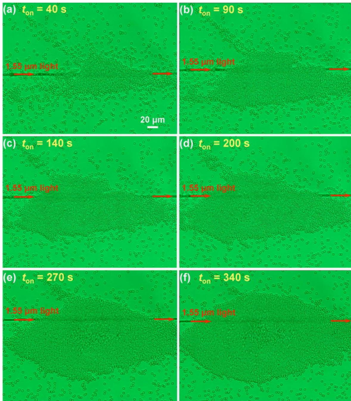
FIG. S1. CCD captured microscope images of the  $\text{SiO}_2$  particles assembled from  $t_{\text{on}} = 40$  to 340 s. (a)  $t_{\text{on}} = 40$  s. (b)  $t_{\text{on}} = 90$  s. (c)  $t_{\text{on}} = 140$  s. (d)  $t_{\text{on}} = 200$  s. (e)  $t_{\text{on}} = 270$  s. (f)  $t_{\text{on}} = 340$  s.
