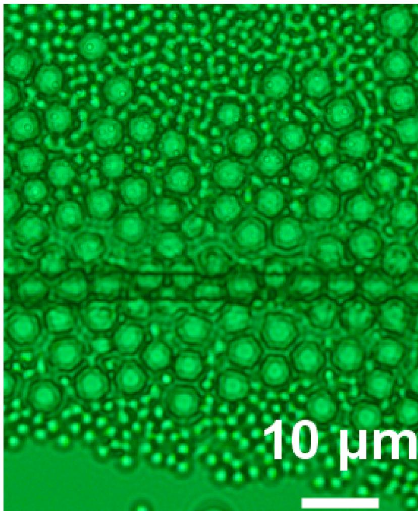
FIG. S6. Selective assembly of SiO<sub>2</sub> particles with diameters of 2.08 and 5.65 μm from a mixture.
