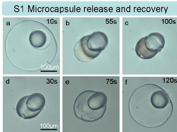
**Figure S1.** Process of the microcapsule release controlled by increasing temperature of ITO substrate as function of heating time (a to c) and microcapsule recovery when ITO substrate is cooled down at room temperature as a function of cooling time (d to f).
