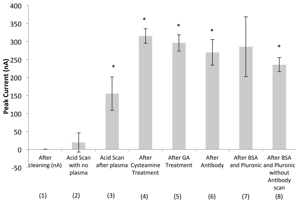
**Supplementary Figure 2** | Peak current from DPV method after every reaction step in the antibody conjugation method. Error bars represent  $\pm$  standard deviation, n=6. Numbers in brackets signify the step number.
