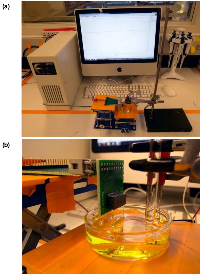
**Supplementary Figure 1 | Experimental setup.** (A) BASi Potentiostat (B) Close-up of electrochemical analysis set-up. Three-electrode system consisting of an Ag/AgCl electrode as the reference electrode, platinum wire as the auxiliary electrode, and the glass chip as the working electrode. Electrochemical signals were measured in 1X PBS containing 2mM Potassium Ferricyanide ( $K_3[Fe(CN)_6]$ ) and 2mM Potassium Ferrocyanide ( $K_4[Fe(CN)_6]$ ).
