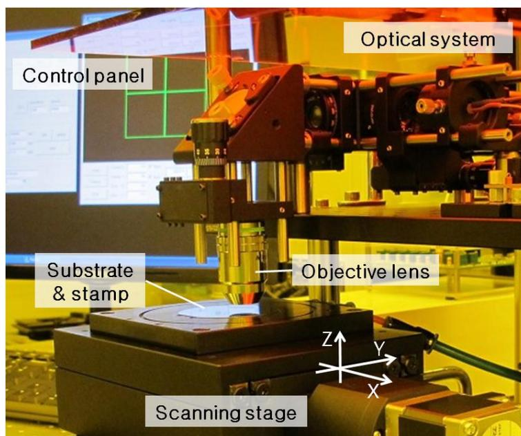
**Figure S4** A picture of the constructed FLB-NIL system. The upper part of the system consists of optical components to produce the focused laser beam. There is a scanning stage in the lower part to move the substrate in the X-Y directions.
