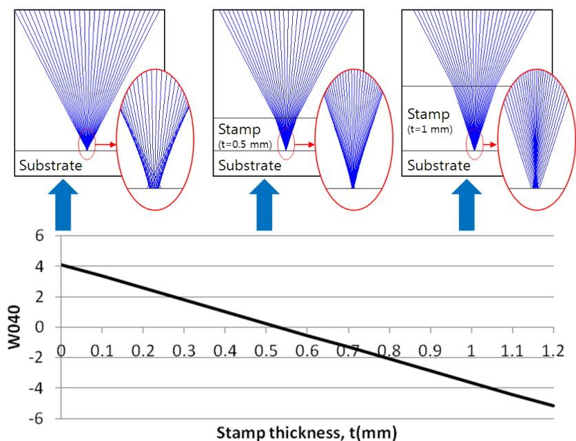
**Figure S3** Variations of the Seidel aberration coefficient  $W040$  due to the thickness of the transparent stamp in the designed optical layout. For the DLW mode ( $t = 0$  mm) and the FLB-NIL mode ( $t = 1$  mm), the Seidel aberration coefficient has the same values. Thus, the size of the focused laser beam will be the same.
