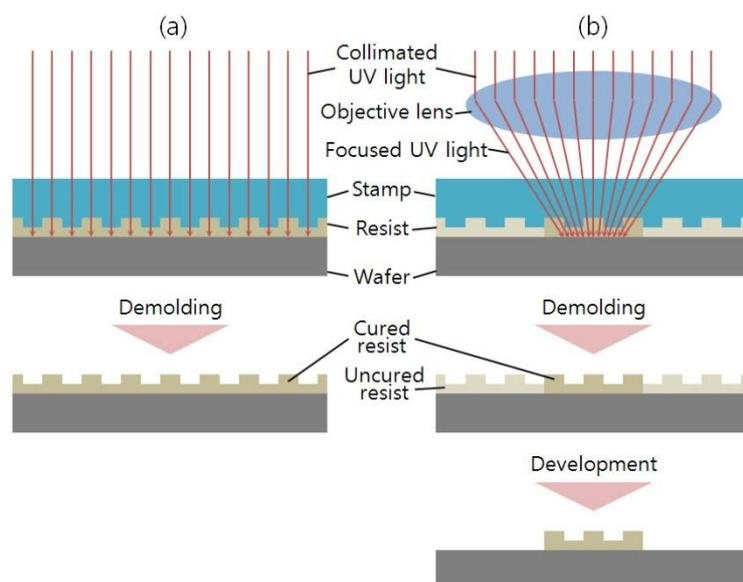
**Figure S1** Conceptual drawing of reducing the cured region of the resist in UV-NIL. a) Conventional UV-NIL process uses a collimated UV light to cure all the resist. b) If the UV light is focused by an objective lens, the cured region of the resist will be reduced. Then, the cured resist remains after development.
