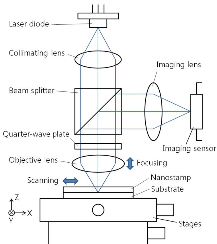
**Figure S2** The optical layout of the FLB-NIL system. The laser beam is collimated by a collimating lens and then focused by an objective lens. The reflected beam reaches the imaging sensor via a quarter-wave plate and a beam splitter. The focusing error can be monitored by signal processing of the imaging sensor.
