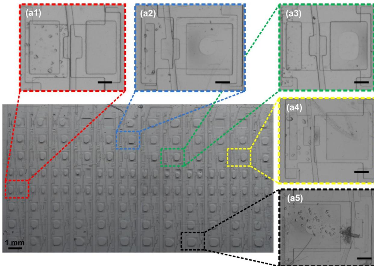
**Figure S2.** Optical micrograph of a 96-well hybrid array based screening chip showing screening of PhnA using the Index Screen. 12 different precipitants are screened in separate columns on a single chip. The enlarged views on top and side show initial crystal hits from condition (a1) I-42, (a2) I-47, (a3) I-54, (a4) I-70, and (a5) I-71 from the Index Screen. The scale bars in the insets correspond to 200  $\mu\text{m}$ .
