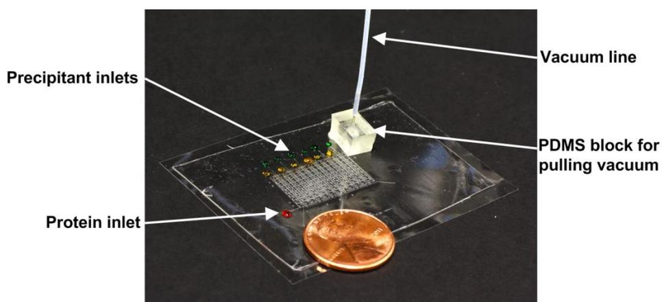
**Figure S1.** Optical micrograph showing the setup of a 96-well microfluidic array chip, including the placement of reagents droplets at inlets, and the way it is connected to a vacuum line to actuate sets of valves.
