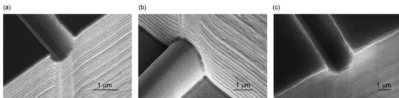
**Figure S3.** (a-c) SEM micrographs of the patching orifice after the main three steps of the fabrication process for the sample type B: silicon master, nickel insert, and replicated polymer part (from left to the right).
