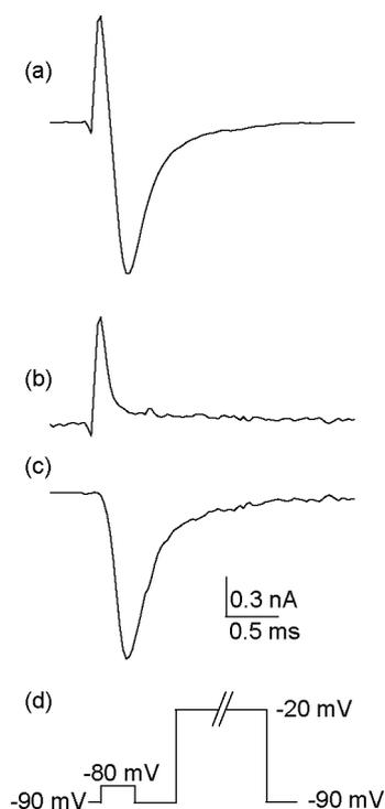
**Figure S1.** Leakage current subtraction using leak subtraction method. A) Whole-cell current recorded in response to voltage step from -90 mV (holding potential) to -20 mV. B) Leak current record produced by 10 mV test pulse multiplied by ratio between the two stimuli (70 mV/ 10 mV). C) Subtracted response of B from A in order to eliminate capacitive current. D) Voltage protocol.
