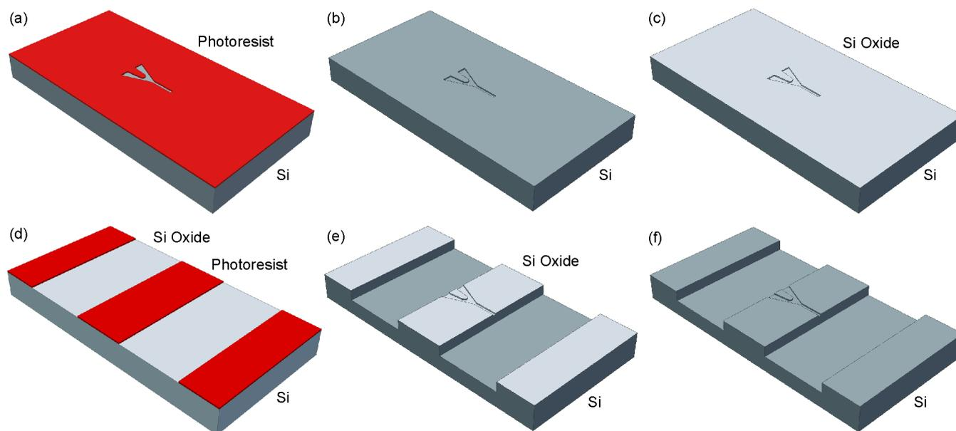
**Figure S2.** Schematics of the fabrication process for shaping the silicon after main steps: photolithography (a); silicon etching of the shallow patching channel (b); oxidation with 50 nm thick thermal silicon oxide (c); photolithography for the deep channel (d); oxide and silicon etching of the deep channels (e); oxide removal of the oxide mask (f).
