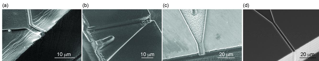
**Figure S4.** SEM micrographs of the capturing channel in the molded polymer chip. (a) In the beginning the orifice was blocked by accumulation of material during the demolding. (b) A circa 5 μm wide patching channel was successfully molded but many defects were present. (c) Tapered sidewalls in the deep channel gave a replica with no defects. (d) Device molded with the presented fabrication process.
