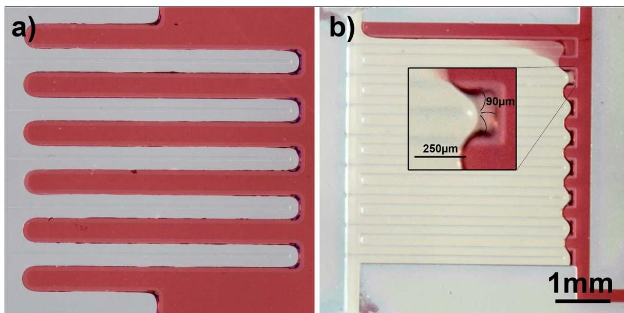
Fig S4: Influence of feature size on liquid guiding effect. Guiding structures are 60  $\mu\text{m}$  high in 150  $\mu\text{m}$  chambers. **a)** Large finger structures enable reliable filling. **b)** As the feature size approaches the vertical meniscus dimension, a critical corner prone to overflow is formed.
