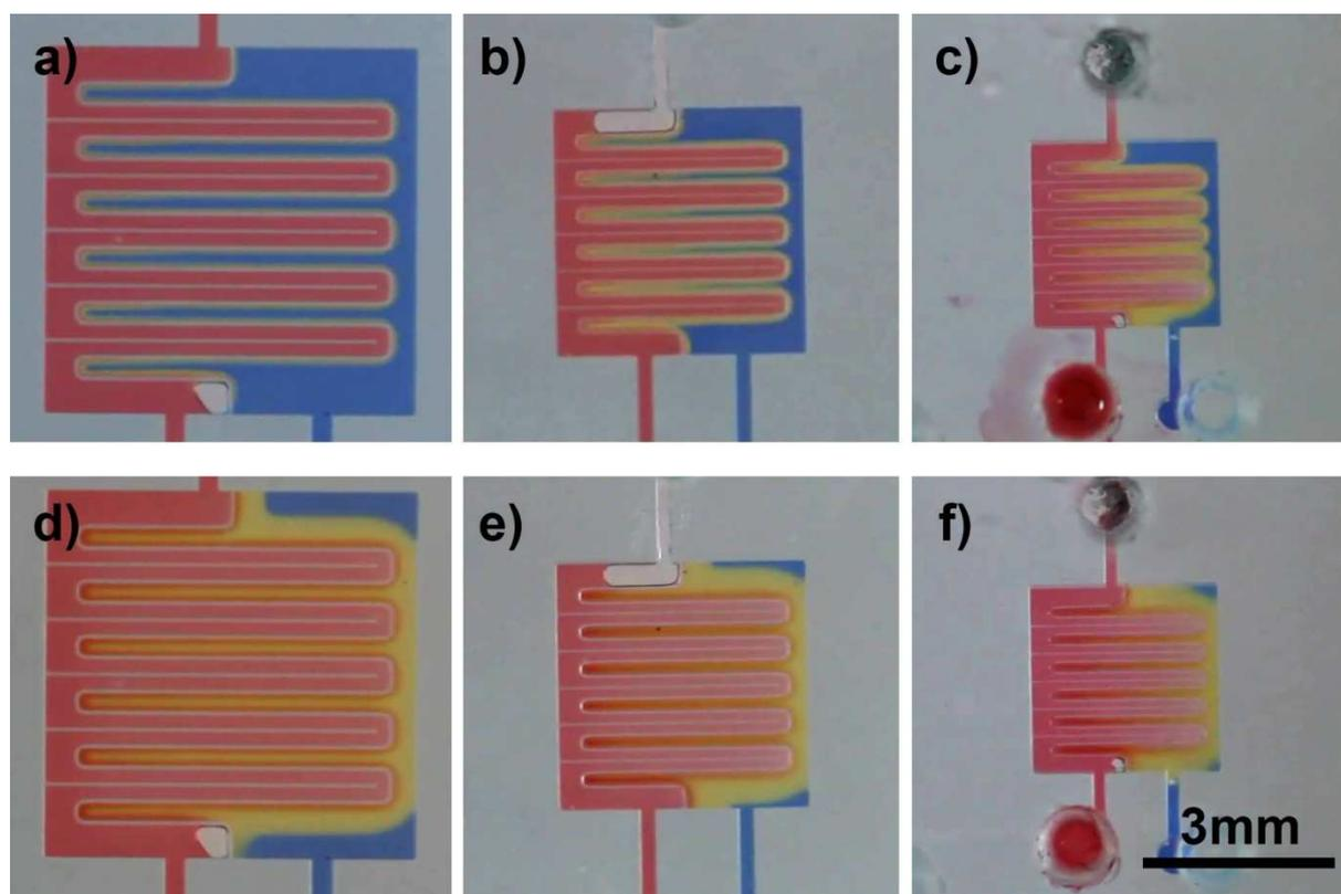
Fig S2: Test structures showing the influence of the chip geometry on the reaction speed. **a-c)** Picture taken 3s after sample injection. **a)** 6 mm chamber 450  $\mu\text{m}$  fingers. **b)** 4 mm chamber 300  $\mu\text{m}$  fingers. **c)** 3 mm chamber 225  $\mu\text{m}$  fingers. **d-f)** 2 min after sample injection. Both, the pH reaction as well as the red dye diffusion are considerably faster as the gel finger width decreases.
