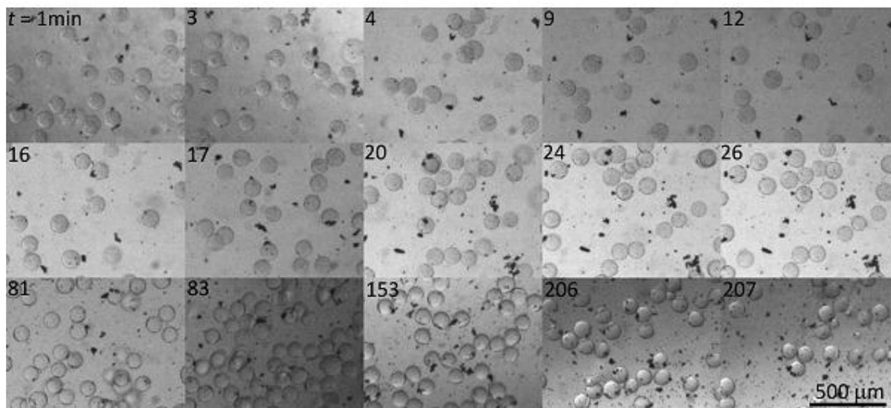
No morphological changes are observed in the delivery vehicles over time at 37 °C and in buffered conditions (pH = 7.4) during more than 200 min. Significant breakage of the delivery vehicles was observed after that time period.
