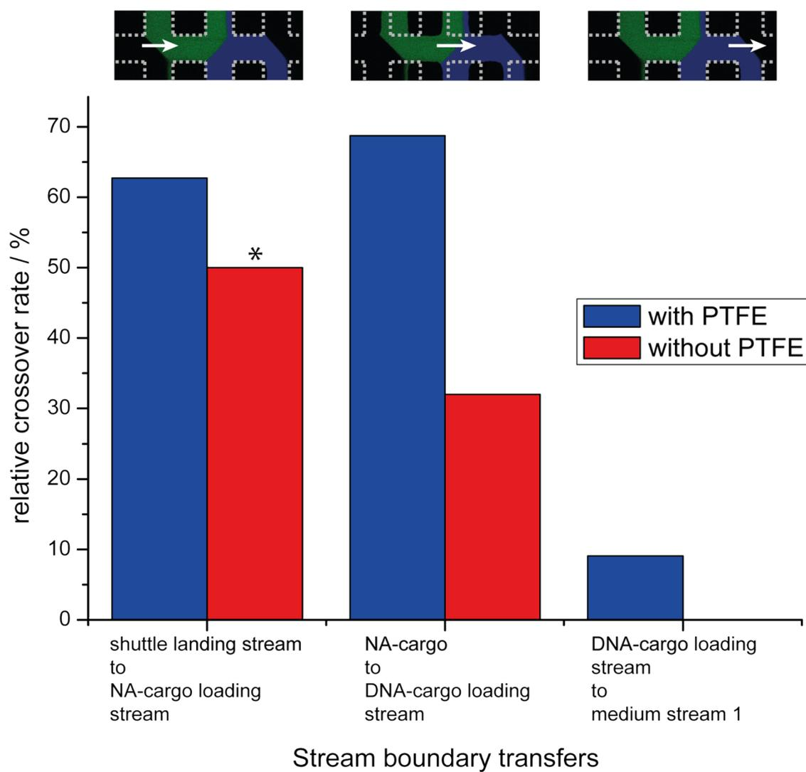
**Figure S7:** Probability of stream boundary crossings. The relative stream boundary crossover rates of nanoshuttles are given at each stream boundary (shuttle landing to NA-cargo loading stream, NA-cargo loading to DNA-cargo loading stream and DNA-cargo loading stream to medium stream 1). The rates in red were obtained in the channel presented in Figure S5, the rates in blue were obtained in the channel that had been coated with PTFE nanotracks presented in Figure S6.
