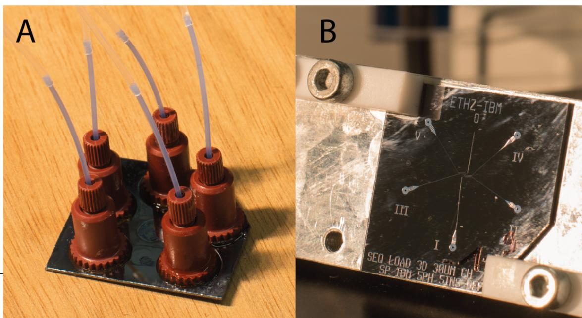
**Figure S1:** Photographs of the microfluidic chip fabricated in silicon. **A:** View from above: Tubing is connected to the chip via nanoports. **B:** View from below: The channels as well as the inlet ports I-V including dust traps are visible.
