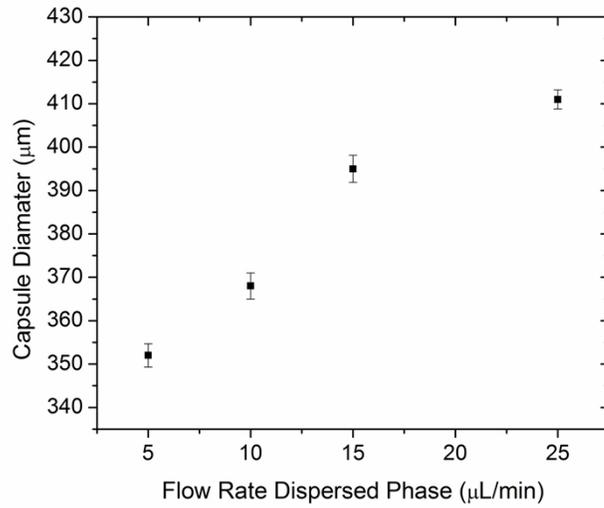
**Figure S1.** (a) The effect of dispersed fluid rate flow rate on capsule diameter. The outer fluid flow rate was held constant at 80 μl/min.
