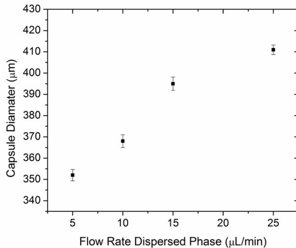
**Figure S1.** (a) The effect of dispersed fluid rate flow rate on capsule diameter. The outer fluid flow rate was held constant at 80 μl/min.
