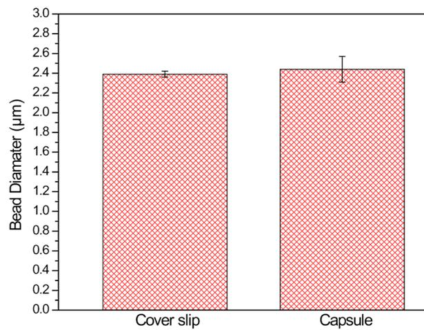
**Figure S2.** Size of Carboxylate-modified fluorescently labeled silica beads imaged on a cover slip and in the capsule shell. Capsules prepared using 0.1 wt.% polymer solution, aqueous ph 2.7, and 0.04 wt.% beads in the aqueous phase.
