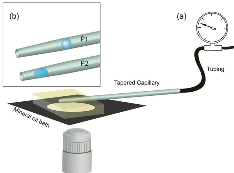
**Figure S6.** (a) Experimental setup for micromechanics experiments. (b) The microcapsule deforms in the tapered capillary as the pressure is increased from P1 to P2.
