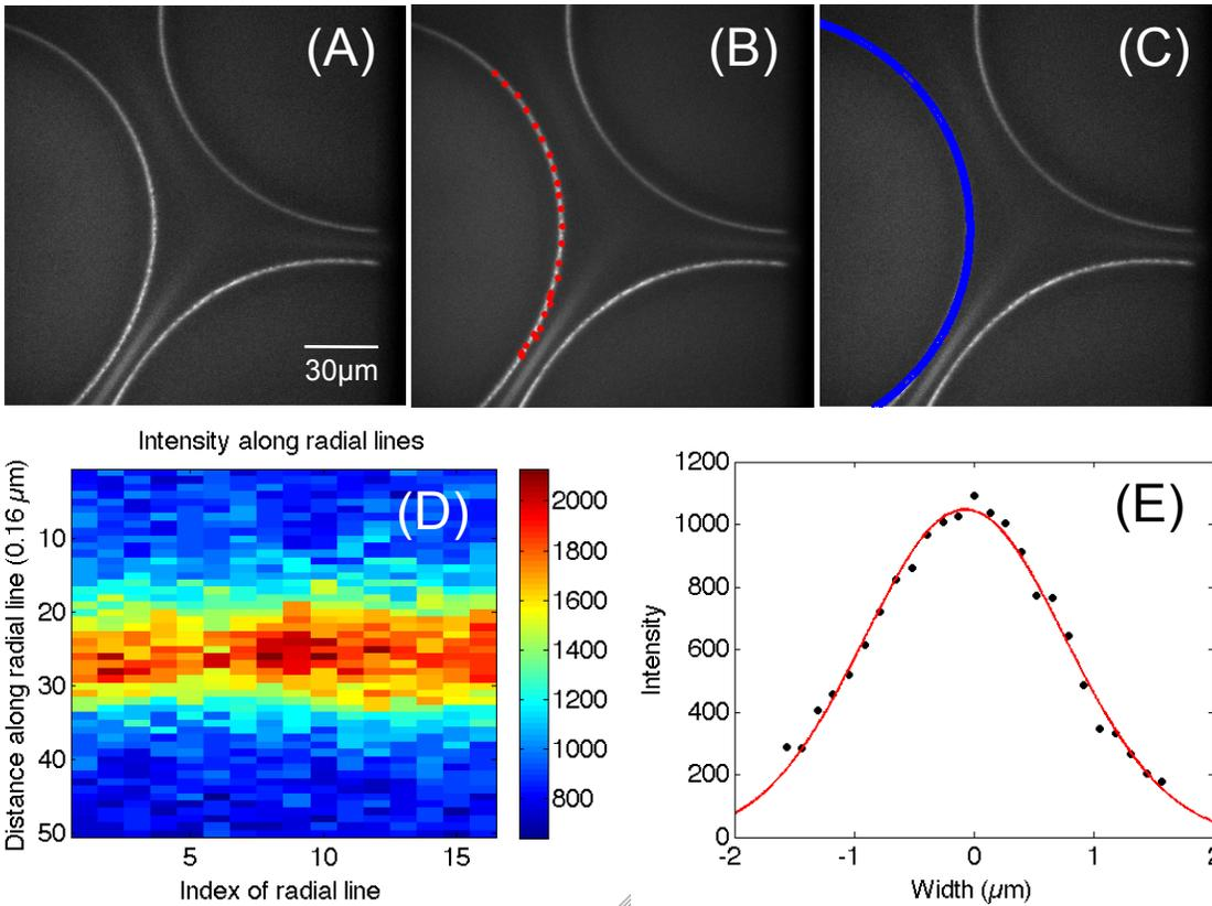
**Figure S3.** An example of analysis of confocal image of microcapsules to determine shell thickness. A) Confocal Image of Microcapsules. B) 25 Points are chosen along the capsule wall. C) Fitting an Arc to selected points D) Intensity profiles of average of radial lines drawn along the arc. E) Gaussian fitted to intensity profile.
