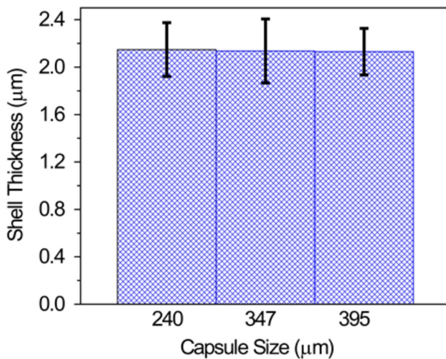
**Figure S7.** Capsule shell thickness as a function of capsule size. Capsules were prepared using 0.1 wt.% solutions at aqueous pH of 2.7 ,and in the absence of salt.
