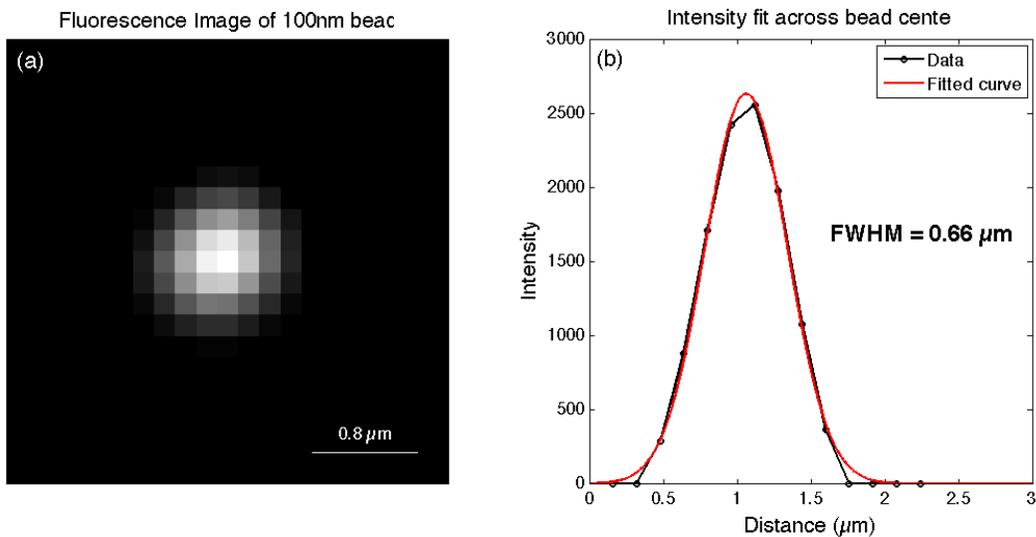
**Figure S4.** (a) Example image of a 100nm diameter bead acquired under the same imaging conditions as microcapsules. (b) Intensity profile along a line across the diameter of the bead fitted with a Gaussian.
