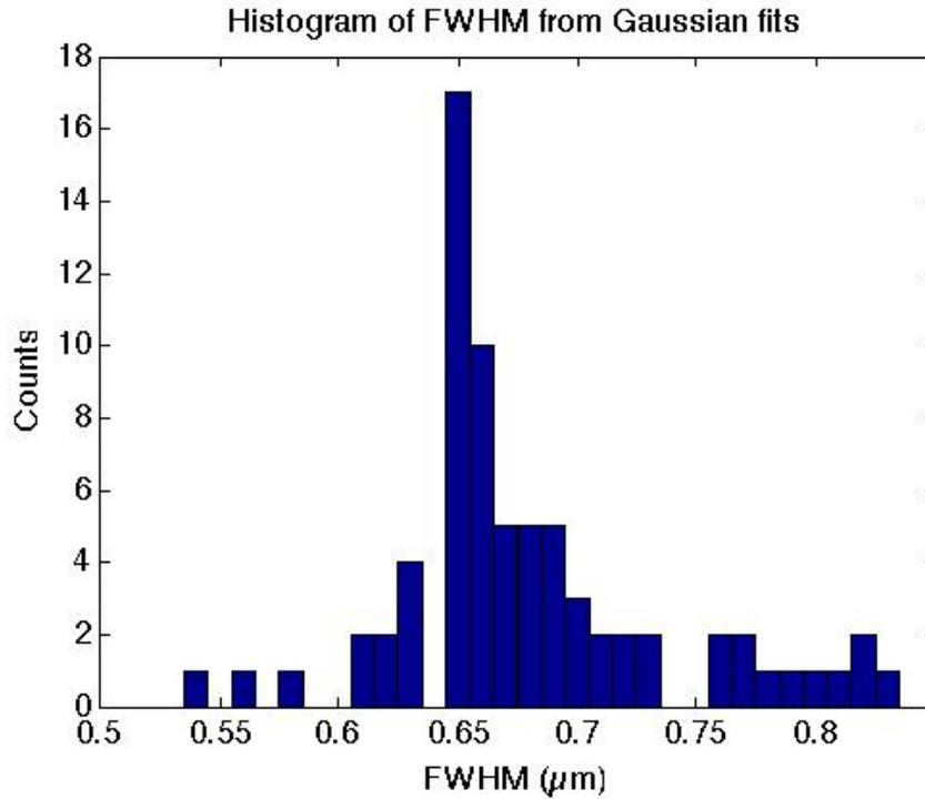
**Figure S5.** Histogram of full width at half maximum (FWHM) from Gaussian fits to profiles as in the example image (Fig. S4). Histogram includes FWHM from 73 beads.
