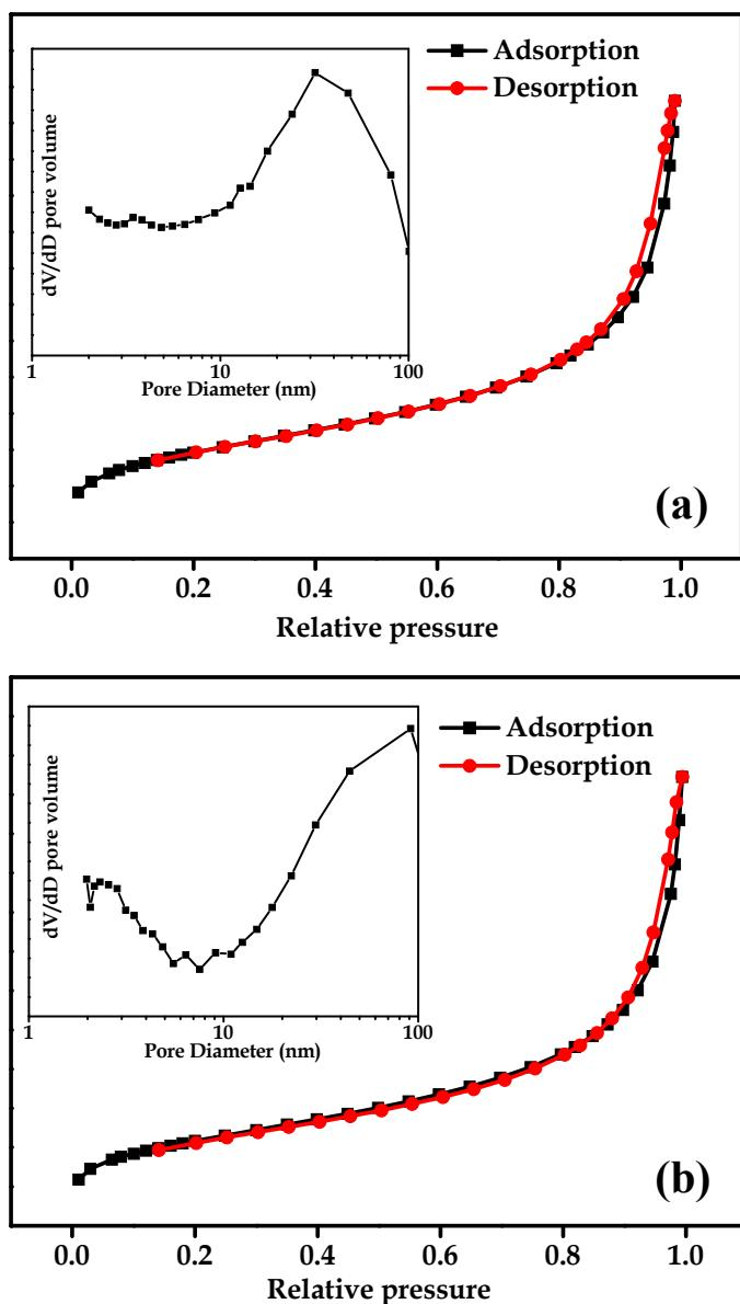
**Figure SI9** Sorption isotherms and corresponding pore size distribution curves (insets in each picture) of the supercritical  $\text{CO}_2$  dried (a) and freeze dried (b) MWCNT/Fe<sub>3</sub>O<sub>4</sub> composite aerogels
