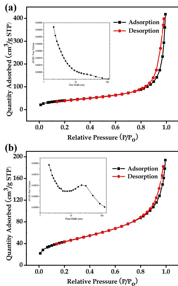
**Figure SI7** Sorption isotherms and corresponding pore size distribution curves (insets in each picture) of the supercritical  $\text{CO}_2$  dried (a) and freeze dried (b) MWCNT aerogels
