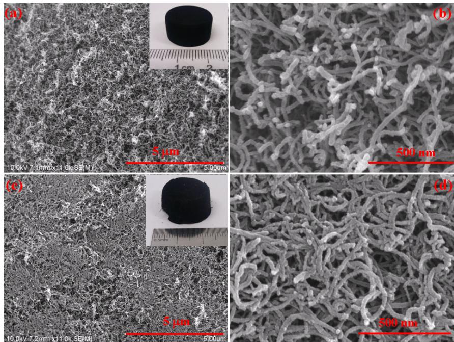
**Figure SI5.** Typical SEM images of the resulting carbon nanotube aerogels processed with supercritical CO<sub>2</sub> drying (a, b) or freeze drying (c, d). Insets in (a) and (c) are the digital photos of the monolithic carbon nanotube aerogels processed with supercritical CO<sub>2</sub> drying and freeze drying, respectively
