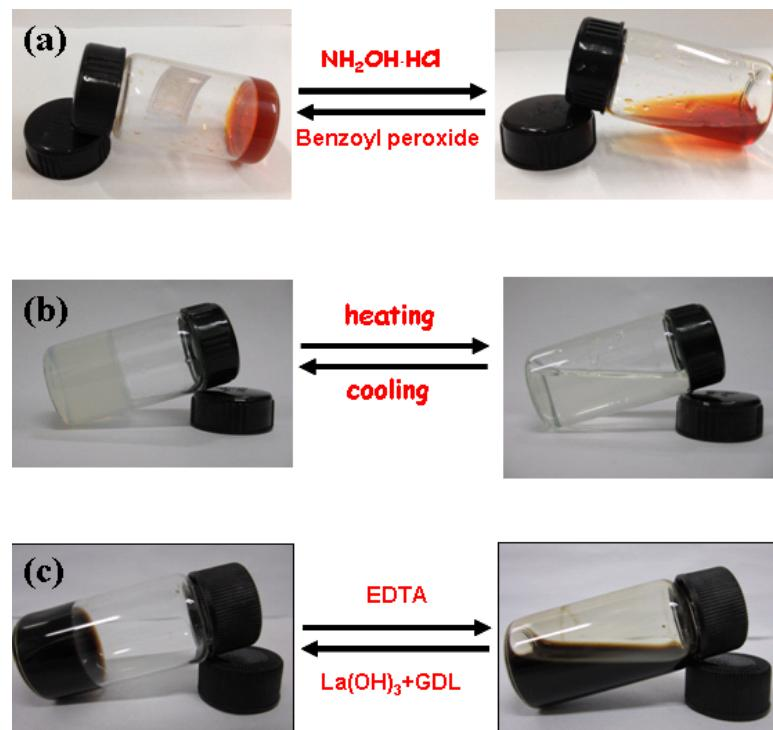
**Figure SI10** Sol-gel transitions of the Fe-H<sub>3</sub>BTC gel (a), agarose gel (b) and graphene oxide gel (c), respectively.
