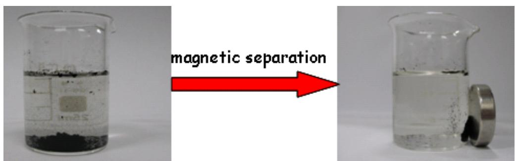
**Figure SI4** Magnetic separation of the MWCNT/Fe<sub>3</sub>O<sub>4</sub> composite aerogel from the aqueous solution after adsorption of the organic dye molecules.
