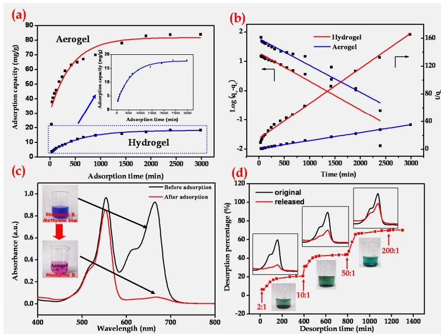
**Figure SI3.** Adsorption capacities at intervals (a) and corresponding kinetic model fits (b) of the dendrimer-crosslinked MWCNT hydrogel and aerogel as the adsorbent for MB removal, selective adsorption behavior (c) of the MWCNT aerogel toward the mixture of the MB and RhB, and controllable desorption behavior (d) of the MWCNT aerogel through addition of the dendrimer PAMAM.
