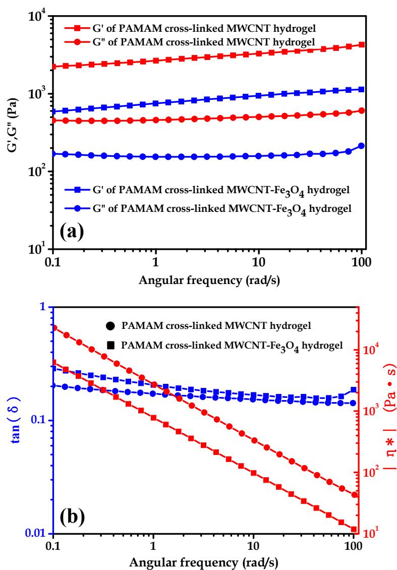
**Figure SI8** Rheological investigation on the as-made MWCNT hydrogel and MWCNT/ $\text{Fe}_3\text{O}_4$  composite hydrogel.
