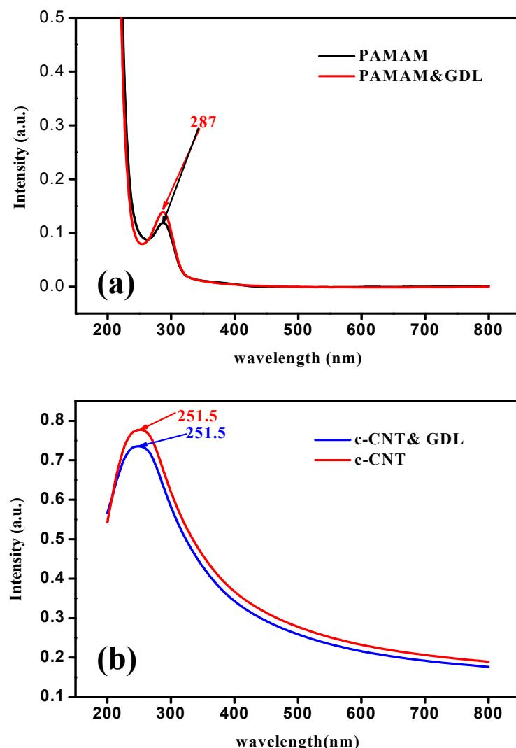
**Figure SI1** UV-vis spectra of the mixtures between GDL and PAMAM (a) or between GDL and carboxylic carbon nanotubes (b). Both of the UV spectra shows no obvious peak shifts, revealing that GDL has no interaction with both PAMAM and MWCNTs, which guarantees that superfluous GDL and its hydrolyzed product can be removed completely from the resulting hydrogel after solvent-exchange process.
