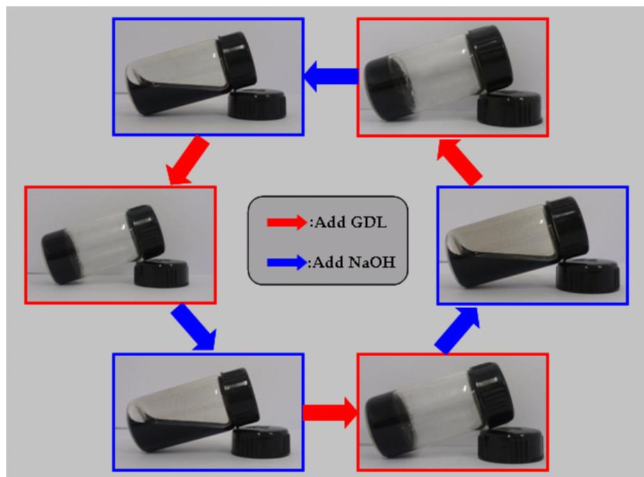
**Figure SI2.** Reversible sol-gel transition of the PAMAM-crosslinked MWCNT/Fe<sub>3</sub>O<sub>4</sub> composite hydrogel
