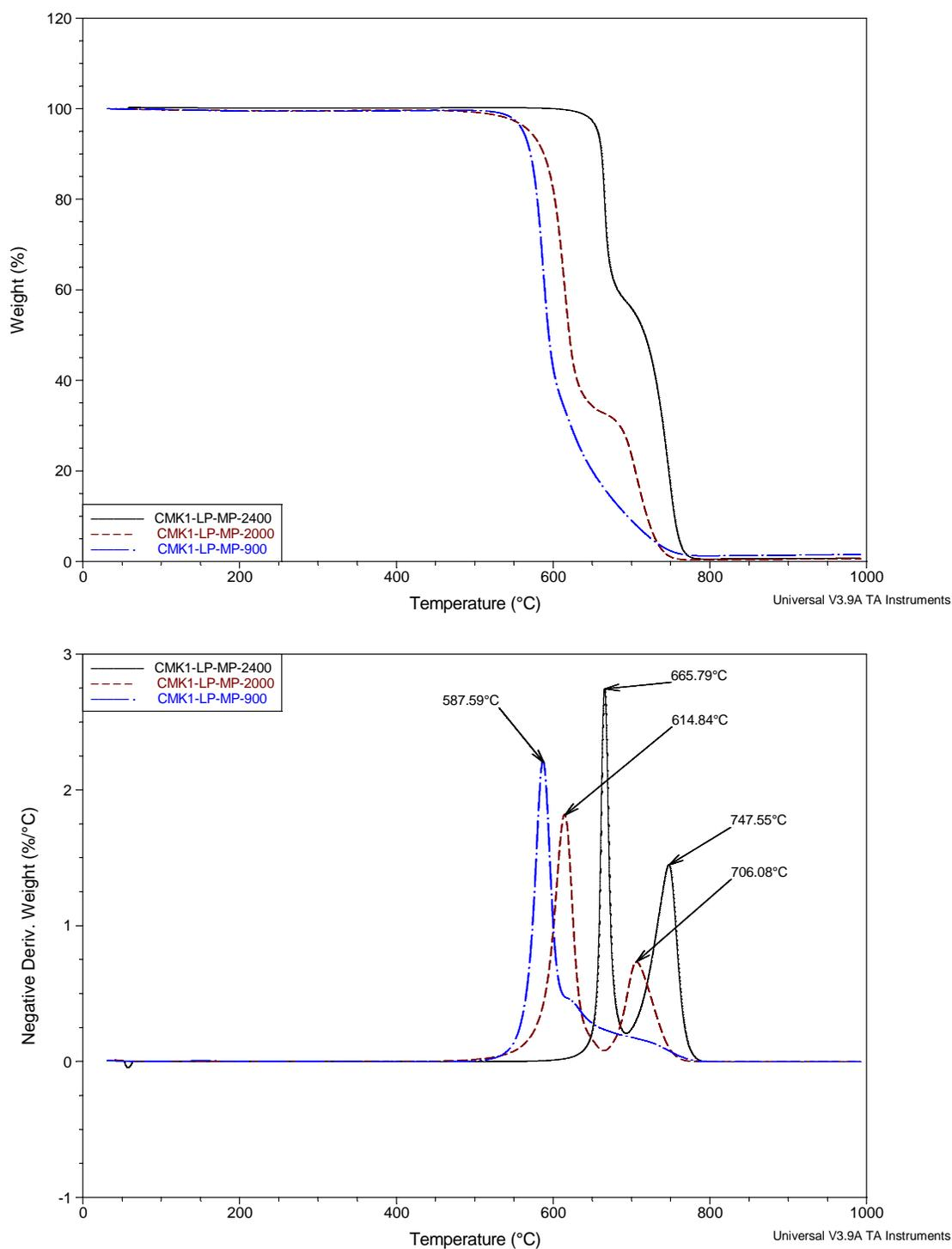
**Figure ESI-3.** TG (top) and DTG (bottom) profiles for the CMK1-LP-MP samples prepared at 900, 2000 and 2400 °C. The second weight loss (at higher temperature) is related to the oxidation of graphitic domains; it is about 33% and 49% for the carbons graphitized at 2000 and 2400°C, respectively.
