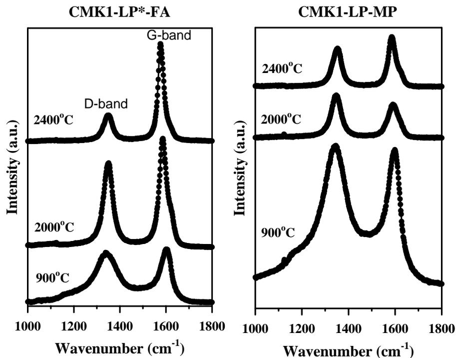
**Fig. ESI-4** Raman spectra for the CMK1-LP\*-FA and CMK1-LP-MP carbons prepared at 900, 2000 and 2400 °C; these spectra were collected on a high-resolution dispersive Raman microscope (LabRAM HR UV/Vis/NIR, Horiba Jobin Yvon), by the addition of four spectra with collection times of 40s each. The measurement was performed with a 514.5 nm line of an argon ion laser at room temperature. The integrated intensity ratio for the D and G bands ( $I_D/I_G$ ) is given below:
