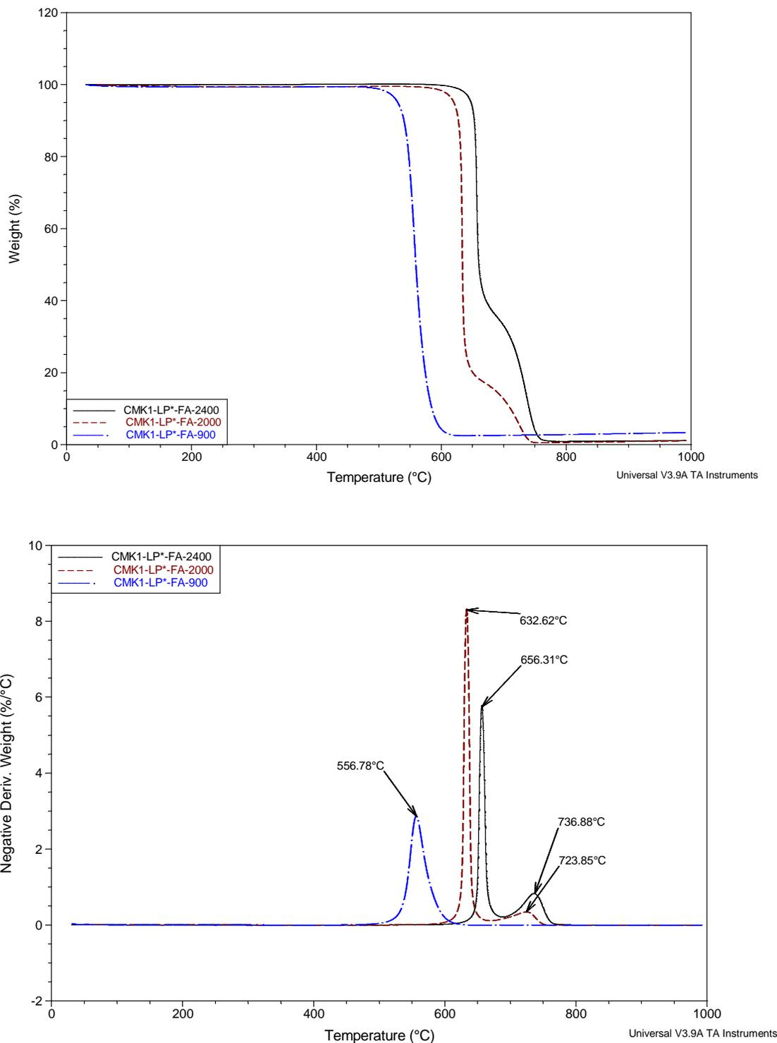
**Figure ESI-2.** TG (top) and DTG (bottom) profiles for the CMK1-LP\*-FA samples prepared at 900, 2000 and 2400 °C. While one-step oxidation profile is visible for the sample at 900 °C, the samples graphitized at 2000 and 2400°C show two-step weight loss profiles. The second weight loss (at higher temperature) is related to the oxidation of graphitic domains; it is about 17% and 35% for the carbons graphitized at 2000 and 2400°C, respectively.
