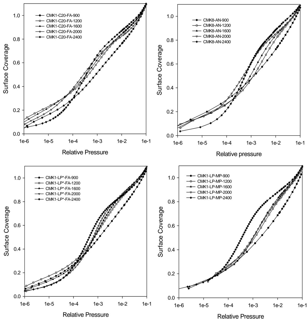
**Figure ESI-1.** Low-pressure adsorption isotherms plotted at a semi-logarithmic scale for series of the CMK1-C20-FA, CMK8-AN, CMK1-LP\*-FA and CMK1-LP-MP carbons.
