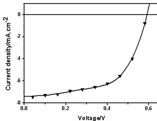
**Fig.2** I-V characteristics of the PV device with the structure of ITO/PEDOT:PSS/P3HT:PC<sub>61</sub>BM/LiF/Al under an illumination of AM 1.5 G (80 mW cm<sup>-2</sup>).
