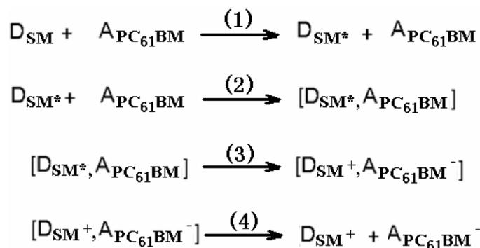
**Scheme. 1** Mechanism for photoinduced charge separation of synthesized donor molecules ( $D_{SM}$ ) and acceptor PCBM ( $A_{PC_{61}BM}$ ): (1) photoexcitation of  $D_{SM}$ ; (2) diffusion of the exciton and formation of an encounter pair; (3) electron transfer to form a geminate pair; (4) charge separation.
