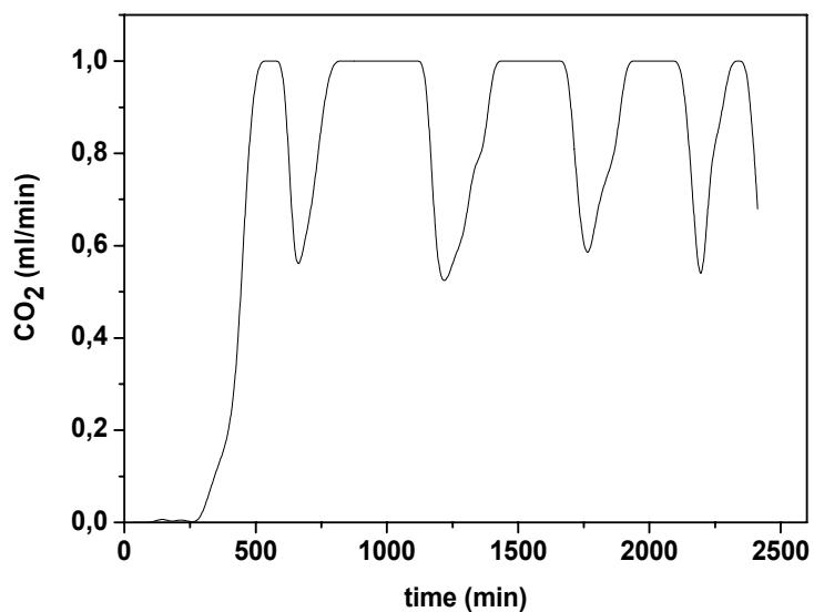
**Figure SI.7** Produced  $\text{CO}_2$  versus time for AU2/ZnO.
