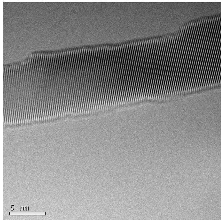
**Figure SI.2 HRTEM of a single ZnO nanorod.**
