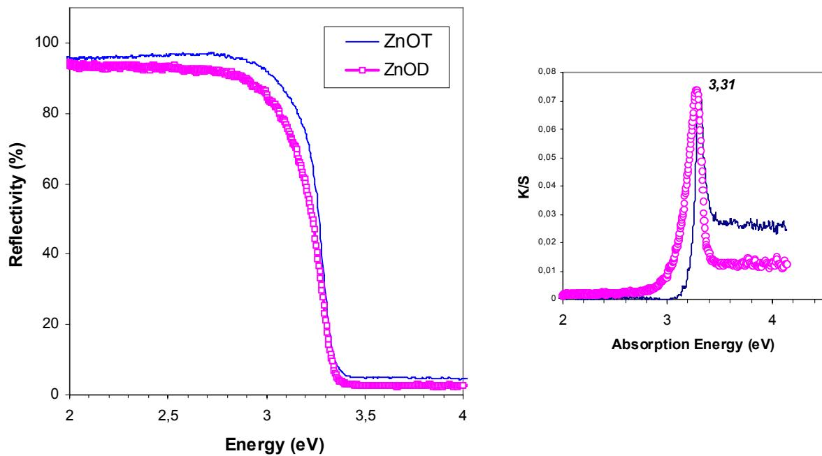
**Figure SI.3** Diffuse reflectance spectra of  $\text{ZnO}_T$  and  $\text{ZnO}_D$  powders at 298 K. The plot of the Kubelka Munk function for the two spectra is shown on the right.
