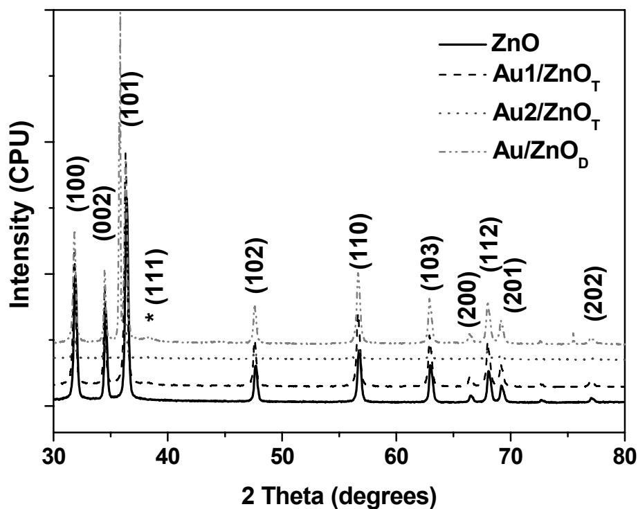
**Figure SI.5** Powder X-ray diffractograms of the pure ZnO<sub>T</sub> support and Au/ZnO catalysts.
