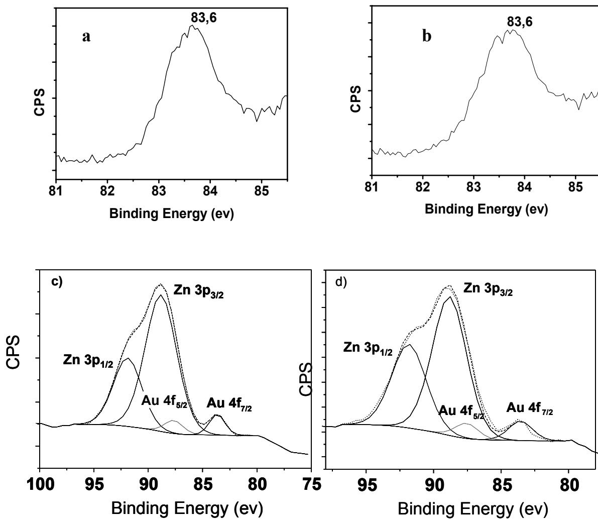
**Figure SI6** XPS spectra of Au/ZnO<sub>D</sub> a) before and b) after reaction, c) the complete spectrum before reaction, and d) the complete spectrum after reaction.
