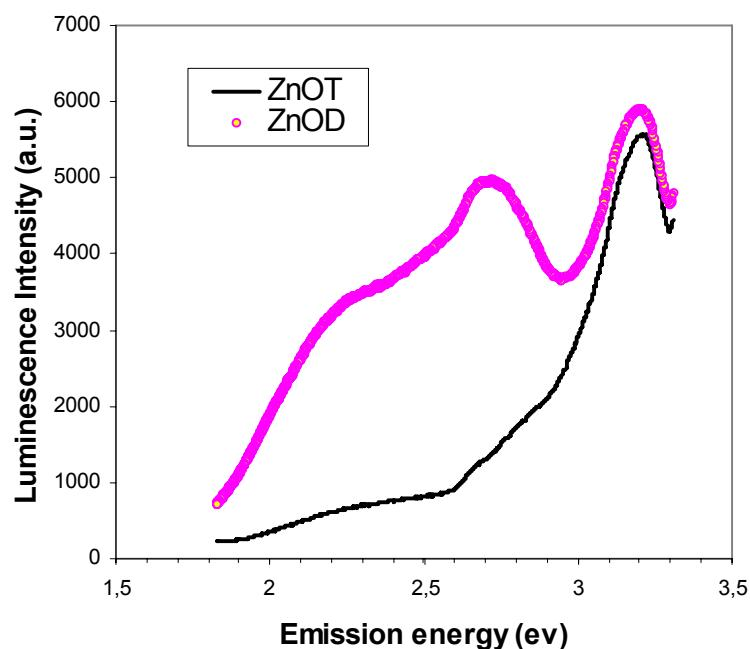
**Figure SI.4 Luminescence spectra of  $\text{ZnO}_T$  and  $\text{ZnO}_D$  powders at 298 K.**
