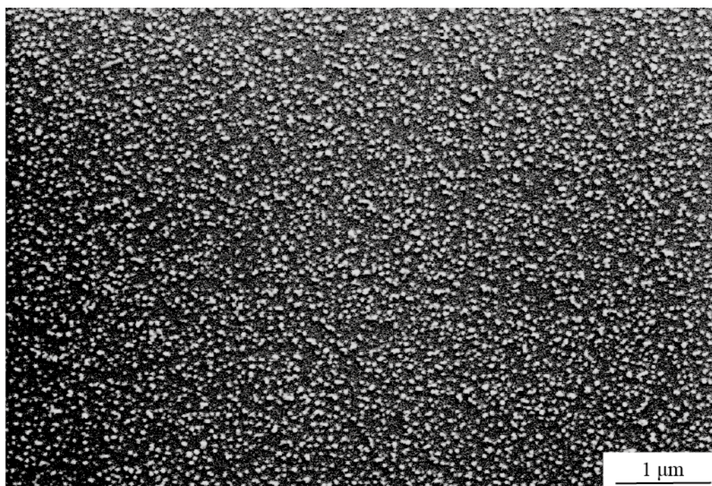
Fig. S11 SEM image of psNP deposited on a glass slide. The glass slide was covered with PEI and immersed for 30 min into a psNP solution with a salt concentration of 10 mM.
