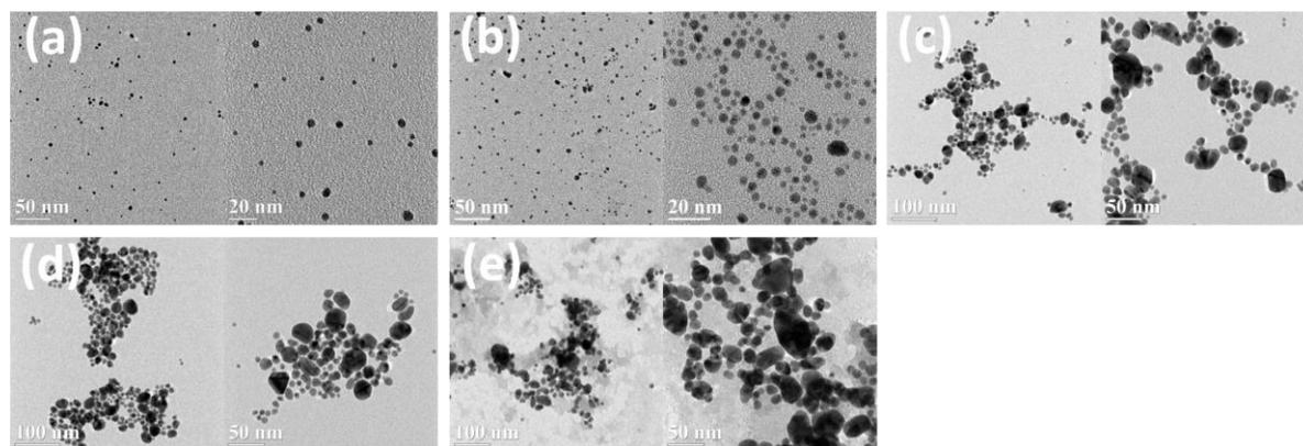
Fig. S1. TEM analysis of the gold nanoparticles prepared using AuBP1 at an Au/peptide ratio of (a) 2:1, (b) 4:1, (c) 10:1, (d) 20:1, (e) 40:1 with peptide concentration fixed at 0.1 mM.
