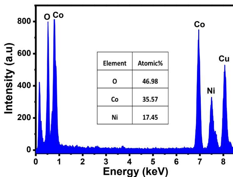
Fig. S1. EDS spectrum and analyzed atomic % of Co, Ni and O (inset) for the spinel  $\text{NiCo}_2\text{O}_4$  annealed at 673 K for 2 h.
