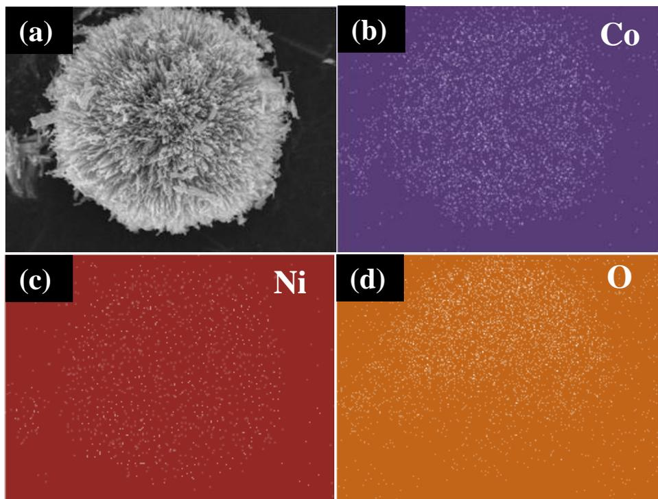
Fig. S2 (a) FE-SEM image and corresponding EDS elemental mapping for (b) Co, (c) Ni, and (d) O.
