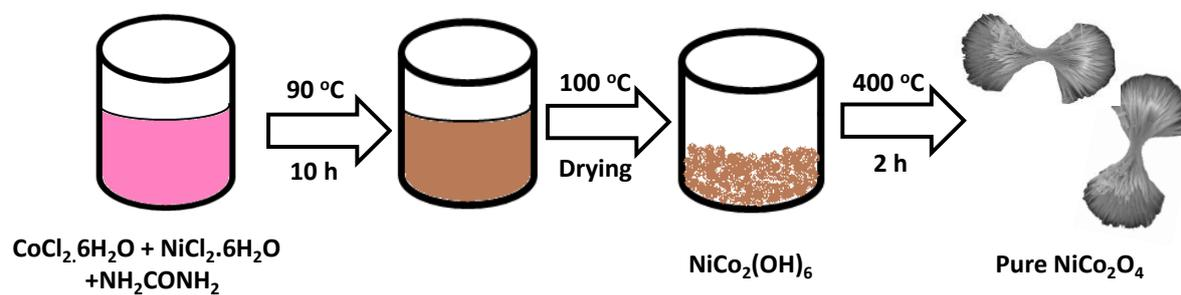
Scheme 1. Schematic illustration of synthesis of urchin-like  $\text{NiCo}_2\text{O}_4$ .
