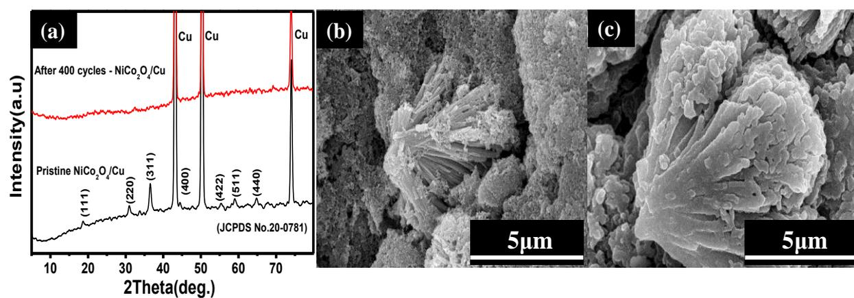
Fig. S4 (a) XRD patterns and FE-SEM images (b) before and after (c) 400 cycles of NiCo<sub>2</sub>O<sub>4</sub>/Cu electrode at 0.5 C rate.
