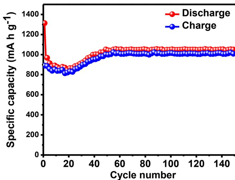
Fig. S3 Cyclability of the  $\text{NiCo}_2\text{O}_4$  electrode discharged and charged at 0.1 C.
