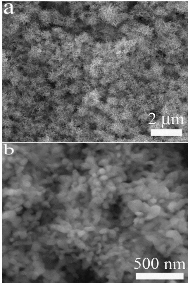
**Fig. S6** SEM images of the sample obtained from heat treatment of  $\text{Ni}_{1/3}\text{Mn}_{2/3}\text{CO}_3$  precursor without using PAN. It is clearly to see that the tremella-like structure has collapsed.
