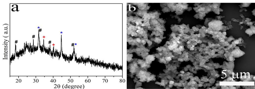
**Fig. S3** (a) XRD pattern and (b) SEM images of the sample using  $\text{MnSO}_4$  and  $\text{NiCl}_2$  as raw materials.
