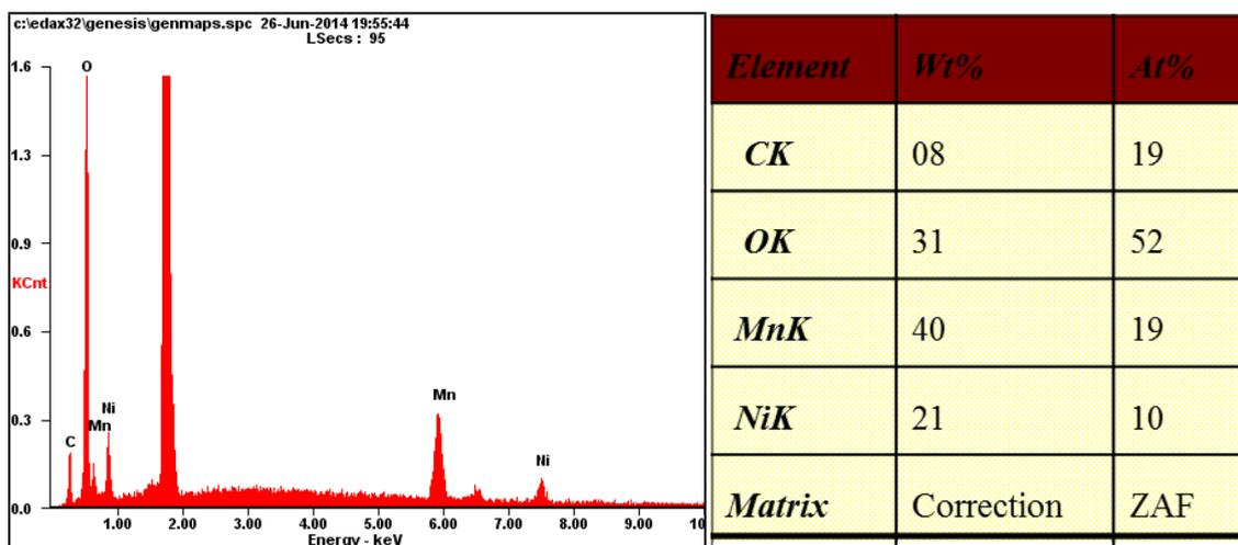
**Fig. S4** Energy dispersive spectroscopy (EDS) of the carbonate precursor, the elements of C, O, Mn and Ni can be detected and the strong peak is attributed to the Si wafer. The ratio of Mn and Ni is about 2:1, based on which the precursor can be confirmed as  $\text{Ni}_{1/3}\text{Mn}_{2/3}\text{CO}_3$ .
