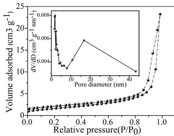
**Fig. S11** N<sub>2</sub> adsorption–desorption isotherms with an inserted pore size distribution of porous tremella-like NiMn<sub>2</sub>O<sub>4</sub>/C hierarchical nanostructure.
