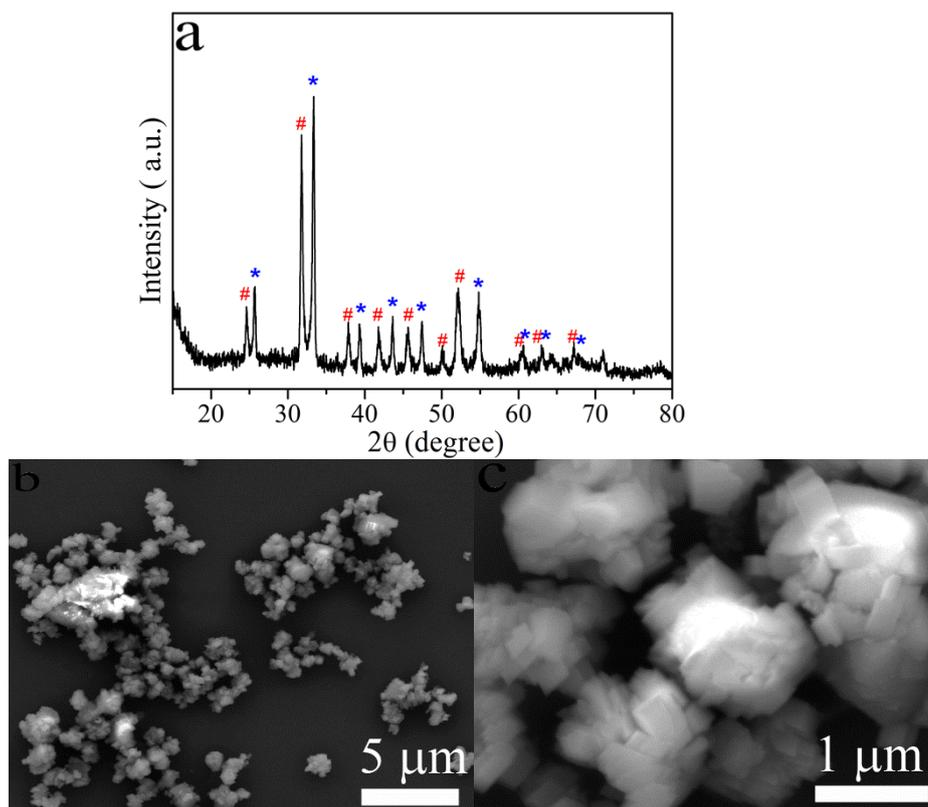
**Fig. S1** (a) XRD and (b) SEM images of the carbonate precursor formed in the water. The divided XRD patterns indicate that the obtained carbonate precipitate is a mixture of  $\text{NiCO}_3$  (# JCPDS No: 78-0210) and  $\text{MnCO}_3$  (\* JCPDS No: 86-0173), indicating the importance of TEG for the preparation of bimetallic carbonate precursor. And the morphology of the carbonate precipitate is irregular aggregate.
