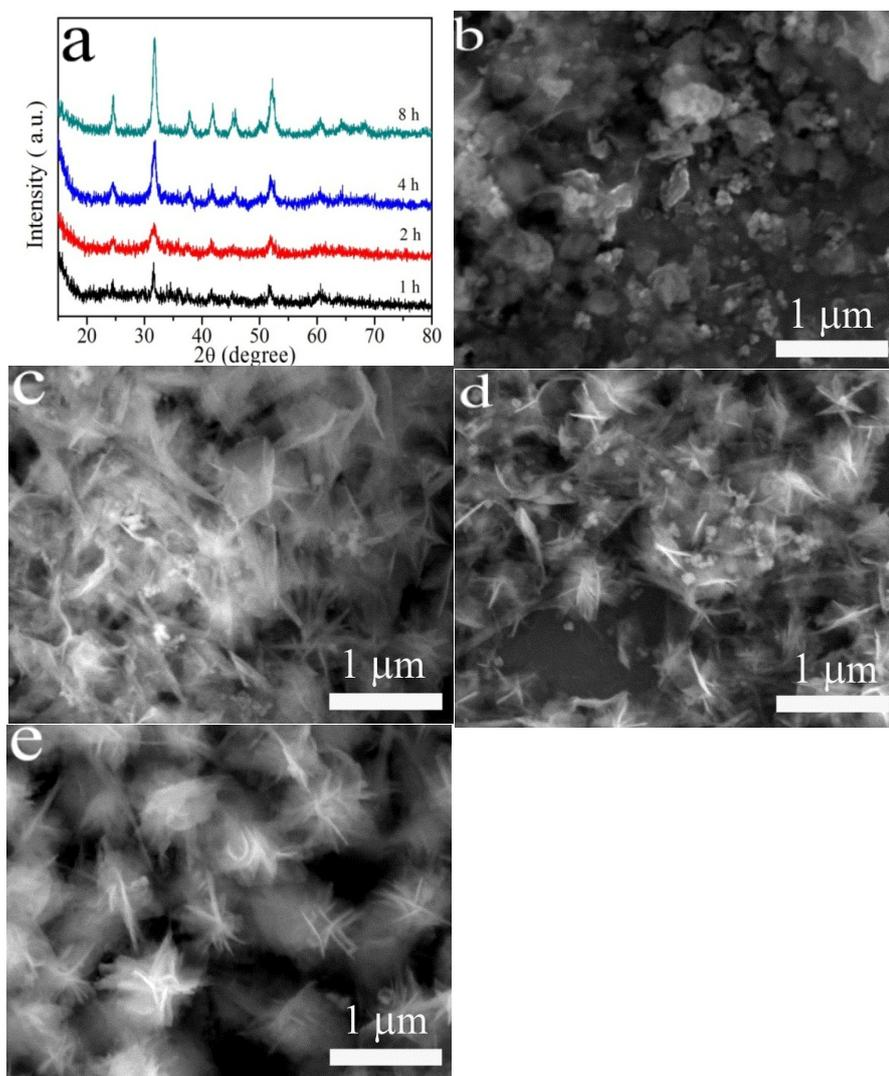
**Fig. S5** (a) XRD patterns of the XRD pattern of the samples obtained after different reaction durations; SEM images of the samples prepared at 180 °C for 1 h (a), 2 h (b); 4.0 h (c), 8 h (d).
