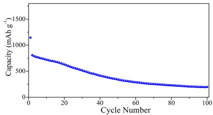
**Fig S12.** Cycling performance of pristine NiMn<sub>2</sub>O<sub>4</sub> nanoparticles at a current density of 1000 mA g<sup>-1</sup>. The pristine NiMn<sub>2</sub>O<sub>4</sub> electrode shows continuously decreasing capacities. The capacity decreases to ~200 mAh g<sup>-1</sup> after 100 cycles.
