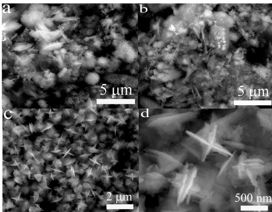
**Fig. S2** SEM images of the carbonate precursor obtained (a, b) in TEG and (c, d) in a solvent of TEG and water with a ratio of 1:1.
