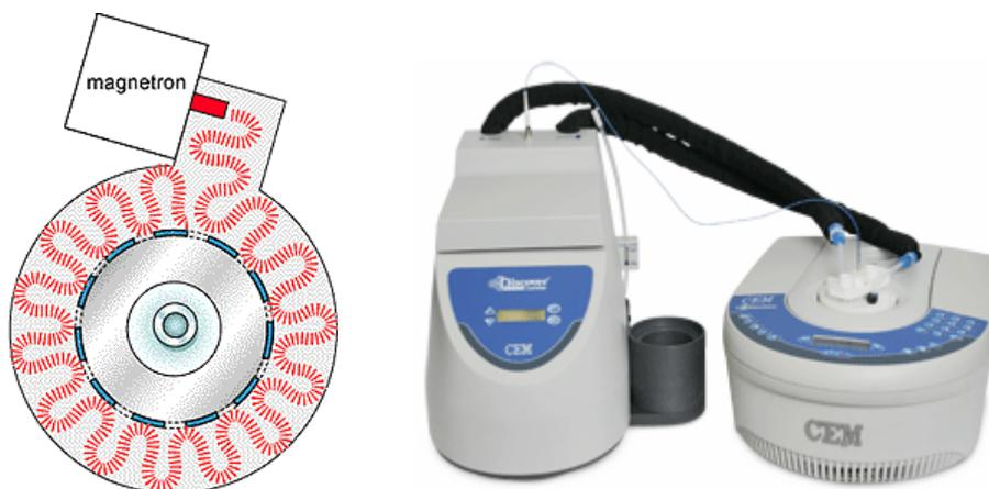
**Figure S1.** Left: CEM Discover single-mode microwave cavity. The sample is located in the center of the cavity and focused microwaves are generated and used to irradiate the sample. Right: CEM Discover equipped with a Coolmate. Images obtained from [www.cem.com](http://www.cem.com).
