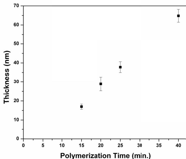
**Figure SI.4:** Isocyanate functionalized polymer brush thickness as a function of polymerization time.
