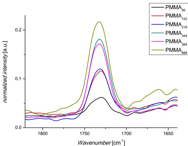
**Fig. S3:** The average spectra of the FT-IR micrographs showing an increase of the carbonyl stretching vibration with increasing degree of polymerization. The spectra were obtained by averaging 13×13 spectra in a square of ~10.5 μm<sup>2</sup> on the cellulose surface.
