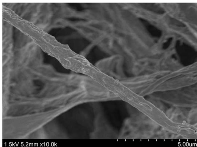
**Fig. S2:** The FE-SEM micrograph of the PMMA<sub>384</sub>-grafted cellulose fiber.
