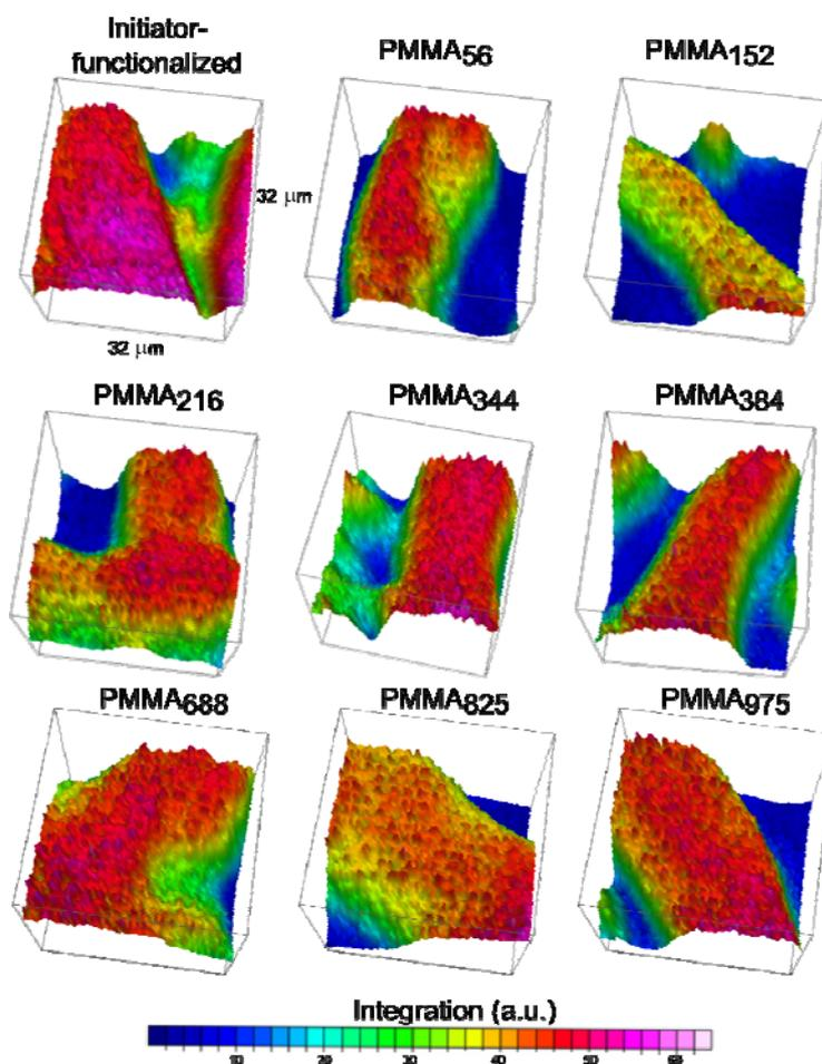
**Fig. S1.** False color high resolution FT-IR micrographs (4 cm<sup>-1</sup> spectral resolution with a 0.25 μm<sup>2</sup> spatial pixel resolution and an optical resolution of close to 1 μm) displaying the cellulose fibers located via their IR signal by integration of the region 950-1250 cm<sup>-1</sup>.
