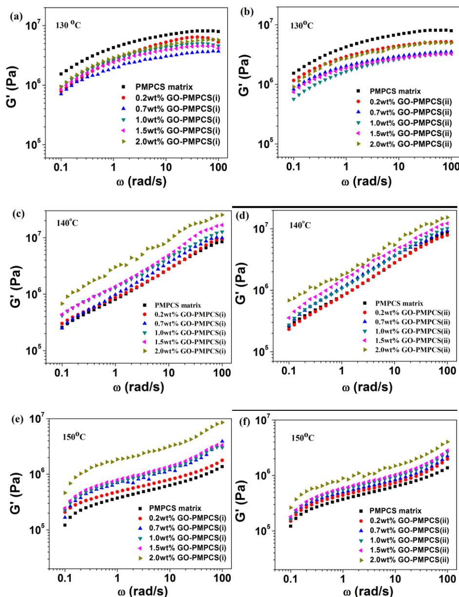
Figure S2. Frequency dependence of storage modulus of the matrixes with different GO-PMPCS composites contents : (a), (b) at 130 °C; (c),(d) at 140 °C, (e),(f) at 150 °C.
