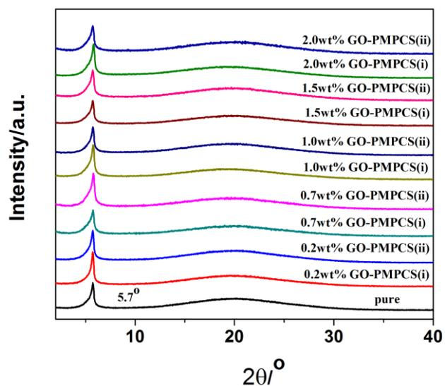
**Fig.S3.** Wide-angle X-ray diffraction spectra of PMPCS matrix with different GO-PMPCS composites contents.
