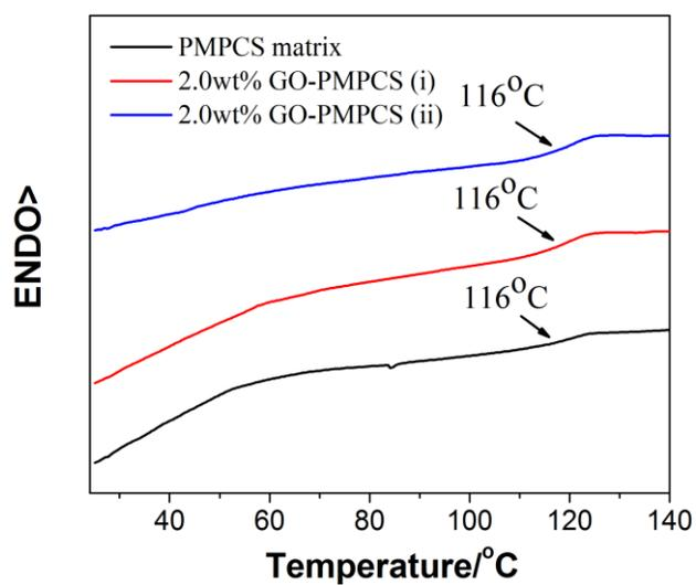
**Fig.S4.** DSC curves of PMPCS matrix, PMPCS matrix with 2.0 wt% GO-PMPCS (i) and 2.0 wt% GO-PMPCS (ii). The heating rate was 20 °C min<sup>-1</sup>.
