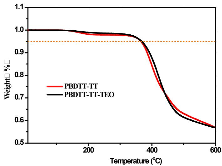
**Figure S4.** TGA thermograms of the polymers with a heating rate of 10 °C /min under nitrogen.
