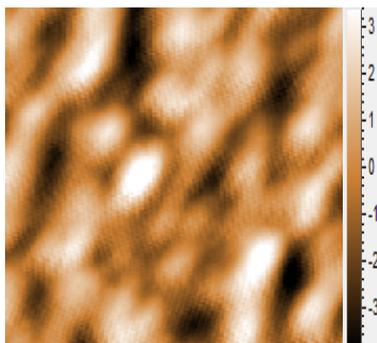
**Figure S7.** AFM topography mages ( $1\mu\text{m} \times 1\mu\text{m}$ ) of PBDTT-TT-TEO:PCB-TEO (1:2 w/w).
