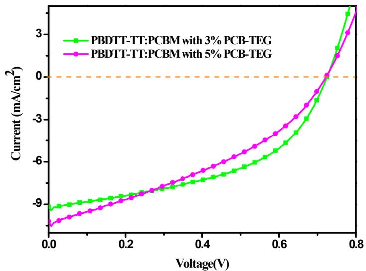
**Figure S8.** J-V curves of PBDTT-TT:PCBM with 3% PCB-TEO and PBDTT-TT:PCBM with 5% PCB-TEO.
