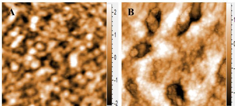
**Figure S9.** AFM topography mages ( $1\mu\text{m} \times 1\mu\text{m}$ ) of (A) PBDTT-TT:PCBM, (B) PBDTT-TT:PCBM with 3% PCB-TEO.
