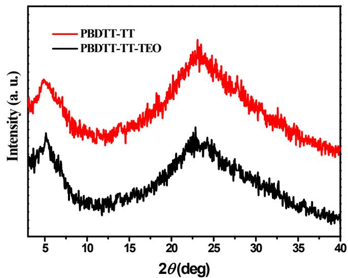
**Figure S6.** X-ray diffraction patterns of the polymers PBDTT-TT and PBDTT-TT-TEO.
