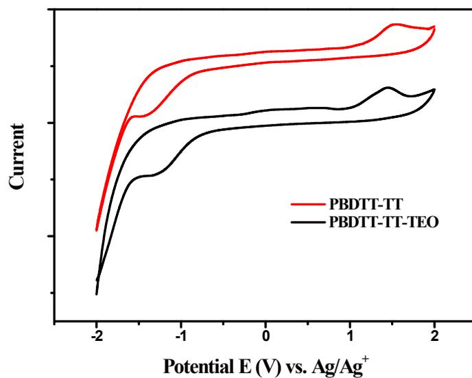
**Figure S5.** Cyclic voltammograms of PBDTT-TT and PBDTT-TT-TEO drop-cast on a Pt electrode in 0.1 mol/L  $\text{Bu}_4\text{NPF}_6$ -acetonitrile solutions at a scan rate of 50 mV/s.
