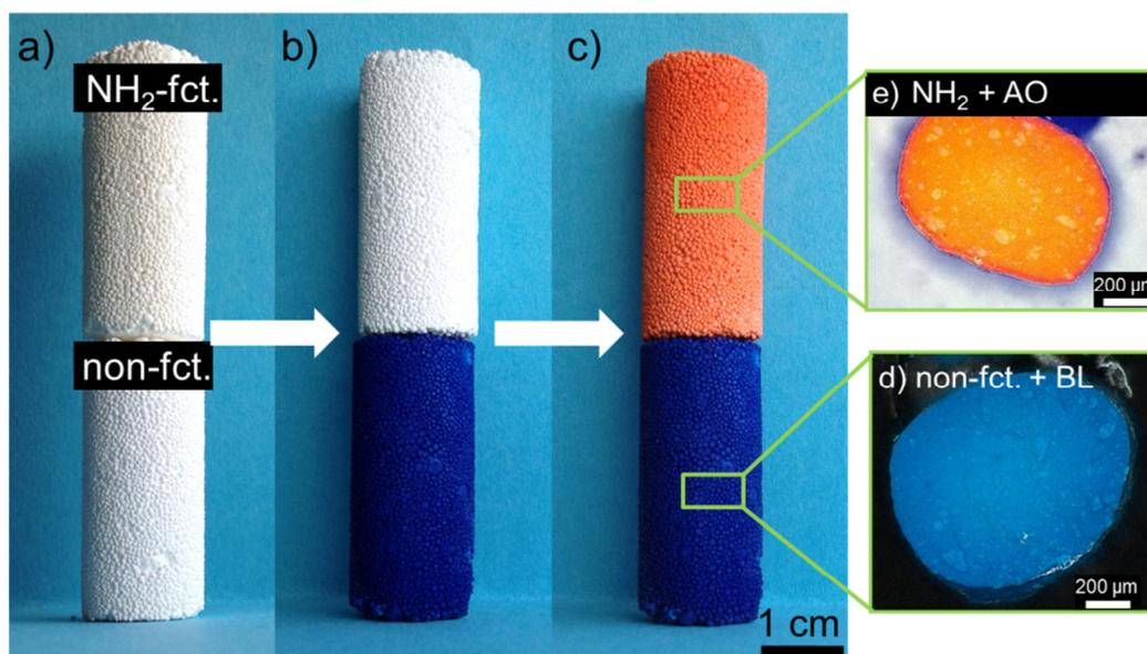
**Figure S.3:** Selective adsorption of model dye molecules on MAdS: a) amino-functionalized and non-functionalized MAdS before adsorption; b) after adsorption of methylene blue (BL); c) after adsorption of acid orange (AO); d and e) microscopic cross-sections of single beads after dye adsorption.
