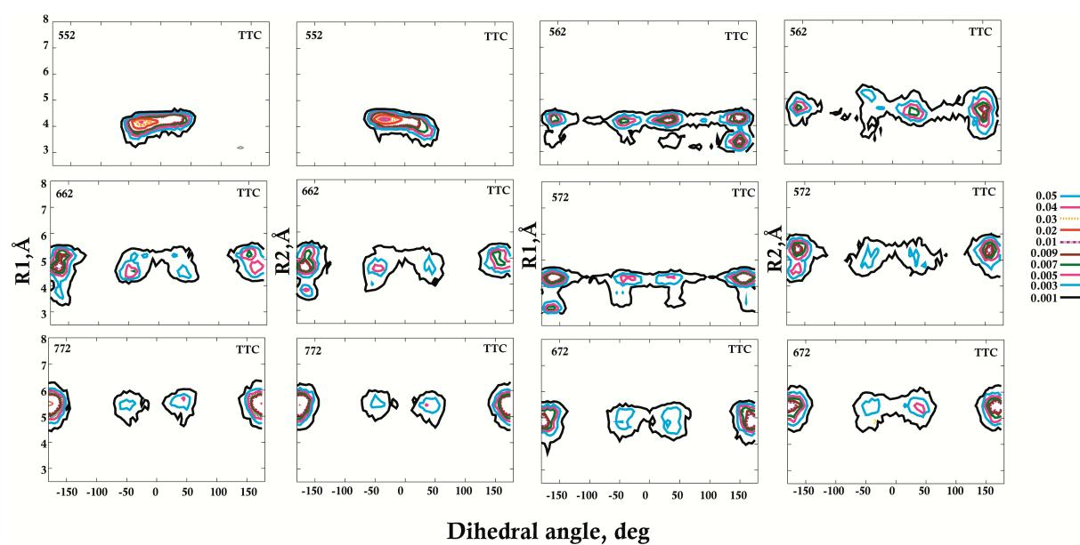
(c) Probability contours corresponding to the diene dihedral angle,  $\varphi_4$  and distances R1 & R2 between reactive sites for the TCT triene of all the ring systems:
