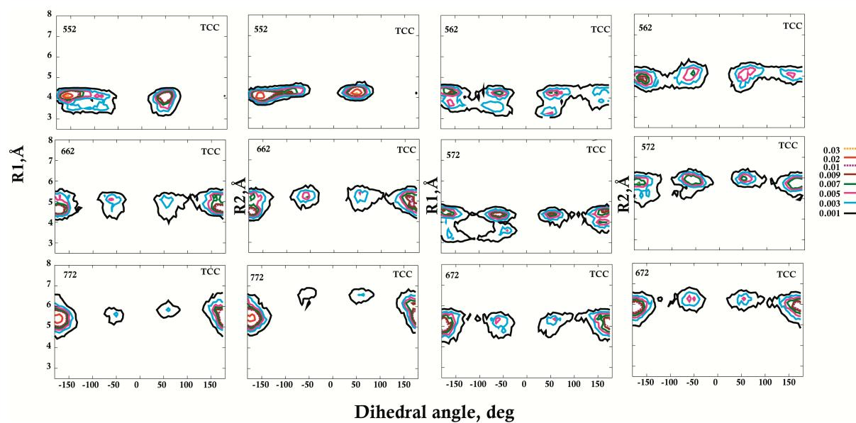
(g) Probability contours corresponding to the diene dihedral angle,  $\varphi_4$  and distances R1 & R2 between reactive sites for the CCT triene of all the ring systems:
