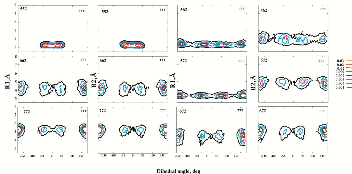
(b) Probability contours corresponding to the diene dihedral angle,  $\varphi_4$  and distances R1 & R2 between reactive sites for the TTC triene of all the ring systems:
