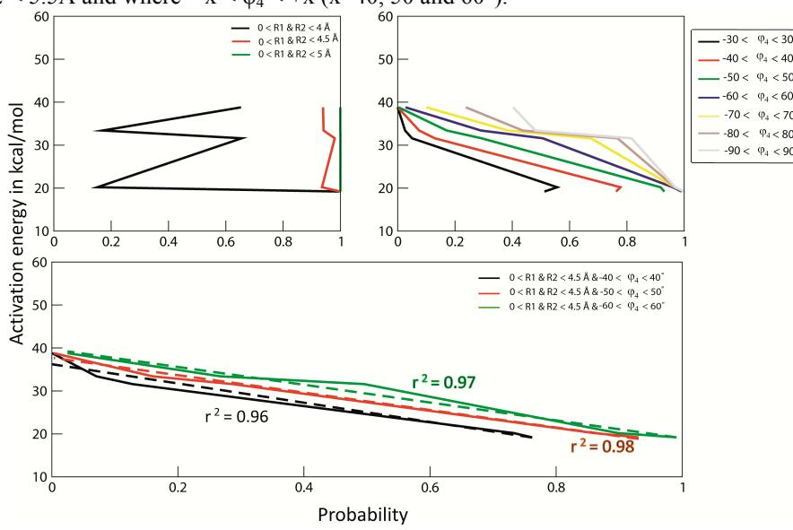
(b) Transition state energy barrier for 662 ring system versus (a) probability of finding the system where the distances R1 and R2 are <4 Å, < 4.5 Å, < 5 Å, < 5.5 Å, ; (b) Probability of finding the system where the diene dihedral angles satisfies  $-x < \varphi_4 < +x$  ( $x=30, 40, 50, 60, 70, 80, 90^\circ$ ); (c) probability of finding the system where R1 & R2 < 5.5 Å and where  $-x < \varphi_4 < +x$  ( $x=50, 60$  and  $70^\circ$ ).
