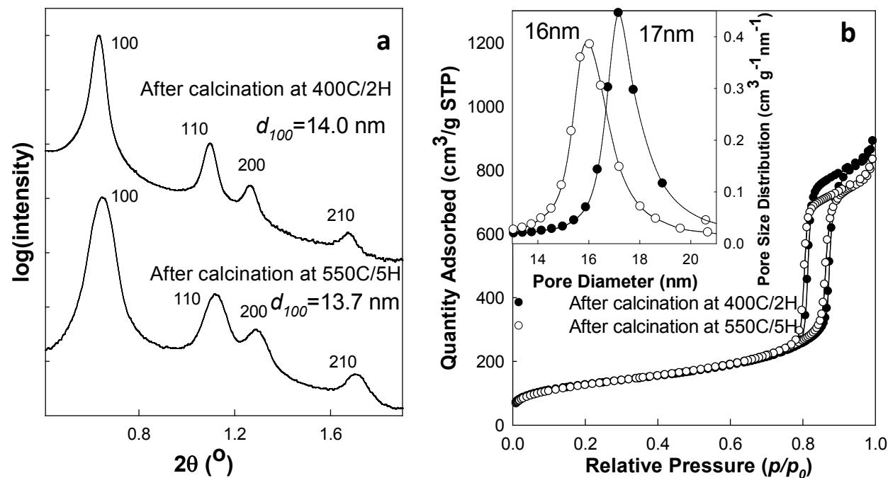
**Supporting Figure S5.** (a) SAXS patterns and (b) nitrogen adsorption isotherm (and inset with pore size distributions) of LP-SBA-15 silica after a shortened and standard calcination. LP-SBA-15 samples were synthesized with the condition of 17C/1H+130C/3H, 1 g TIPB per 2.4 g Pluronic P123. SAXS patterns were offset vertically to facilitate comparison. Figures taken from L. Cao, Ph.D. Dissertation, Graduate Center, City University of New York, 2010
