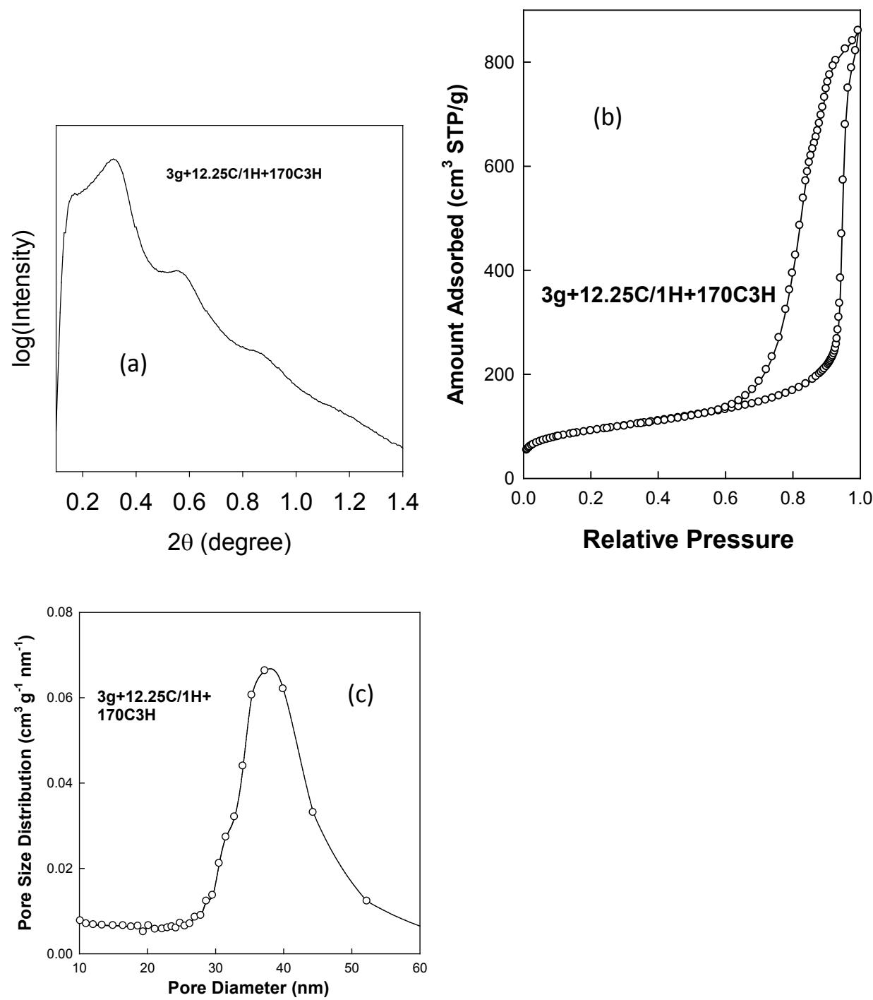
**Supporting Figure S4.** (a) SAXS pattern, (b) nitrogen adsorption isotherm and (c) pore size distribution of a calcined SBA-15 sample prepared at an initial synthesis temperature of 12.25 °C and hydrothermally treated at 170 °C for 3 hours.
