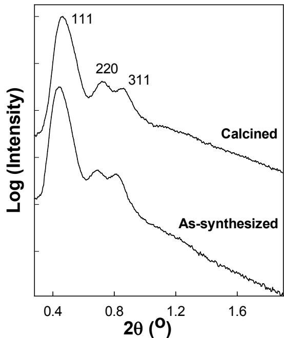
**Supporting Figure S7.** SAXS patterns of as-synthesized and calcined LP-FDU-12 prepared via a short synthesis. Figure taken from L. Cao, Ph.D. Dissertation, Graduate Center, City University of New York, 2010
