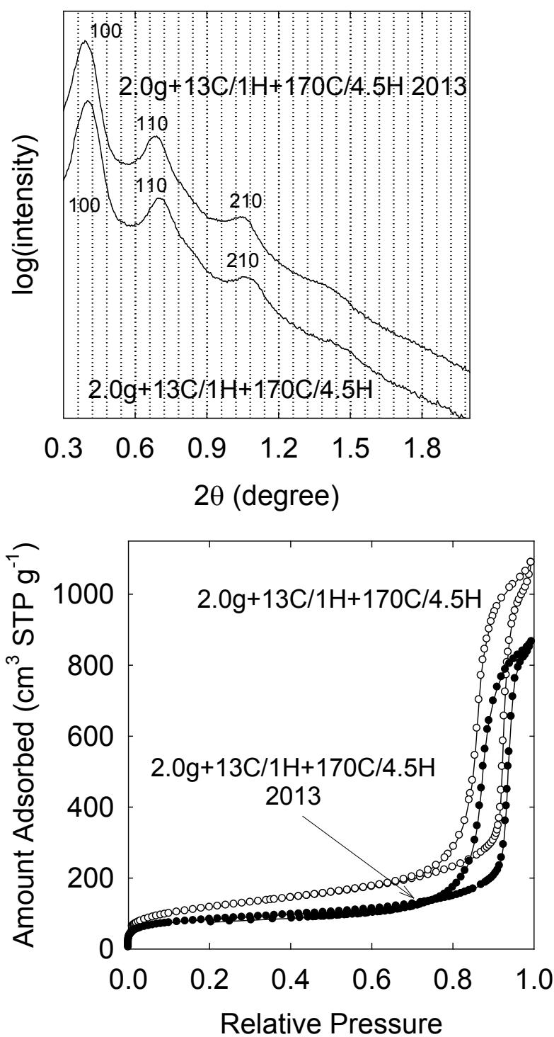
**Supporting Figure S9.** (top) SAXS patterns of calcined sample prepared at an initial temperature of 13 °C with subsequent hydrothermal treatment at 170 °C for 4.5 h. One pattern was shown in Figure 1. The pattern denoted “2013” was acquired after storage in the calcined form for 4 years. Grid lines are included to allow for an easier comparison of the peak positions. (bottom) Nitrogen adsorption isotherms for this sample, collected initially and after 4 years of storage.
