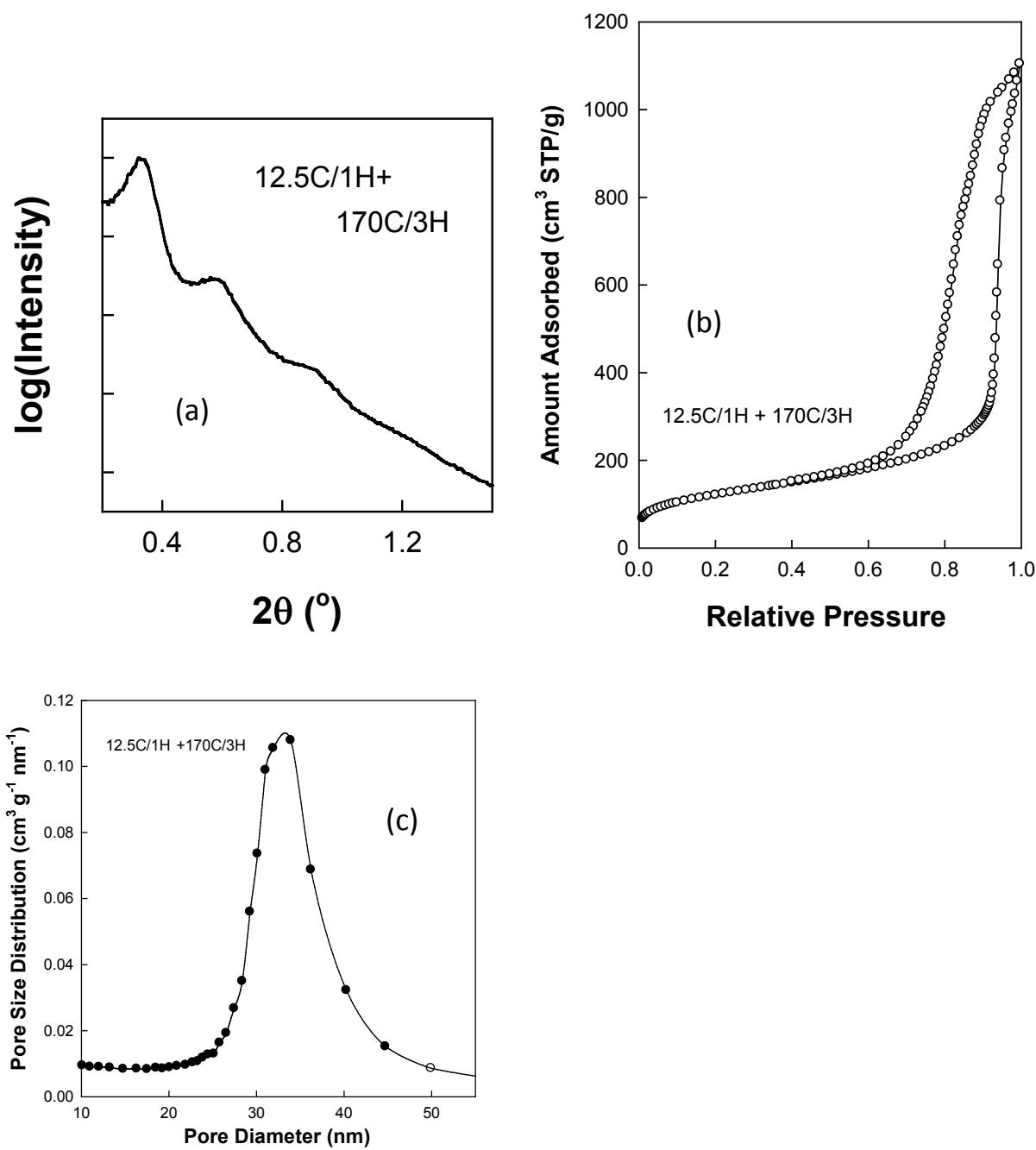
**Supporting Figure S3.** (a) SAXS pattern, (b) nitrogen adsorption isotherm and (c) pore size distribution of a calcined SBA-15 sample prepared at an initial synthesis temperature of  $12.5^{\circ}\text{C}$  and hydrothermally treated at  $170^{\circ}\text{C}$  for 3 hours.
