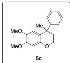
**6,7-dimethoxy-4-methyl-4-phenylchromane (5c):** General procedure-4 was carried out with alcohol **4c** (109 mg, 0.30 mmol), CuI (12 mg, 20 mol %), 2,2'-bipyridine (10 mg, 20 mol %), KO'Bu (101 mg, 0.90 mmol), and DMF (3 mL) at 120 °C for 24 h. Purification of the crude material by silica gel column chromatography (petroleum ether/ethyl acetate, 90:10) furnished
