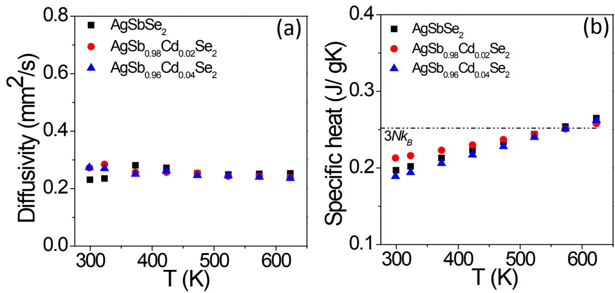
**Fig. S2** Temperature dependent (a) thermal diffusivity and (b) specific heat of AgSb<sub>1-x</sub>Cd<sub>x</sub>Se<sub>2</sub> (x= 0-4 mol%) samples with Dulong–Petit specific heat at constant volume.
