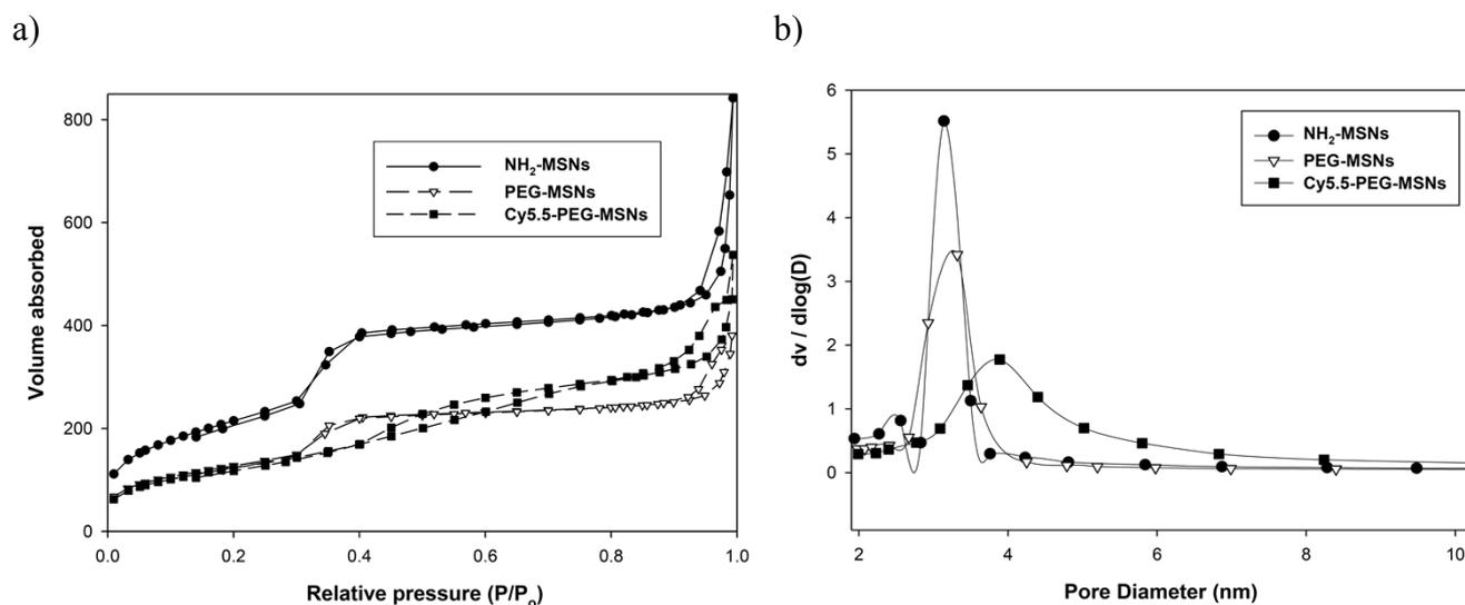
**Figure S4.** a) Nitrogen adsorption/desorption isotherms of NH<sub>2</sub>-MSNs, PEG-MSNs, Cy5.5-PEG-MSNs. b) BJH narrow pore size distributions (based on adsorption branch).
