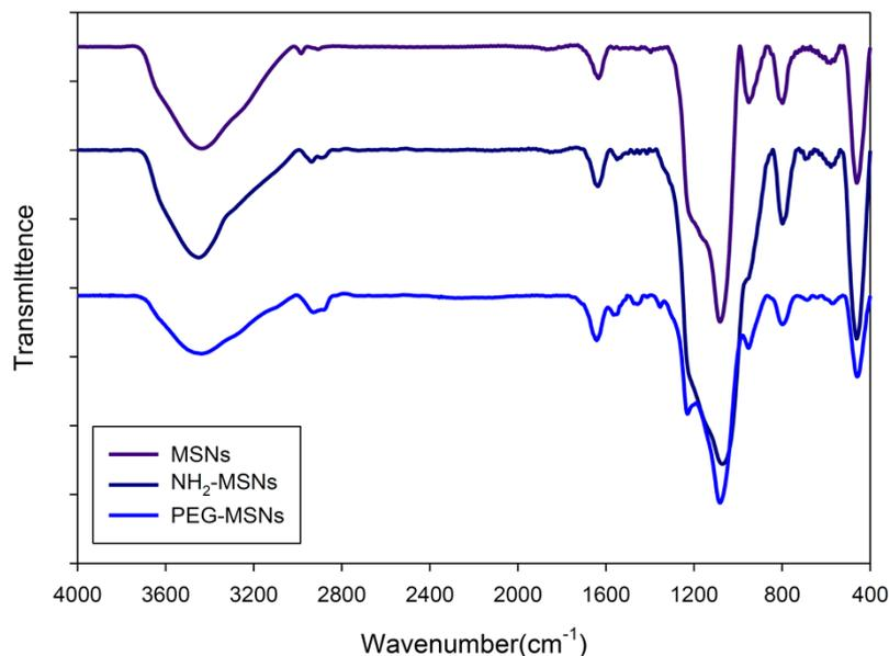
**Figure S1.** FT-IR spectra. MSNs, NH<sub>2</sub>-MSNs and PEG-MSNs.
