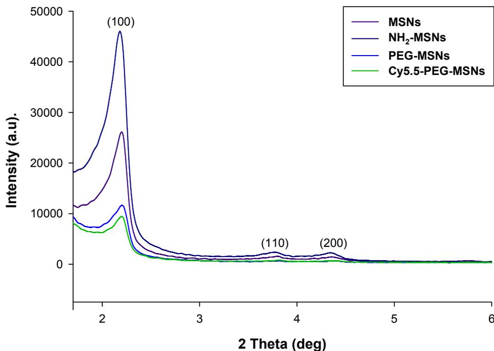
**Figure S3.** Low-angle XRD (1-6°) XRD patterns of the MSNs. Typical of hexagonal mesoporous silica nanoparticles are shown (100, 110, 200) in MSNs, NH<sub>2</sub>-MSNs, PEG-MSNs and Cy5.5-PEG-MSNs.
