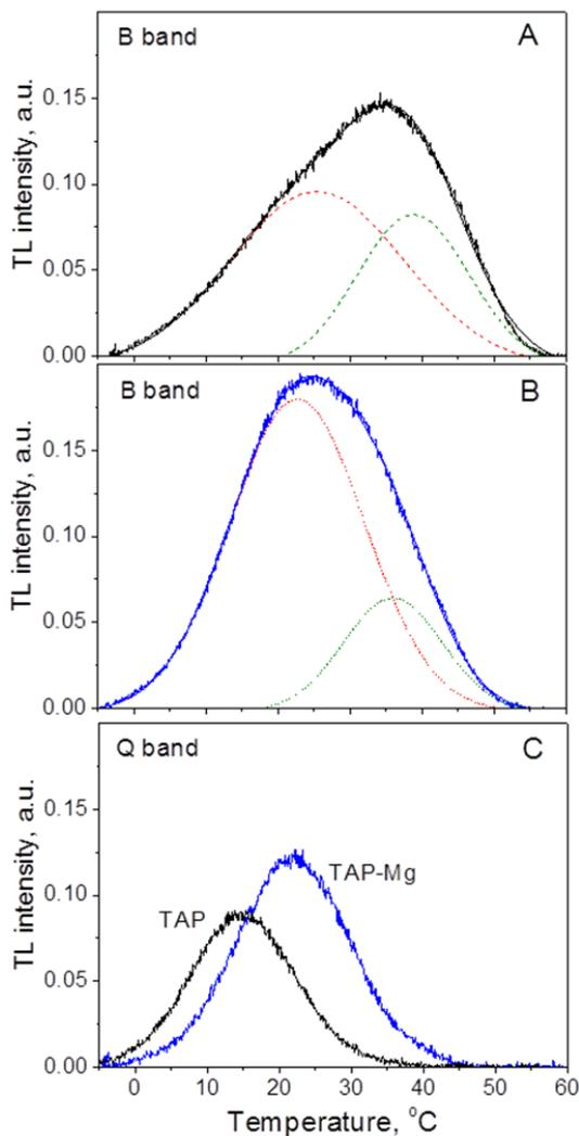
**Figure 2.** Effect of Mg-deprivation on thermoluminescence glow curves measured from *C. reinhardtii* cells. (A) Thermoluminescence curves measured from the control cells (TAP) and (B) after seven days of Mg-starvation (TAP-Mg) at pH 7.0 in the absence (A, B) and the presence of 20  $\mu$ M DCMU (C). The dashed lines represent deconvolution of the Gaussian sub-components.
