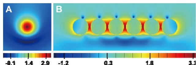
**Figure S3.** Electric field intensity enhancement contours at a logarithmic scale for a single-line Au nanoparticle array. The nanoparticle array consists of six nanoparticles which are linearly aligned in a row with a gap distance of 8 nm. The diameter of the nanoparticles is 66 nm. Projections are shown in the yz plane (A) and xz plane (B) of the Au nanoparticles array. The mesh size is 1 nm.
