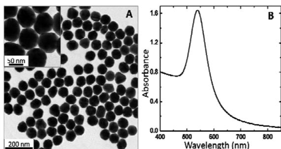
**Figure S2.** TEM micrograph (A) and UV-vis-NIR spectrum of the employed 66 nm gold nanoparticle colloid.
