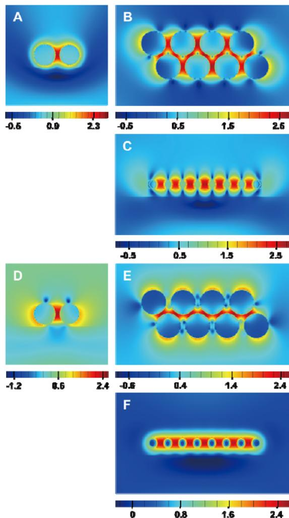
**Figure S4.** Electric field intensity enhancement contours at a logarithmic scale for a double-line Au nanoparticle array. The array consists of eight nanoparticles linearly aligned in two alternate rows with a closest gap distance of 8 nm. (A-C) yz, xy, and xz projections of E-field enhancement maps for the double-line array, with excitation polarization in the x direction. (D-F) yz, xy, and xz projections of E-field enhancement maps for excitation polarization in the y direction.
