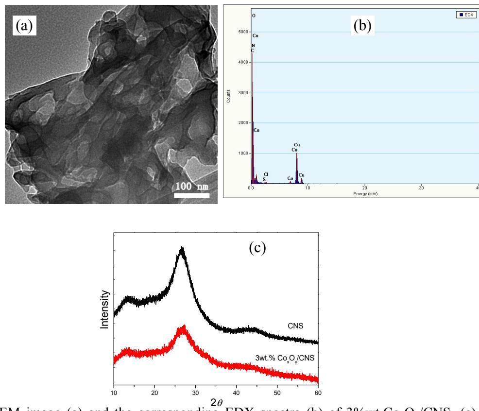
**Figure S4.** TEM image (a) and the corresponding EDX spectra (b) of 3%wt. $\text{Co}_x\text{O}_y$ /CNS. (c) Powder X-ray diffraction pattern of CNS and 3%wt.  $\text{Co}_x\text{O}_y$ /CNS. No solid-state cobalt species can be found with TEM and XRD investigations, but the result of EDX analysis confirmed the presence of cobalt in CNS matrix, which was further realized as Co(III) and Co(II) species by XPS analysis (Figure S3).
