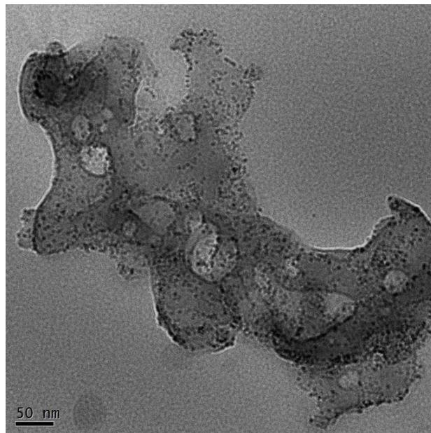
**Figure S9.** Typical TEM image of 3%wt.Co<sub>3</sub>O<sub>4</sub>/CNS. Co<sub>3</sub>O<sub>4</sub> nanoparticles were found to be well dispersed on the CNS matrix.
