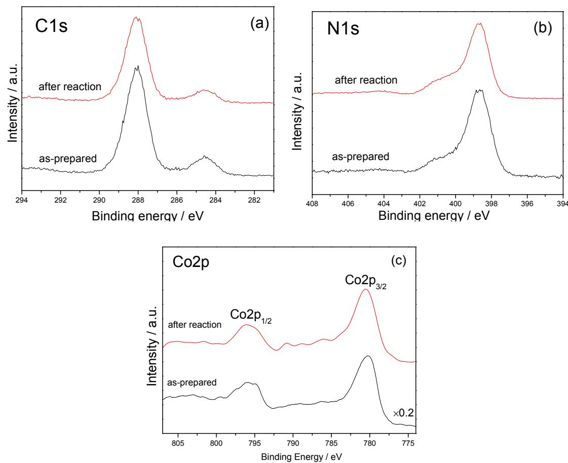
**Figure S12.** XPS analysis of 3%wt. $\text{Co}_3\text{O}_4$ /CNS before and after the photocatalytic water oxidation reaction. No significant alternations can be found from the C1s (a), N1s (b) and Co2p (c) spectra before and after the reaction.
