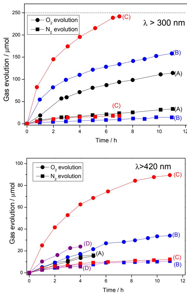
**Figure S6.** Photocatalytic water oxidation by CNS (A), 3%wt.  $\text{Co}_x\text{O}_y/\text{CNS}$  (B), 3%wt.  $\text{Co}_3\text{O}_4/\text{CNS}$  (C) and physical mixture of 3%wt.  $\text{Co}_3\text{O}_4$  and CNS (D), as a function of time under UV and visible light illumination.
