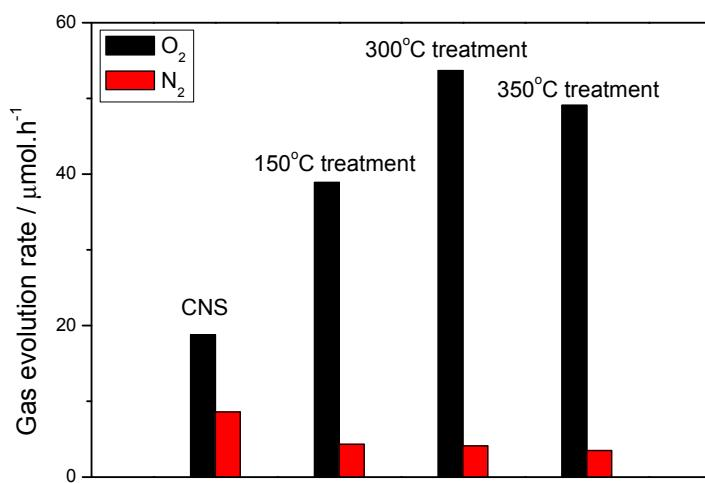
**Figure S2.** The relationship between the temperature of heat treatment and the photocatalytic activities of 3wt.%  $\text{Co}_x\text{O}_y/\text{CNS}$  sample.
