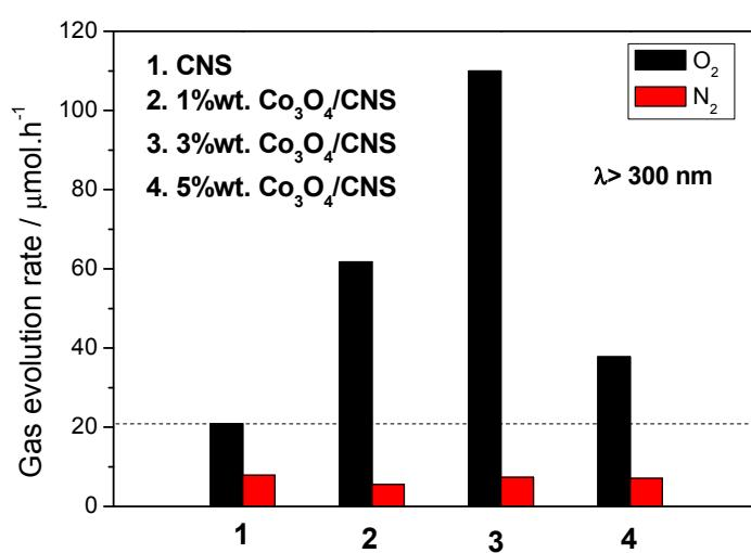
**Figure S7.** Influence of loading amount of Co<sub>3</sub>O<sub>4</sub> on photocatalytic water oxidation.
