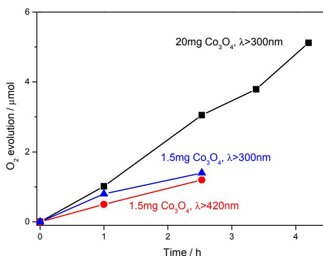
**Figure S8.** Photocatalytic water oxidation by Co<sub>3</sub>O<sub>4</sub> nanoparticles (~3nm).
