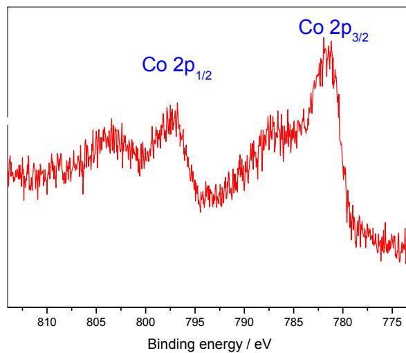
**Figure S3.** XPS spectrum of Co lines obtained from 3%wt. $\text{Co}_x\text{O}_y/\text{CNS}$  sample.
