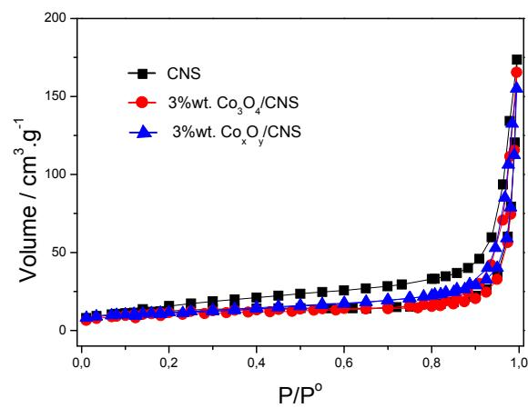
**Figure S5.** Nitrogen adsorption-desorption isotherms of CNS, 3%wt.  $\text{Co}_3\text{O}_4$ /CNS and 3%wt.  $\text{Co}_x\text{O}_y$ /CNS.
